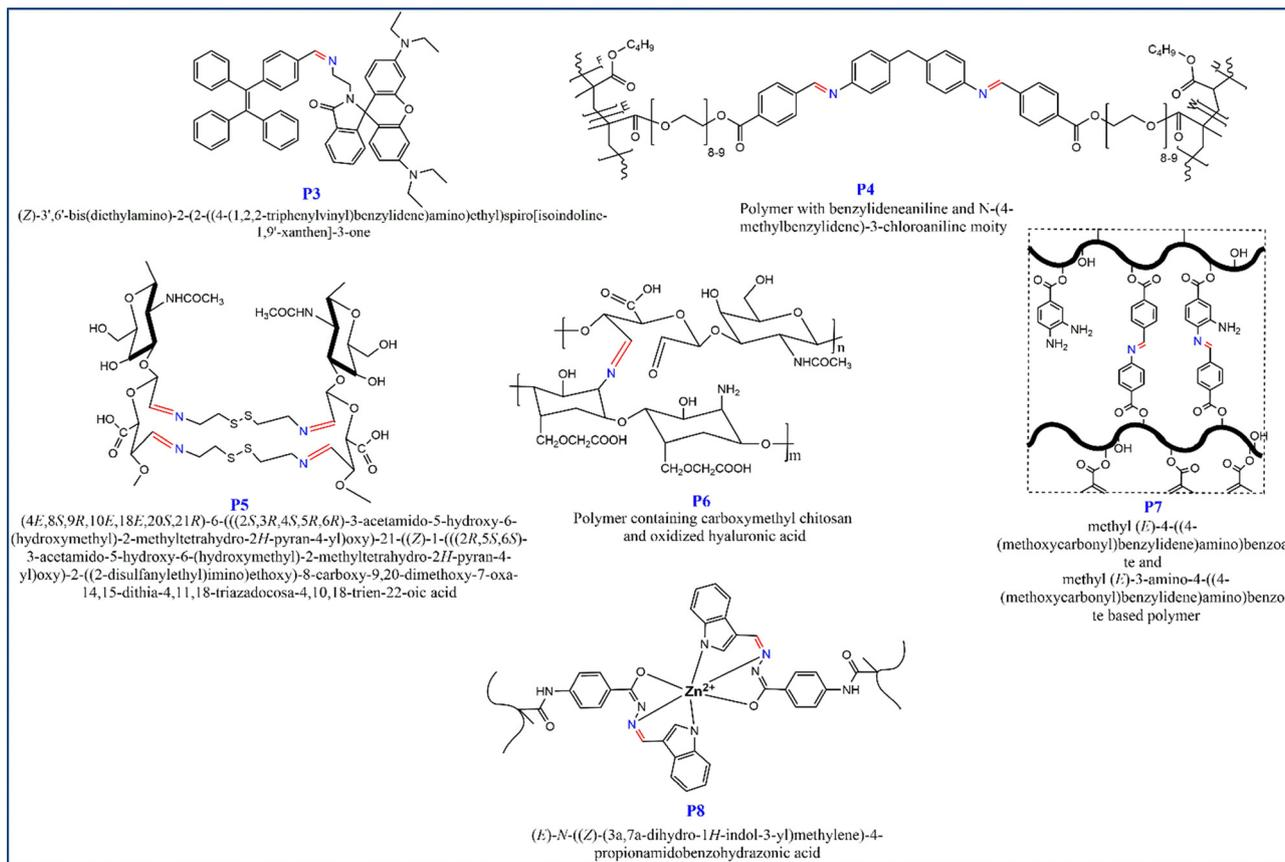
Scheme 4 Schiff base-based systems exhibiting self-healing capacity.
