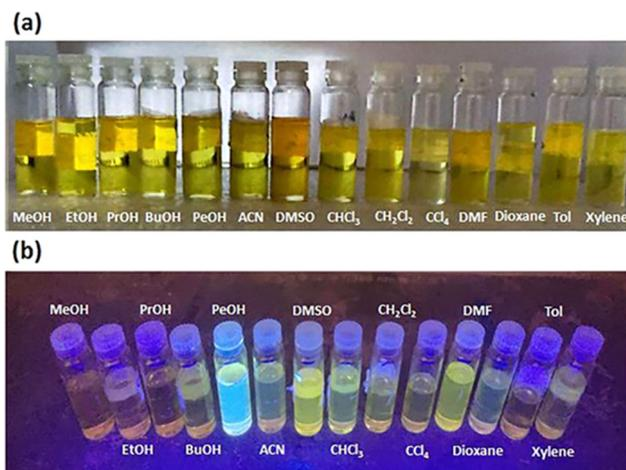
**Fig. 13** Fluorescence images of Schiff base ( $L^{30}$ ) in different solvents: (a) Normal light (no emission), (b) upon UV radiation (emission wavelength,  $\lambda_{ex} = 366$  nm) at room temperature; reproduced from ref. 123 with permission from Elsevier, Copyright 2024.
