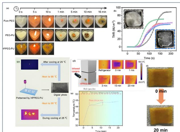
**Fig. 29** (a) Fire-resistance performance by candle test of pure PEG, PEG4000-PU, and **P1**-4000; (b) total heat release rate curve; (c) imaging of thermosensitivity of **P1**-6000 in nonwoven fabric during heating or cooling; (d) infrared images (e), time-temperature curves, and shape stability (f) of **P1**-6000 on the refrigerator; reproduced from ref. 52 with permission from Elsevier, Copyright 2022.
