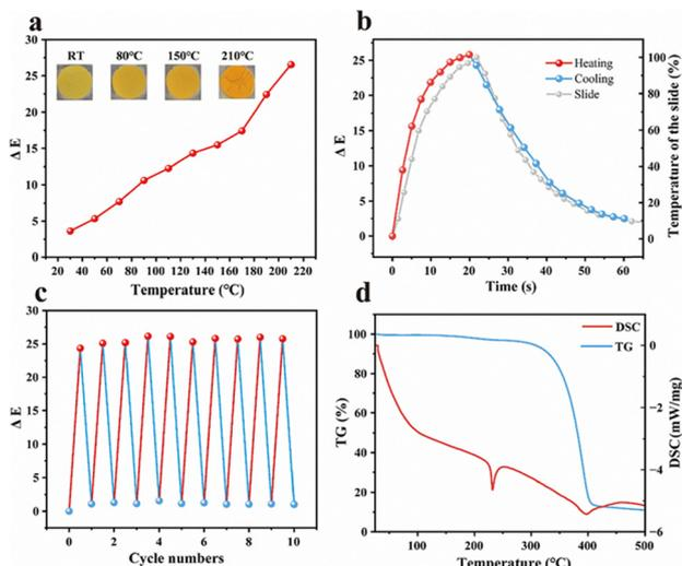
**Fig. 9**  $\text{H}_2\text{L}^{21}$  showing thermochromic responsiveness (a)  $\Delta E$ - $T$  plot, (b) response time curve and temperature of the slide, (c) heating-cooling cycles, and (d) TG-DSC curve; reproduced from ref. 80 with permission from Elsevier, Copyright 2024.
