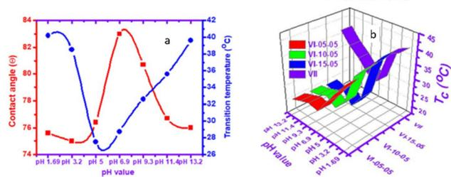
Fig. 19 The change in transition temperature ( $T_{cs}$ ) and contact angles ( $\theta$ )<sup>o</sup> via the pH contact angles ( $\theta$ )<sup>o</sup> against pH changes; reproduced from ref. 129 with permission from Springer, Copyright 2023.
