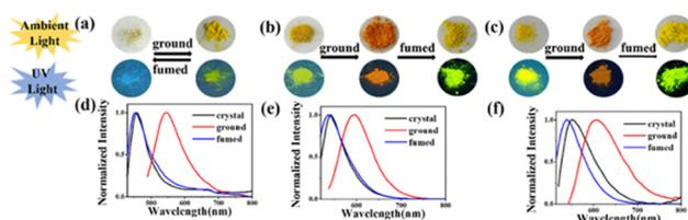
**Fig. 14** Images and fluorescence spectra of  $HL^1$  (a) and (d), 1-Zn-complex of  $HL^1$  (b) and (e), and 1-THF (c) and (f) under ambient light and UV irradiation at 365 nm under different conditions; reproduced from ref. 61 with permission from ACS, Copyright 2022.
