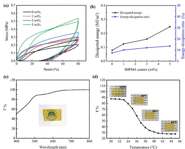
Fig. 18 (a) **P18** showing a continuous loading–unloading cycle, (b) changes in dissipation energy, (c) transmittance plots and optical photographs of **P18** hydrogel at room temperature, and (d) temperature–transmittance change curves; reproduced from ref. 36 with permission from Wiley, Copyright 2023.
