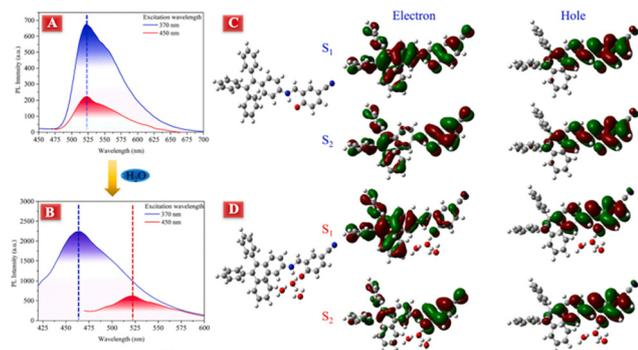
Fig. 27 PL spectra of the  $L^{26}$  compound in THF (A) and 10% water fraction with THF after 12 h standing (B). (C) and (D) Optimized keto structure of  $L^{26}$  and pertinent calculated orbitals of the solvated keto structure for the  $S_1$  and  $S_2$  state; reproduced from ref. 121 with permission from Elsevier, Copyright 2021.
