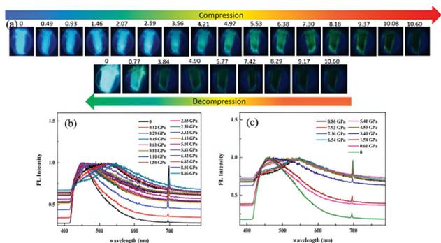
Fig. 11 (a) Fluorescence images and (b) and (c) spectra captured *in situ* at 365 nm (excitation) of a single crystal of **P3** during compression and decompression; reproduced from ref. 65 with permission from Elsevier, Copyright 2019.
