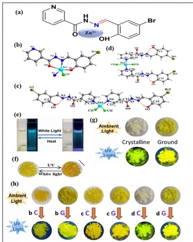
Fig. 16 (a) Chemical and (b), (c), (d) molecular structure of H<sub>2</sub>L<sup>11</sup> and complex synthesized using salicylaldehyde hydrazone ligand, respectively. (e) & (f) Photochromism shown by complex (b) & (c). (g) Mechanochromic luminescence property displayed by complex (d). (h) Photographs showing mechanochromic properties of complexes (b), (c) and (d) under ambient light and 365 nm UV light; reproduced from ref. 127 with permission from ACS, Copyright 2023.
