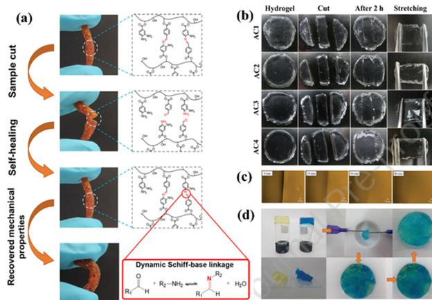
**Fig. 10** (a) Self-healing mechanism (24 hour) of PVA-CHO-NH<sub>2</sub> polymer (**P7**) *via* Schiff base reaction; reproduced from ref. 102 with permission from Elsevier, Copyright 2022; (b) self-healing ability **P5** hydrogel induced by cutting; (c) microlevel illustration of the hydrogel at different times after the hydrogel is cut; (d) optical evidence of the self-healing process; reproduced from ref. 103 with permission from Elsevier, copyright.
