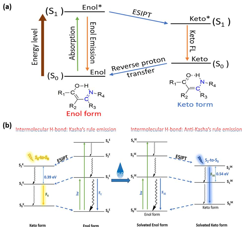
**Scheme 8** (a) Schematic representation of the four-level ESIPT process. (b) Possible mechanism for the dynamic stimuli-responsive fluorescence switch, following Kasha and Anti-Kasha's rule involving in intermolecular H-bond for solvated L26, respectively.<sup>121</sup>
