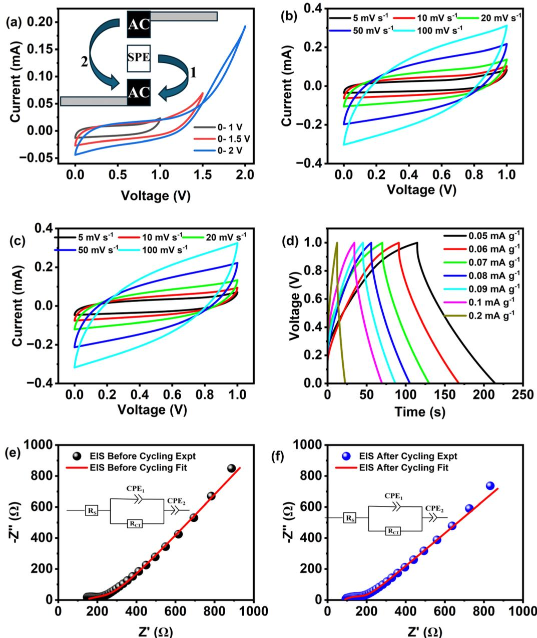
Fig. 14 (a) Cyclic voltammety of the EDLC device at different potential windows (inset: schematic diagram of the EDLC device). (b) Cyclic voltammety of the EDLC device at different scan rates. (c) CV after performing the cycling test for 5000 cycles. (d) GCD of the EDLC at different current densities. (e) Nyquist plot of the EDLC before cycling, and (f) Nyquist plot of the EDLC after cycling.
