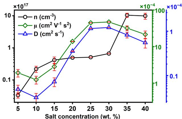
Fig. 5 Variation of transport properties such as  $n$ ,  $\mu$  and  $D$  as per the S-G model for PVA/CS-NaClO<sub>4</sub> SPEs.
