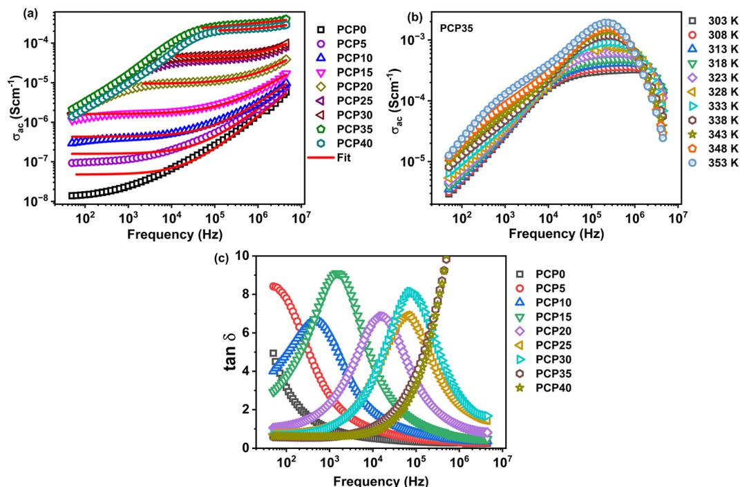
Fig. 6 (a) AC conductivity of the PVA/CS-NaClO<sub>4</sub> SPEs at room temperature (Jonscher's fit is given as a red solid line). (b) AC conductivity of the optimum conductivity sample for various elevated temperatures. (c) The tangent loss plot of PVA/CS-NaClO<sub>4</sub> SPEs at room temperature.
