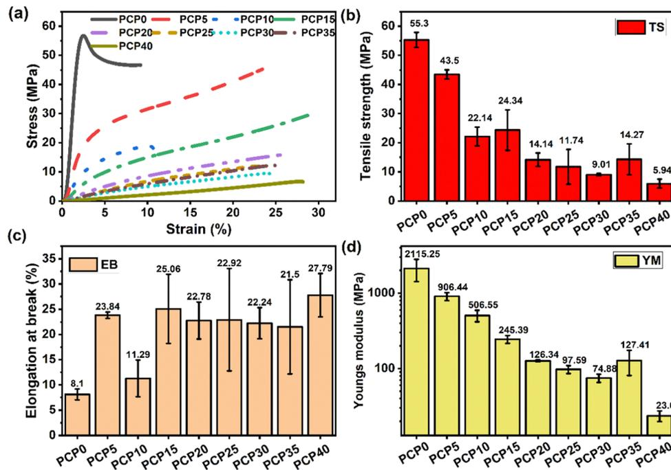
Fig. 13 (a) Stress–strain graph and (b)–(d) variation of the mechanical parameters for PVA/CS-NaClO<sub>4</sub> SPEs.
