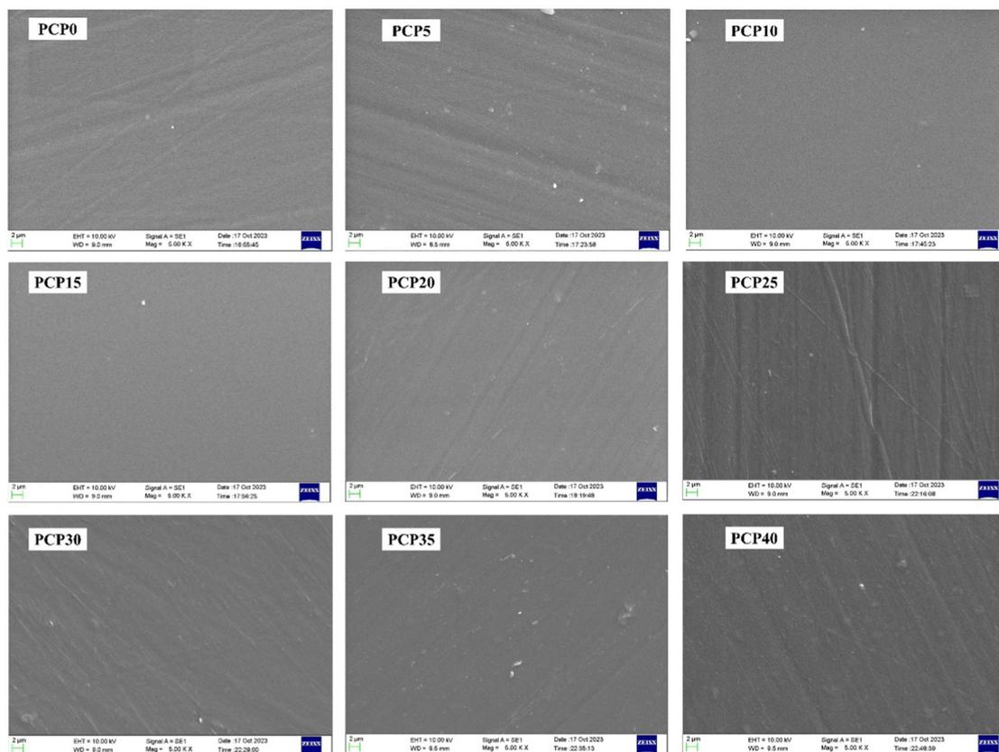
Fig. 8 SEM micrographs of PVA/CS-NaClO<sub>4</sub>·H<sub>2</sub>O SPEs.
