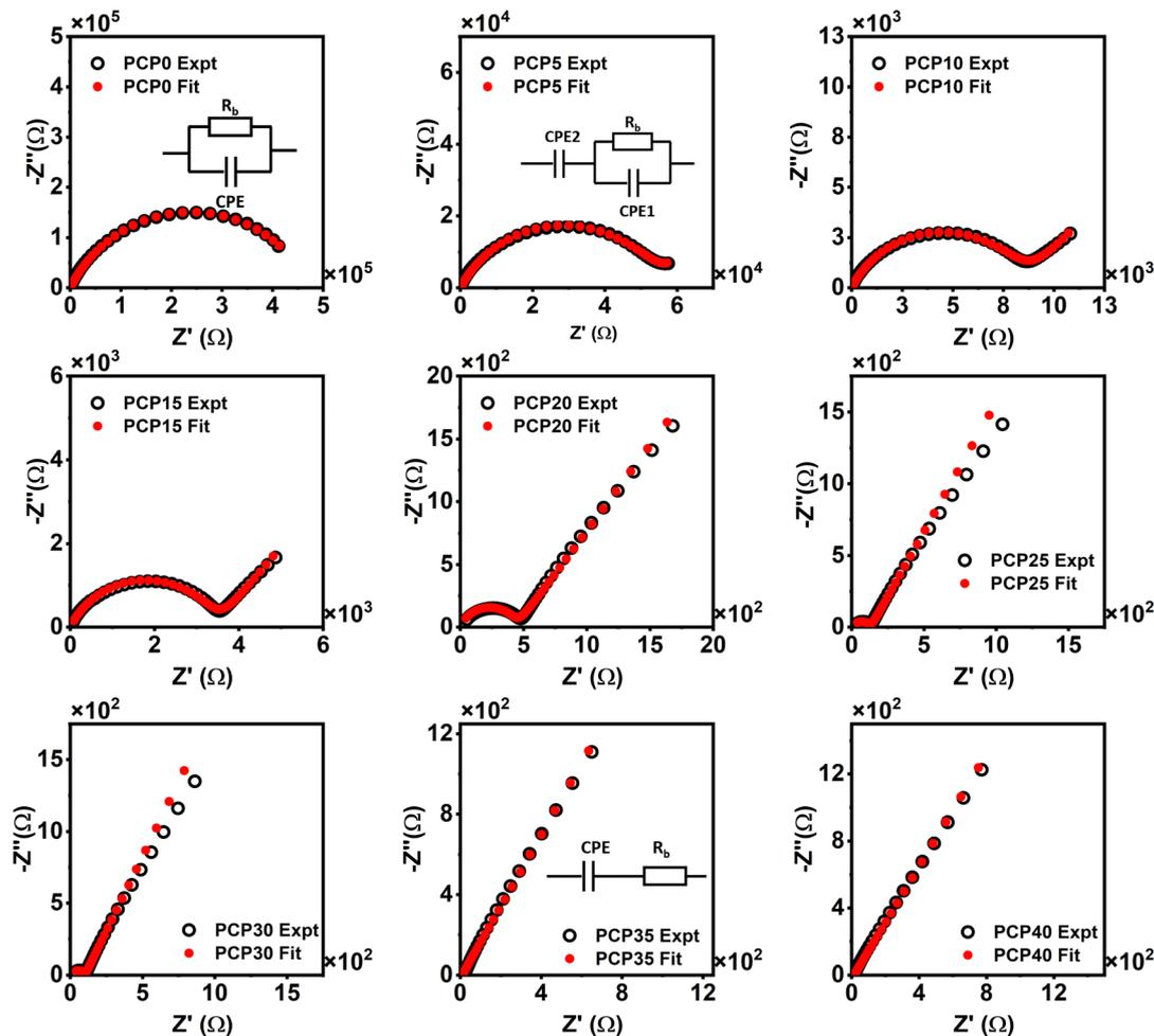
Fig. 4 Nyquist plot of PVA/CS-NaClO<sub>4</sub>-H<sub>2</sub>O SPEs (inset: equivalent circuit obtained through EEC analysis used to fit the Nyquist plot).
