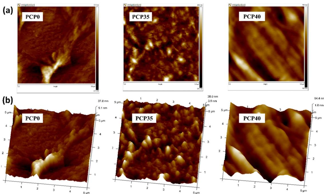
Fig. 9 (a) 2D and (b) 3D AFM images of selected PVA/CS-NaClO<sub>4</sub> SPEs.
