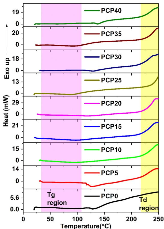
Fig. 10 DSC thermograms of PVA/CS-NaClO<sub>4</sub> SPEs.
