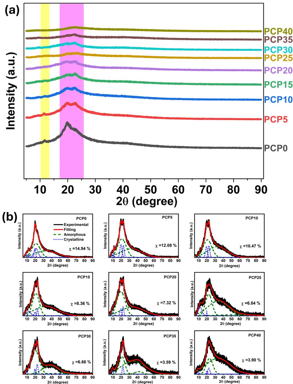
Fig. 3 (a) XRD spectra of PVA/CS-NaClO<sub>4</sub>·H<sub>2</sub>O SPEs and (b) deconvoluted XRD patterns of PVA/CS-NaClO<sub>4</sub>·H<sub>2</sub>O SPEs.
