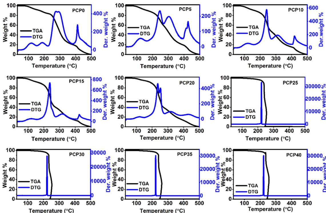
Fig. 11 TGA and DTG thermograms of SPEs.
