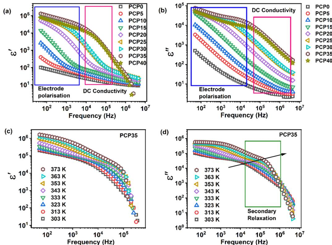
Fig. 7 Variation in (a)  $\epsilon'$  and (b)  $\epsilon''$  for PVA/CS- $\text{NaClO}_4$  SPEs and (c)  $\epsilon'$  and (d)  $\epsilon''$  at elevated temperature for the optimum conductivity sample PCP35.
