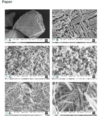
Fig. 2 FE-SEM micrographs of (A) Cu-BTC at 10kx, (B) Cu-BTC at 75kx, (C)  $CoMn_2O_4$  at  $40k\times$ , (D)  $CoMn_2O_4$  at  $180k\times$ , (E) K-OMS-2 at  $40k\times$ , and (F) K-OMS-2 at 180k×.
