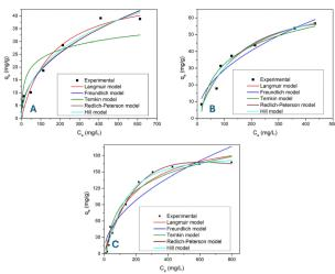
Fig. 7 Isotherm plots for the adsorption of asphaltenes onto (A) Cu-BTC (adsorbent dosage = 12.5 g L<sup>-1</sup>, t = 24 h, T = 30 °C, 150 rpm), (B) CoMn<sub>2</sub>O<sub>4</sub> (adsorbent dosage = 12.5 g L<sup>-1</sup>, t = 24 h, T = 30 °C, 150 rpm), and (C) K-OMS-2 (adsorbent dosage = 20 g L<sup>-1</sup>, t = 24 h, T = 30 °C, 150 rpm).
