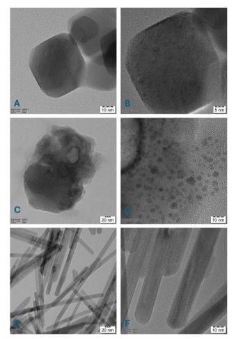
Fig. 3 HR-TEM images of (A) Cu-BTC at 300k×, (B) Cu-BTC at 500k×, (C)  $CoMn_2O_4$  at  $80k\times$ , (D)  $CoMn_2O_4$  at  $300k\times$ , (E) K-OMS-2 at  $80k\times$ , and (F) K-OMS-2 at 300k×
