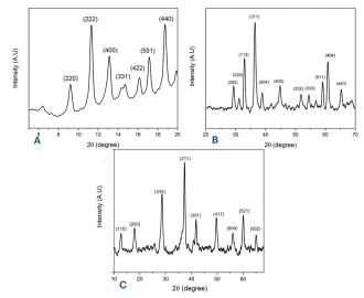
Fig. 6 XRD spectrum of (A) Cu-BTC, (B) CoMn<sub>2</sub>O<sub>4</sub>, and (C) K-OMS-2
