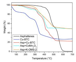
Fig. 8 Thermal degradation profile of Cu-BTC, asphaltenes, and asphaltenes subjected to oxidation under Cu-BTC, CoMn<sub>2</sub>O<sub>4</sub>, and K-OMS-2
