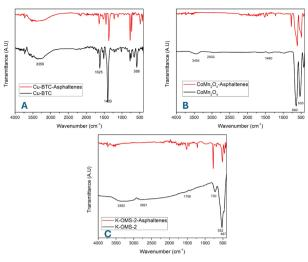
Fig. 5 FT-IR spectrum of (A) Cu-BTC, (B) CoMn<sub>2</sub>O<sub>4</sub>, and (C) K-OMS-2, before and after asphaltene adsorption
