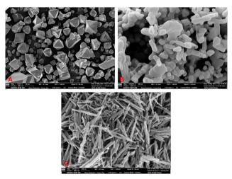
Fig. 4 FE-SEM micrographs of (A) Cu-BTC, (B) CoMn<sub>2</sub>O<sub>4</sub>, and (C) K-OMS-2 after asphaltene adsorption.
