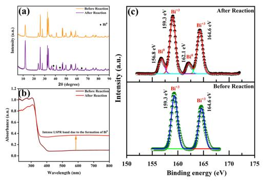
Fig. 12 (a) XRD, (b) DRS and (c) XPS patterns of AB10 before and after the reaction.
