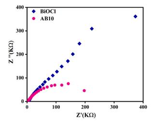
Fig. 7 EIS Nyquist plot of BiOCl and AB10
