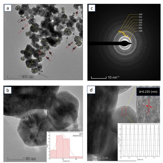
Fig. 6 HR-TEM images of AgZO NPs for analyzing (a) morphology and particle size, (b) particle size distribution histogram, (c) SAED pattern, and (d) interplanar spacing measurements.
