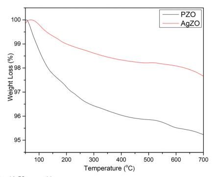
Fig. 8 TGA curves of PZO and AgZO nanoparticles.
