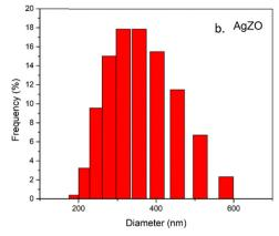
The DLS method was utilized to analyze the particle sizes of (a) PZO and (b) AgZO samples.
