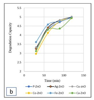
Fig. 10 Photocatalytic degradation (a) and degradation capacity (b) curve of CR dye with pure and several metal-doped ZnO nanoparticles.
