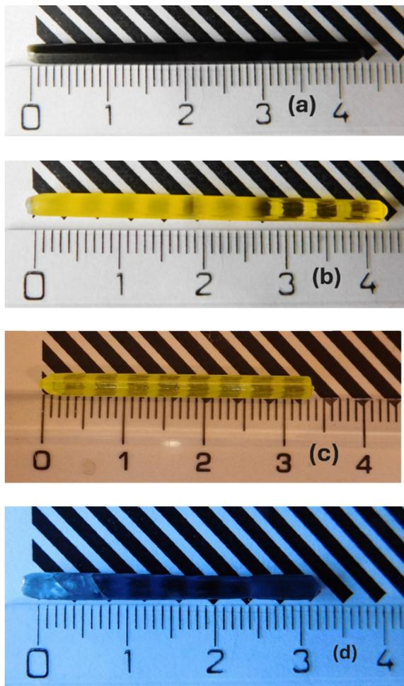
Fig. 1 Photographs of some of the grown crystals: (a)  $\text{Gd}_3\text{Sc}_2$  as grown; (b)  $\text{Gd}_3\text{Sc}_2$  air-annealed (1200 °C/12 h); (c)  $\text{Gd}_3\text{Ga}_{2.7}$  as grown; and (d)  $\text{Y}_3\text{Sc}_2\text{Al}_3\text{O}_{12}$  as grown.
