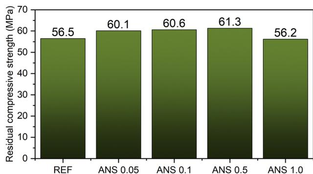
Fig. 13 Residual compressive strength measured after 24 h immersion in water.
