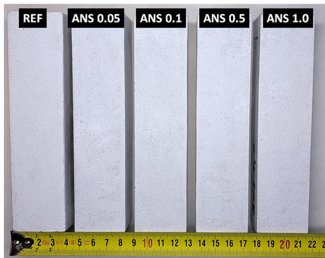
Fig. 4 Photograph of the prepared MOC-based composite samples.
