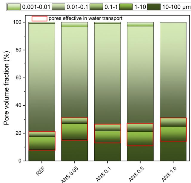
Fig. 12 Pore volume fraction determined by MIP analysis.
