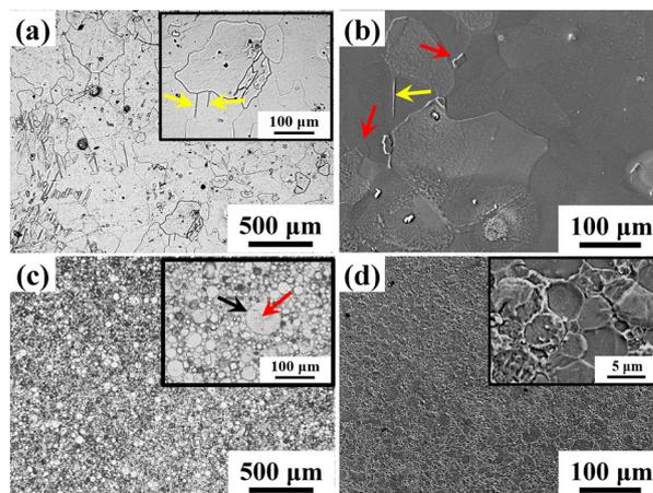
Fig. 5 (a) and (c) Optical and (b) and (d) scanning electron microscopy images of the zinc samples fabricated by (a) and (b) casting and (c) and (d) spark plasma sintering processes.
