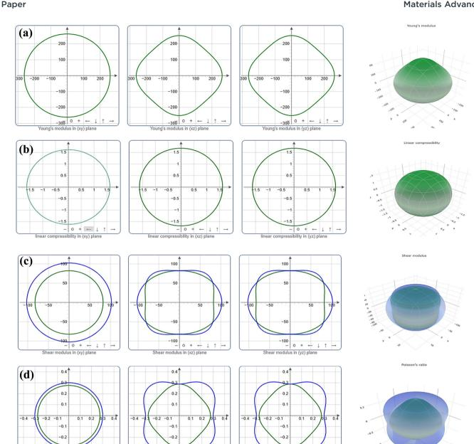
Fig. 3 Directional dependence of (a) Young's modulus (Y), (b) linear compressibility ( $\beta$ ), (c) shear modulus (G), and (d) Poisson's ratio ( $\nu$ ) of Ru<sub>3</sub>B<sub>2</sub>Th.
