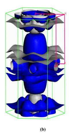
Fig. 7 The Fermi surfaces of (a) Ru<sub>3</sub>B<sub>2</sub>U and (b) Ru<sub>3</sub>B<sub>2</sub>Th.
