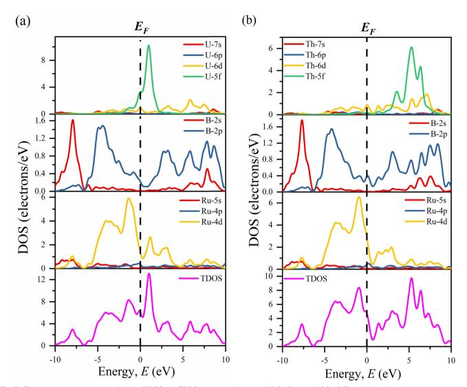
Fig. 6 The partial and total density of states (PDOS and TDOS, respectively) plots of (a) Ru<sub>3</sub>B<sub>2</sub>U and (b) Ru<sub>3</sub>B<sub>2</sub>Th as a function of energy.
