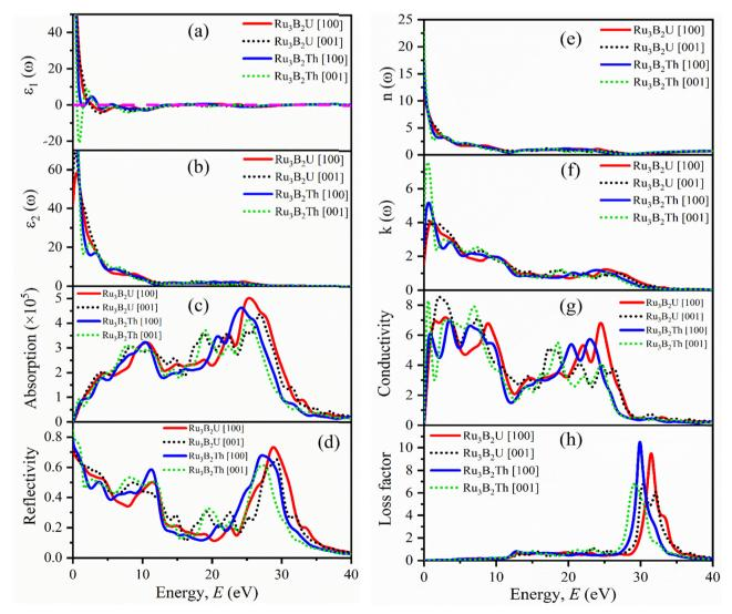
Fig. 10 (a)  $\varepsilon_1(\omega)$ , (b)  $\varepsilon_2(\omega)$ , (c) absorption coefficient, (d) reflectivity, (e)  $n(\omega)$ , (f)  $k(\omega)$ , (g) optical conductivity, and (h) energy loss function of Ru<sub>3</sub>B<sub>2</sub>X (X = Th, U) in the [001] and [100] direction
