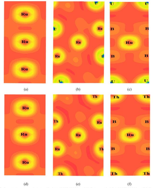
Fig. 8 Electronic charge density distribution of Ru<sub>3</sub>B<sub>2</sub>U in (a) (100), (b) (101), and (c) (110) planes and Ru<sub>3</sub>B<sub>2</sub>Th in (d) (100), (e) (101), and (f) (110) planes.
