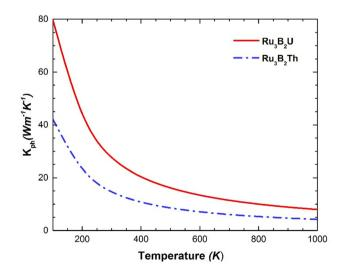
Fig. 9 Variation of lattice thermal conductivity of  $Ru_3B_2X$  (X = Th, U) as a function of temperature.
