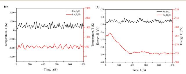
Fig. 2 Change of (a) temperature and (b) energy with time for  $Ru_3B_2U$  and  $Ru_3B_2Th$ .
