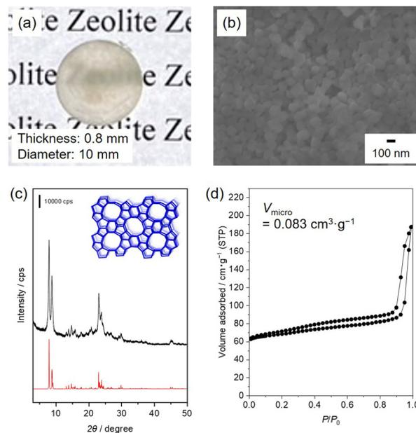
Fig. 1 Characterisation of a translucent silicalite-1 ceramic prepared under optimised SPS conditions. (a) Photograph, (b) cross-sectional SEM image, (c) PXRD pattern, and (d) N<sub>2</sub> adsorption-desorption isotherm. Silicalite-1<sub>70</sub> (100 mg) was sintered at 400 MPa and 500 °C for 5 min using a tungsten carbide die. The ramping rate was 32 °C min<sup>-1</sup>.
