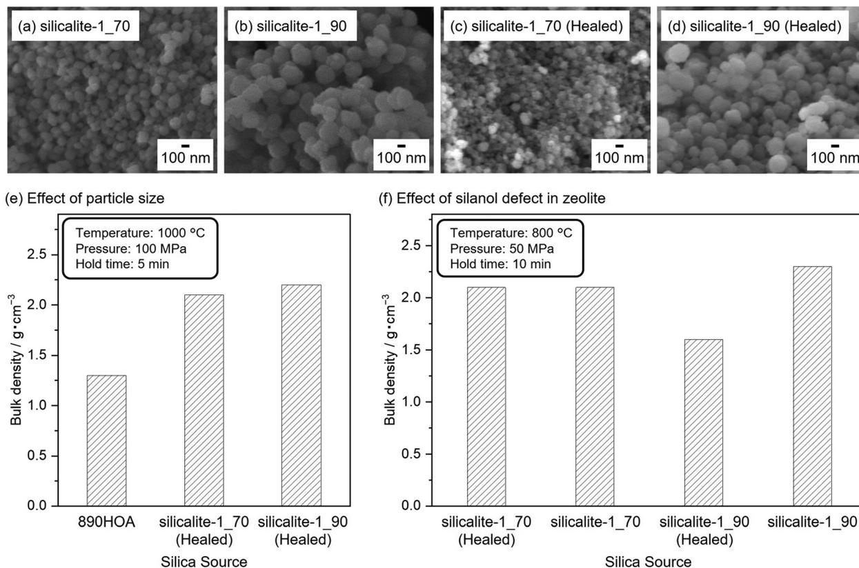
Fig. 3 SEM images of (a) silicalite-1\_70, (b) silicalite-1\_90, (c) silicalite-1\_70 (healed), and (d) silicalite-1\_90 (Healed). Effects of (e) particle size and (f) defects in silicalite-1 on the sinterability of various silica sources. All samples (330 mg) were sintered using the graphite die. The ramping rate was 70 °C min<sup>-1</sup>, and the other SPS conditions are given in the inset.
