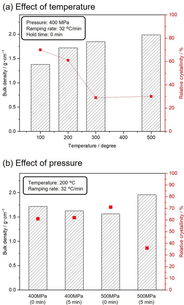
Fig. 4 Effect of (a) temperature and (b) pressure for bulk densities and relative crystallinities of sintered silicalite-1<sub>70</sub> samples. All samples (250 mg) were sintered by using the tungsten carbide die. Fixed conditions were described in the inset of each figure.
