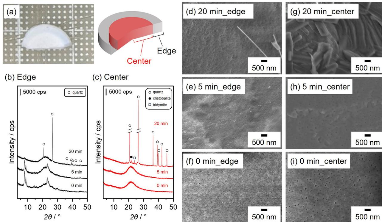
Fig. 5 (a) Photograph of bulk ceramic silicalite-1\_70 obtained by SPS treatment at 500 °C with a ramping rate of 32 °C min<sup>-1</sup> under 400 MPa for 0 min. (b) and (c) PXRD patterns and (d)–(i) cross-sectional SEM images of the edge and centre of sintered silicalite-1\_70 °C ceramics at varying times.
