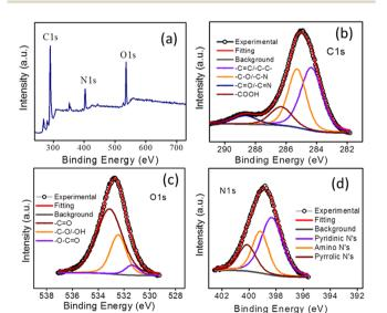
Fig. 2 (a) The XPS survey spectrum of PD-CNDs; (b)–(d) XPS fitting curves of C 1s, O 1s and N 1s of PD-CNDs.
