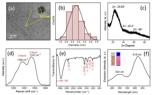
Fig. 1 (a) TEM image of PD-CNDs (inset: high resolution TEM image showing the lattice fringes with a d-spacing value of 0.19 nm) and (b) particle size distribution determined from the TEM image. (c) XRD profile, (d) Raman spectrum, (e) FT-IR spectrum and (f) fluorescence emission spectrum ( $\lambda_{ex}$ = 360 nm) of PD-CNDs (inset: image of PD-CNDs agueous dispersion under daylight and 365 nm UV light.).
