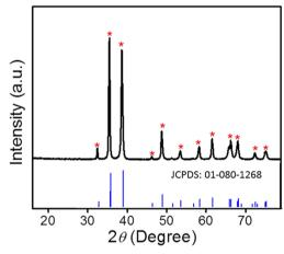
Fig. 8 XRD pattern of CuO synthesized from PD-CND@Cu.
