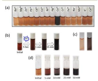
Fig. 3 (a) Visual sensing of Cu<sup>2+</sup> ions using PD-CNDs showing the selective response of cupric ions (mM) towards carbon nanodots. (b) Photographs showing the response to PD-CNDs to Cu<sup>2+</sup> at various time intervals. (c) PD-CND solution without and (left) and with (right) cupric ions. (d) Photographs showing the concentration dependent response of cupric ions (images captured after 30 min of Cu2+ ion (mM) solution addition).
