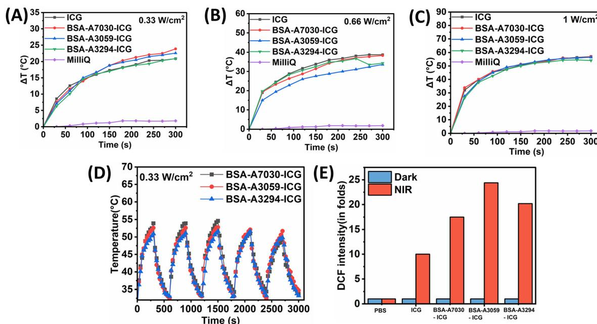
Fig. 5 (A)–(C) Photothermal temperature rise of ICG, BSA-A7030-ICG, BSA-A3059-ICG, and BSA-A3294-ICG with  $0.33$ ,  $0.66$  and  $1 \text{ W cm}^{-2}$ , respectively, when irradiated for 5 min; (D) photostability of BSA-ICG for five ON-OFF cycles; and (E) acellular ROS generation. All measurements were recorded in deionized water.
