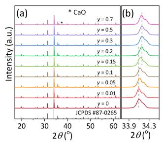
Fig. 3 (a) XRD patterns of the Ca<sub>14</sub>Zn<sub>6</sub>Al<sub>9.8-y</sub>B<sub>y</sub>Mn<sub>0.1</sub>Mg<sub>0.1</sub>O<sub>35</sub> phosphors sintered at 1250 °C for 5 h, (b) enlarged patterns around  $2\theta$  = 34.1°.
