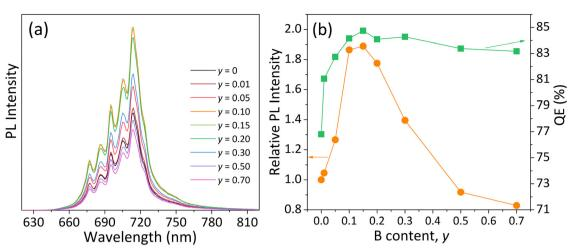
Fig. 5 (a) Room-temperature PL spectra of the  $Ca_{14}Zn_6Al_{9.8-V}B_vMn_{0.1}Mg_{0.1}O_{35}$  phosphors. (b) Dependence of the PL intensity and QE on the B-doping concentration
