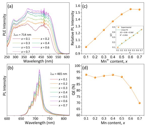
Fig. 6 (a) PLE ( $\lambda_{em}=714$  nm) and (b) PL ( $\lambda_{ex}=465$  nm) spectra of  $Ca_{14}Zn_6Al_{9.85-2x}B_{0.15}Mn_xMg_xO_{35}-0.42\%$   $B_2O_3$  phosphors sintered at 1240 °C for 4 h. Dependence of the integrated PL intensity (c) and QE (d) on the Mn-doping concentration (x) of the  $Ca_{14}Zn_6Al_{9.85-2x}B_{0.15}Mn_xMg_xO_{35}-0.42\%$   $B_2O_3$  phosphors.
