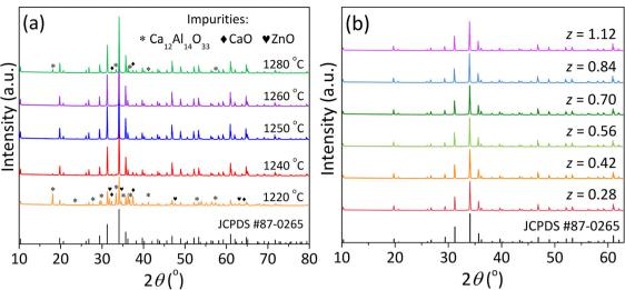
Fig. 1 XRD patterns of (a)  $Ca_{14}Zn_6Al_{9.8}Mn_{0.1}Mg_{0.1}O_{35}$  phosphors sintered at various temperatures for 5 h, and (b)  $Ca_{14}Zn_6Al_{9.8}Mn_{0.1}Mg_{0.1}O_{35} - z$  wt%  $B_2O_3$  phosphors sintered at 1240 °C for 4 h. The standard diffraction pattern of  $Ca_{14}Zn_6Al_{10}O_{35}$  from JCPDS (No. 87-0265) is provided at the bottom of the figure.
