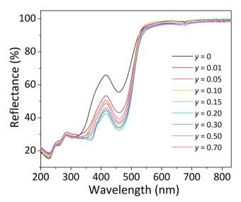
Fig. 4 Reflectance spectra of the  $Ca_{14}Zn_6Al_{9.8-y}B_yMn_{0.1}Mg_{0.1}O_{35}$  phosphors.
