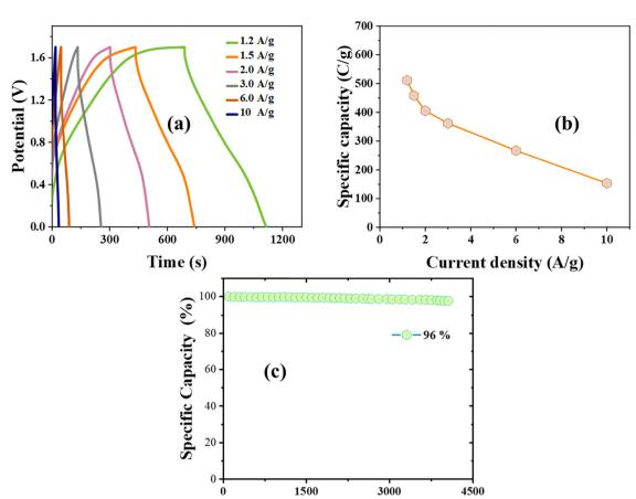
**GCD Cycles (Number)** Fig. 8 (a) S3//AC real device GCD, (b)  $Q_s$  and (c) stability test result.
