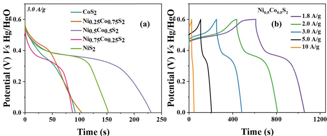
Fig. 4 (a) Discharge curves of all the samples at current density of  $3 \text{ A g}^{-1}$ . (b) GCD results of S3 at different current density values.
