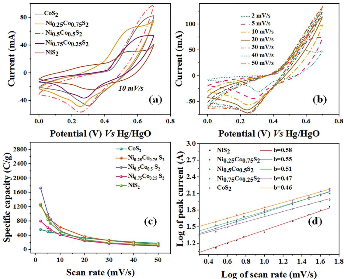
Fig. 3 (a) CV profiles of all the samples recorded at the scan rate of  $10 \text{ mV s}^{-1}$ , elucidating their redox active nature, (b) CV profile of S3 with dominant performance among all, (c)  $Q_s$  calculated for all the samples while being tested at different sweep rates, and (d)  $b$ -value fitting for all the samples.
