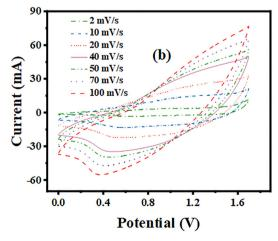
Fig. 7 CV profile of (a) S3 and AC in three cell configurating elaborating their different storage mechanisms, (b) S3//AC real device.
