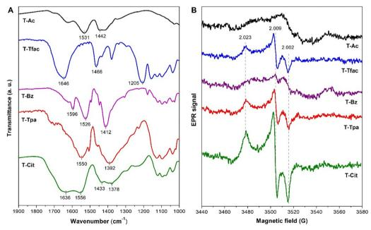
Fig. 4 FTIR spectra (A) and EPR spectra, recorded in air at room temperature, in the dark (B), of the studied TiO<sub>2</sub>-carboxylate samples with the ligand/Ti molar ratio = 0.2 (g values of the EPR signals are indicated)
