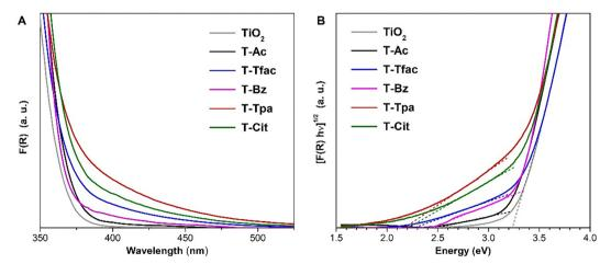
Fig. 5 DRUV-vis spectra of the studied TiO<sub>2</sub>-carboxylate samples with the ligand/Ti molar ratio = 0.2 and reference sol-gel TiO<sub>2</sub> (magnification of the normalized Kubelka-Munk function of reflectance, (A)); corresponding Tauc plot for indirect band gap transitions (B).
