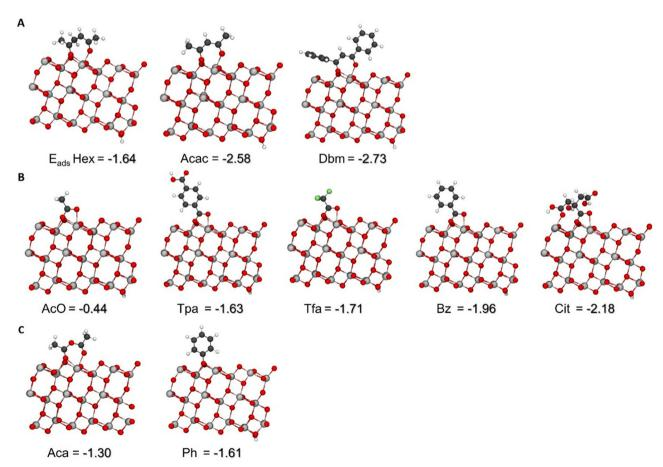
Fig. 2 Optimized structure of the interaction of the TiO<sub>2</sub> (101) surface containing oxygen vacancy VO1 with diketones (A), carboxylic acids (B) and other classes of ligands (C) and the corresponding adsorption energies ( $E_{ads}$ , eV). Ti, C, H, O and F atoms are represented in ball and sticks and depicted in gray, dark gray, white, red and green respectively.
