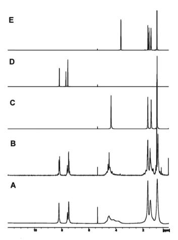
Fig. 3  $^{1}$ H NMR spectra (CD<sub>2</sub>Cl<sub>2</sub>, RT, 600 MHz) of Ti(OBu<sup>n</sup>)<sub>4</sub>:HBa 1:1 reaction mixture (A); Ti(OBu<sup>n</sup>)<sub>4</sub>:HBz 1:1 after removal of butanol (B); Ti(OBu<sup>n</sup>)<sub>4</sub> (C); HBz (D); and butanol (E).
