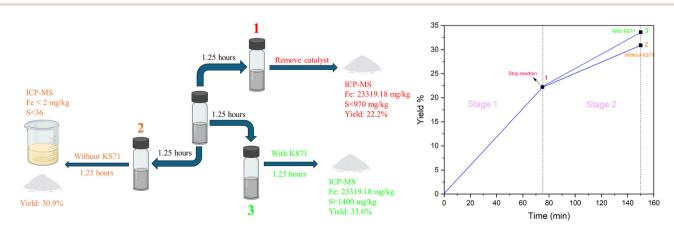
Fig. 11 Leaching test procedure: (1) reaction stopped; (2) reaction without KS71; (3) continuous reaction with KS71.
