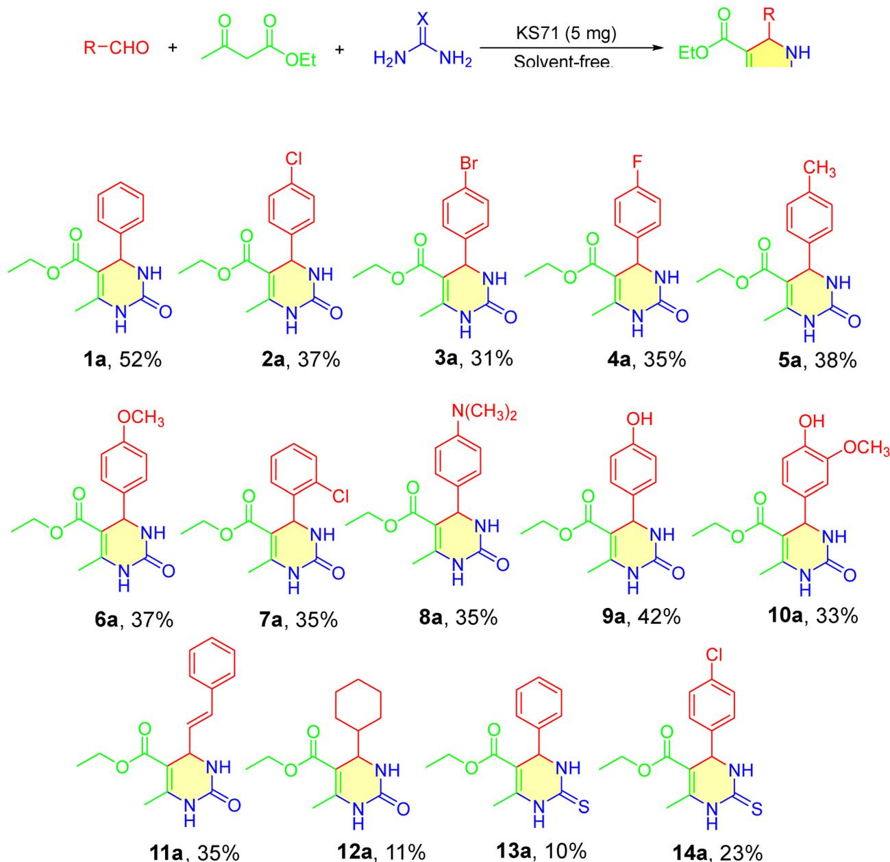
Scheme 6 DHPM derivatives synthesis substrate scope. Reaction conditions: aldehydes (1 mmol), ethyl acetoacetate (1 mmol), urea/thiourea (1 mmol), KS71 (5 mg), under solvent-free conditions.
