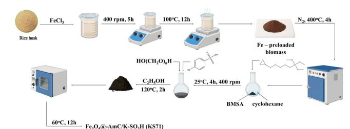
Scheme 2 Synthesis process of KS71 catalyst.
