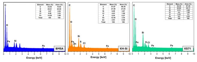
Fig. 4 EDX analysis of BMSA, KH-Si, and KS71.
