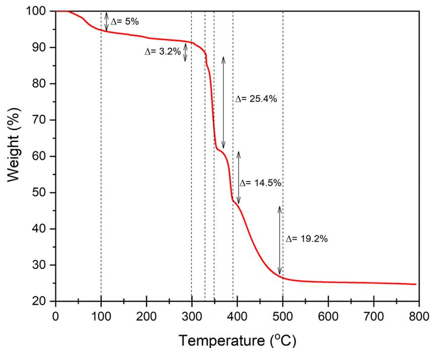
Fig. 6 Thermogravimetric analysis (TGA) curves for KS71.
