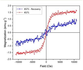
Fig. 10 Magnetization curves of KS71 (red) and recovered KS71 (blue) at room temperature.
