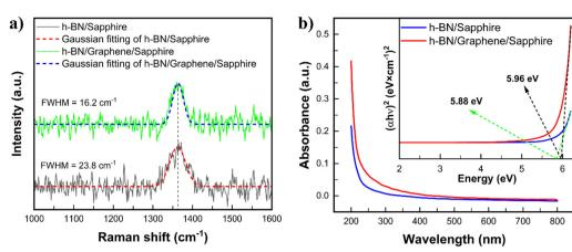
Fig. 4 Raman spectrum of h-BN grown on sapphire and on graphene (a) and UV-Vis absorption spectrum of h-BN grown on sapphire (black line) and graphene (red line); inset: Tauc plot for bandgap identification (b).
