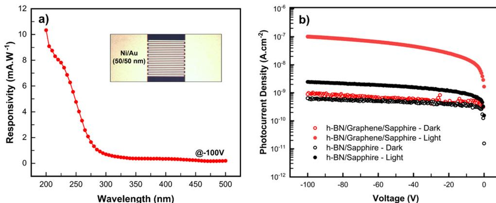
Fig. 7 (a) Photoresponse spectra of vdWHT h-BN/graphene/sapphire photodetector at a  $-100$ -V bias voltage; inset: top-view of the fabricated devices and (b)  $I$ - $V$  characteristics of the vdWHT h-BN/graphene/sapphire and h-BN/sapphire photodetectors under a 254-nm light irradiation.
