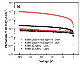
Fig. 7 (a) Photoresponse spectra of vdWHT h-BN/graphene/sapphire photodetector at a -100-V bias voltage; inset: top-view of the fabricated devices and (b) I-V characteristics of the vdWHT h-BN/graphene/sapphire and h-BN/sapphire photodetectors under a 254-nm light irradiation.
