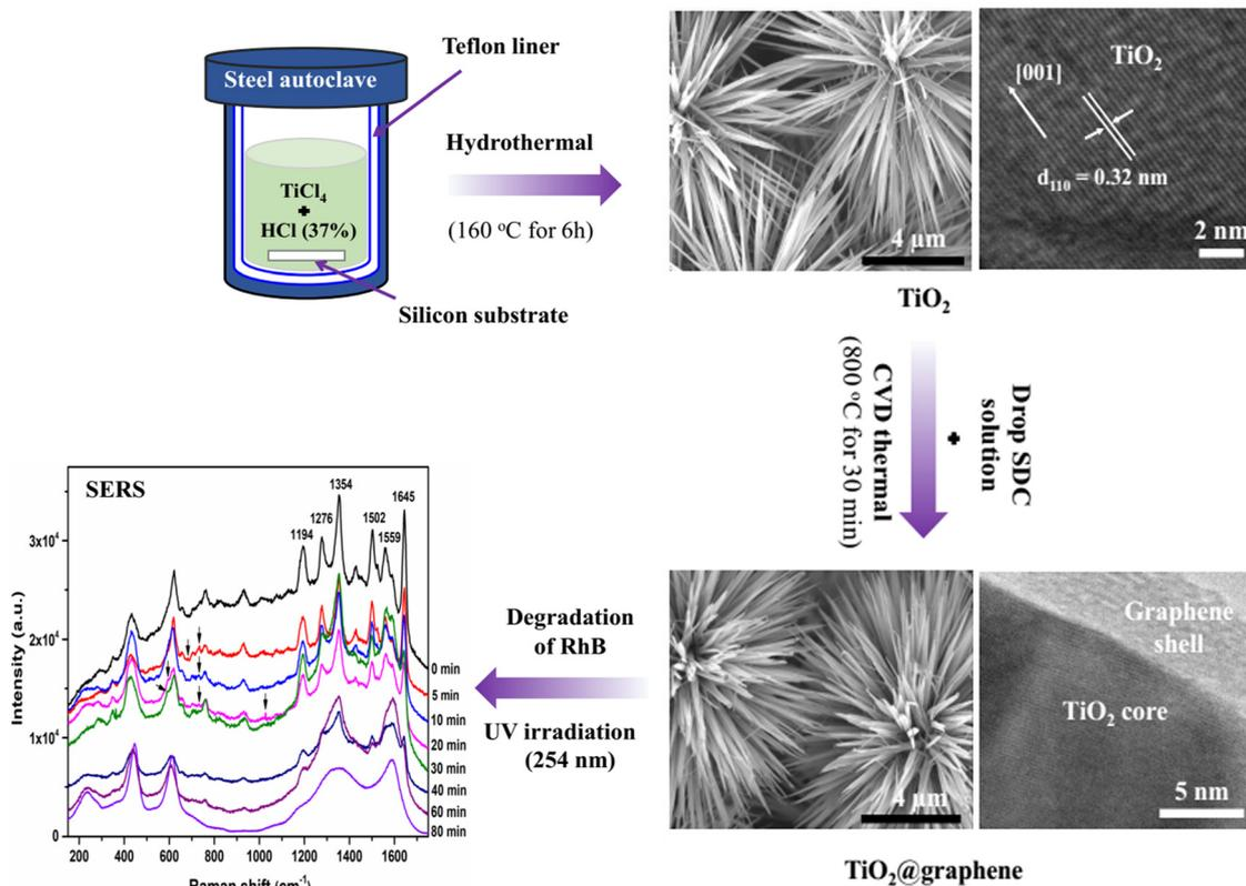
Scheme 1 Fabrication procedure and RhB degradation of TiO<sub>2</sub>@graphene SERS substrates under the irradiation of UV light.
