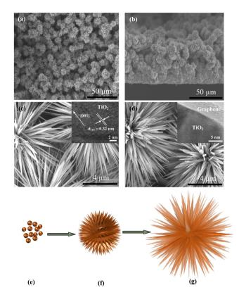
Fig. 1 Surface and cross sectional SEM images (a) and (b) of UTs on the  $SiO_2$  substrate, high-magnification SEM images and the insets are HRTEM images of (c) UTs and (d) UTGs. Schematic illustration of the formation process of the UTs: (e) nucleation, (f) dissolution and recrystallization, and (g) self-assembly.
