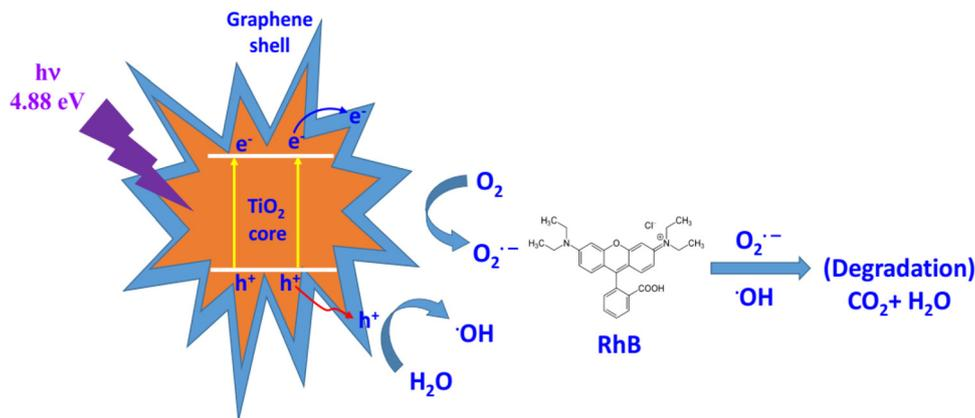
Fig. 8 Degradation mechanism for UTG towards RhB.
