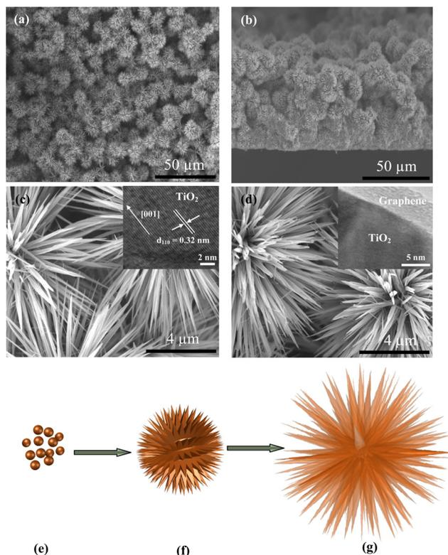
**Fig. 1** Surface and cross sectional SEM images (a) and (b) of UTs on the SiO<sub>2</sub> substrate, high-magnification SEM images and the insets are HRTEM images of (c) UTs and (d) UTGs. Schematic illustration of the formation process of the UTs: (e) nucleation, (f) dissolution and recrystallization, and (g) self-assembly.
