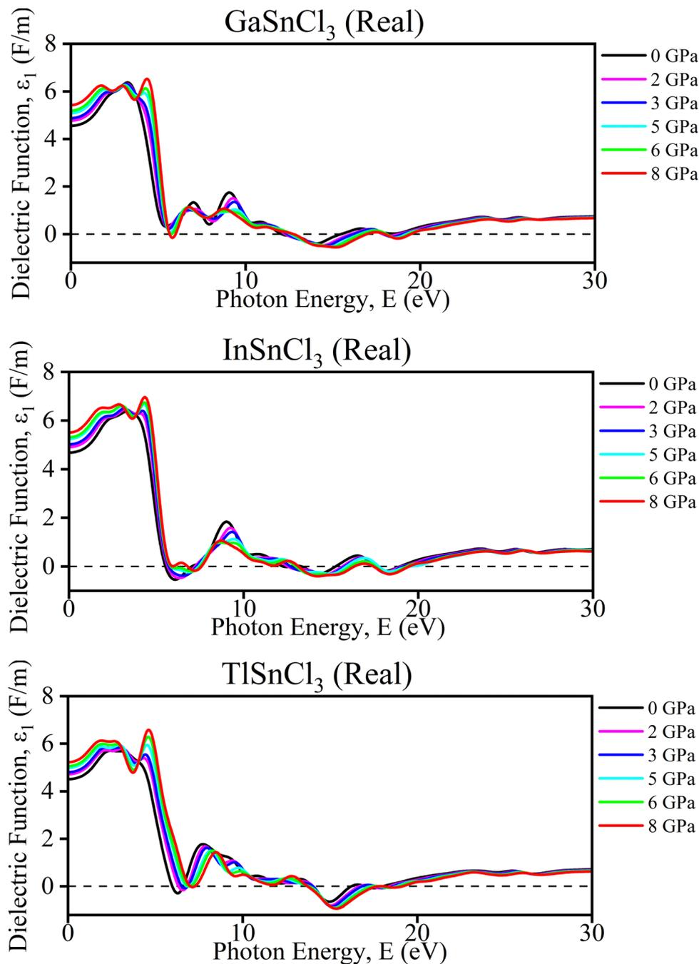
Fig. 10 Calculated pressure induced real spectra of dielectric function ( $\epsilon$ ) for  $\text{ASnCl}_3$  ( $A = \text{Ga}, \text{In}, \text{and Tl}$ ).
