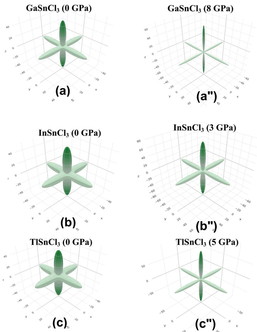
Fig. 14 Young's modulus of (a) and (a'')  $\text{GaSnCl}_3$ , (b) and (b'')  $\text{InSnCl}_3$ , and (c) and (c'')  $\text{TlSnCl}_3$ .
