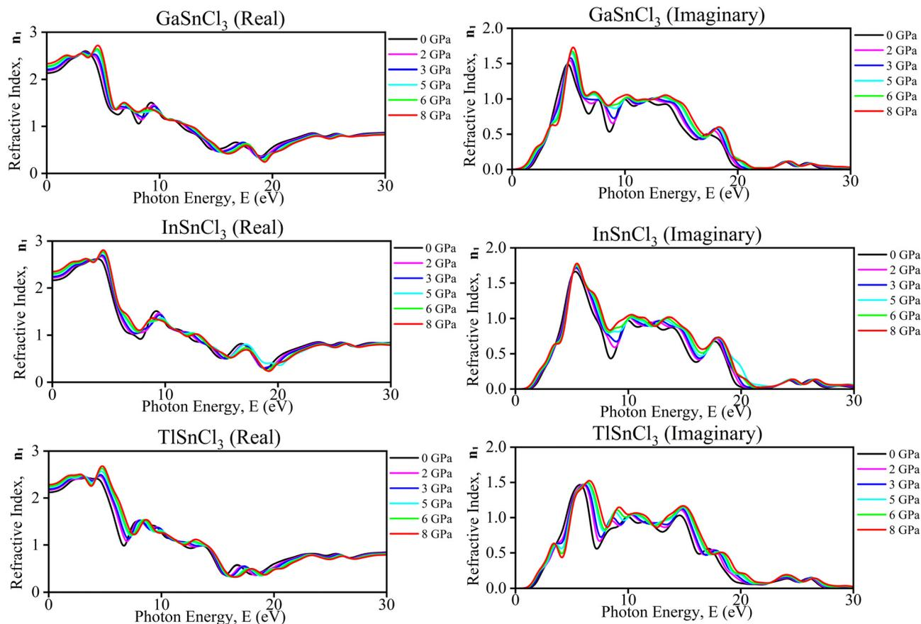
Fig. 12 Calculated pressure induced spectra of the refractive index ( $n_1$ ) of ASnCl<sub>3</sub> (A = Ga, In, and Tl).
