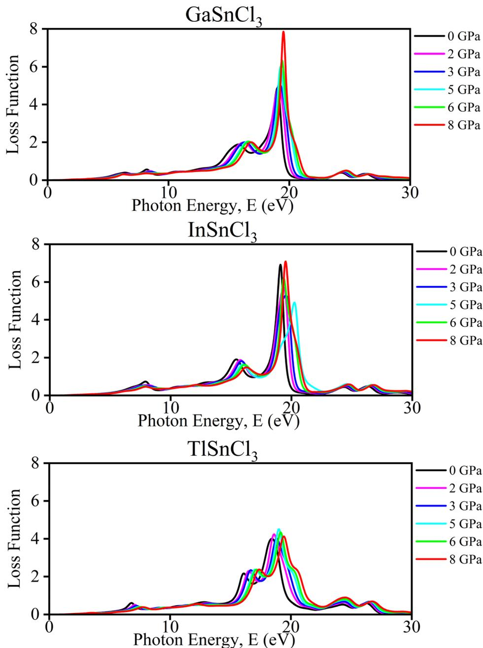
Fig. 11 Calculated pressure-induced spectra of loss function of A<sub>3</sub>SnCl<sub>3</sub> (A = Ga, In, and Tl).
