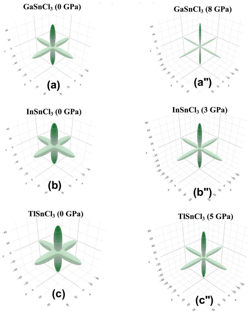
Fig. 16 Poisson's ratio of (a) and (a'') GaSnCl<sub>3</sub>, (b) and (b'') InSnCl<sub>3</sub>, and (c) and (c'') TlSnCl<sub>3</sub>.
