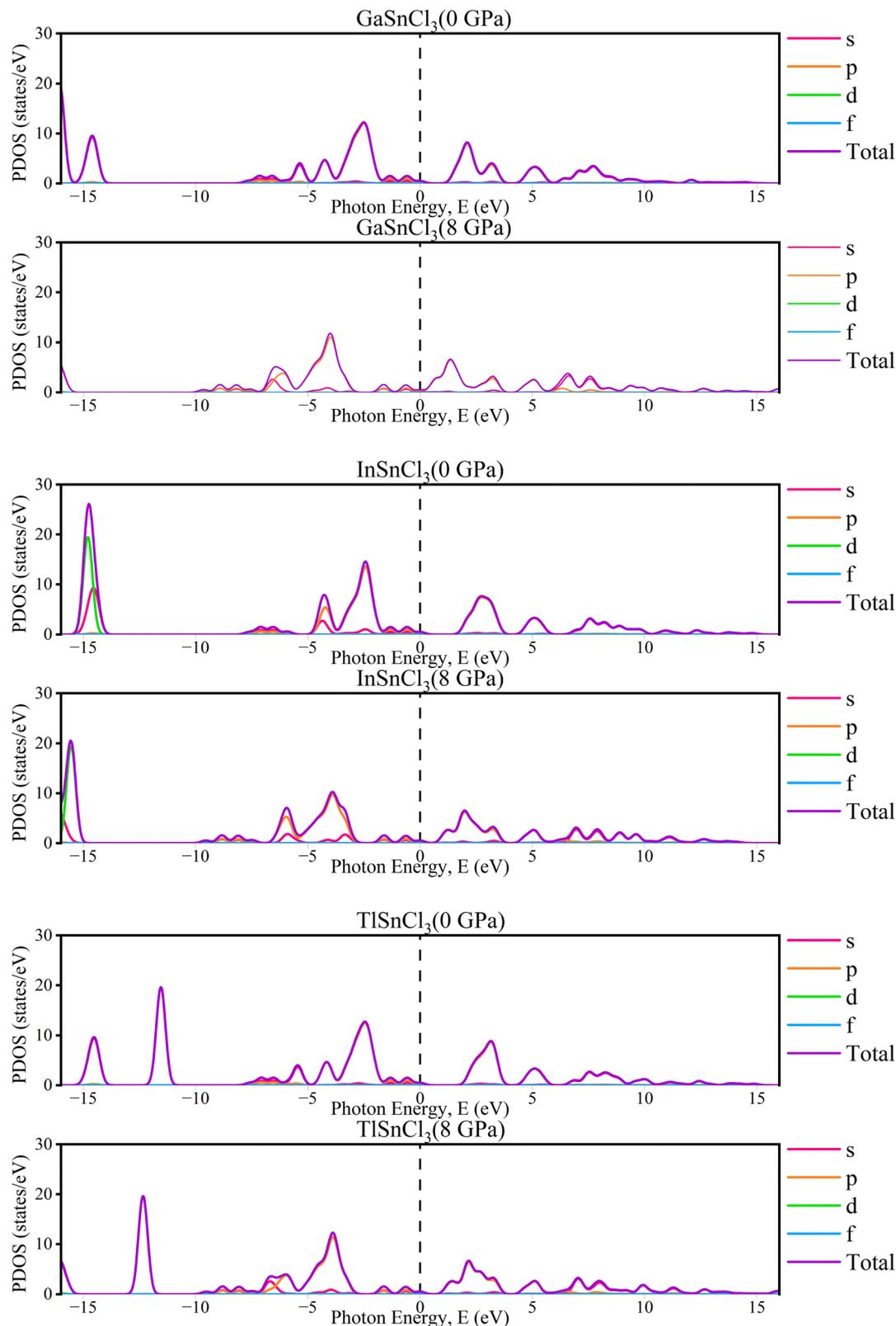
Fig. 5 The partial density of states (PDOS) of  $ASnCl_3$  ( $A = Ga, In, \text{ and } Tl$ ) under pressure.
