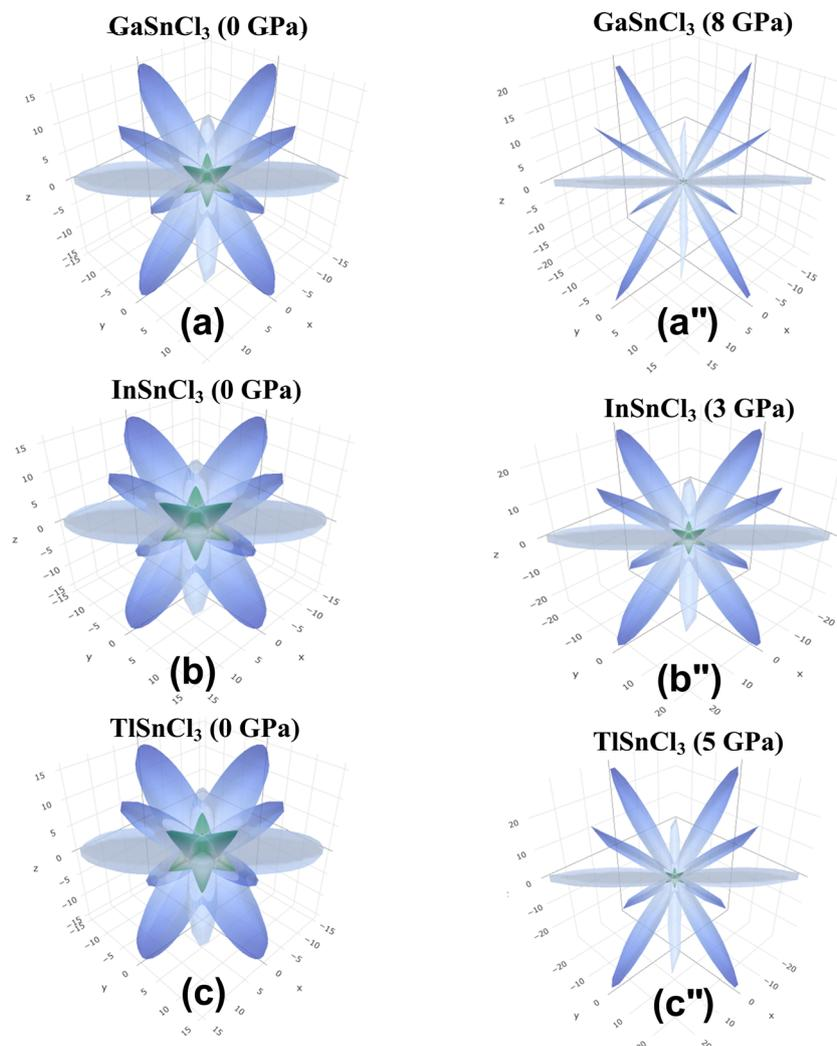
Fig. 15 Shear modulus of (a) and (a'')  $\text{GaSnCl}_3$ , (b) and (b'')  $\text{InSnCl}_3$ , and (c) and (c'')  $\text{TlSnCl}_3$ .
