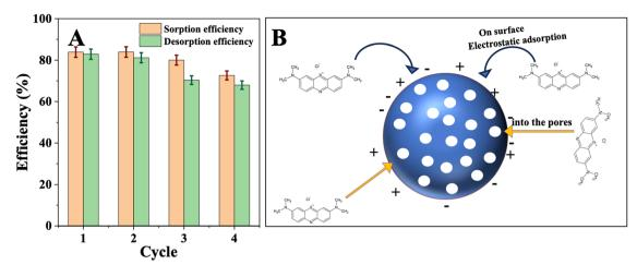
(A) Sorption/desorption cycles of MB dye onto CP NPs. (B) Scheme of the mechanism of MB with CP NPs
