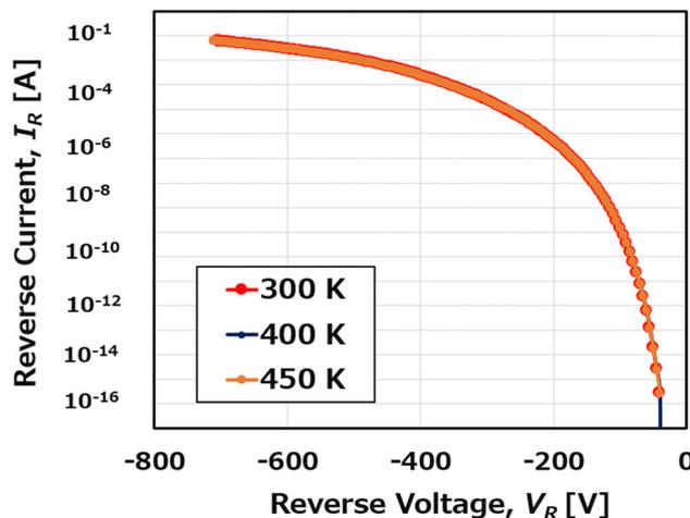
Fig. 6 Simulated temperature-dependent reverse breakdown characteristics of the GaN/ $\beta$ -Ga<sub>2</sub>O<sub>3</sub> p–n diode.
