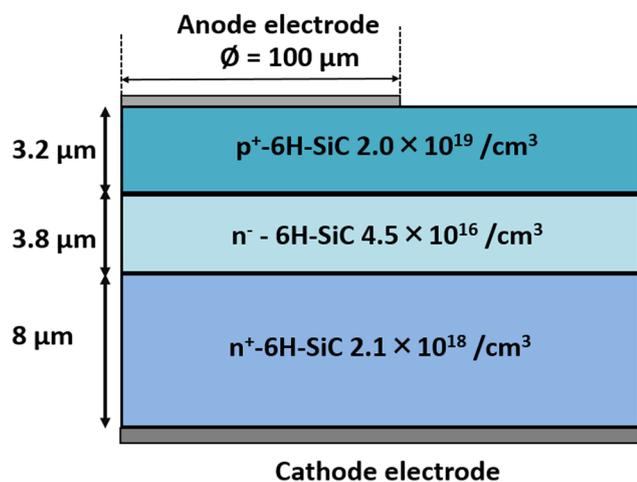
Fig. 8 Schematic representation of the simulated 6H-SiC p-n diode.<sup>52</sup>
