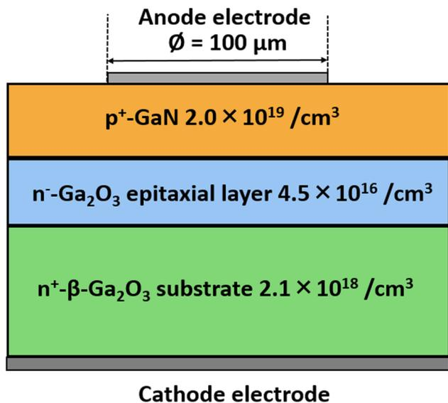
Fig. 1 Schematic representation of the simulated GaN/ $\beta$ -Ga<sub>2</sub>O<sub>3</sub> hetero-junction p-n diode.
