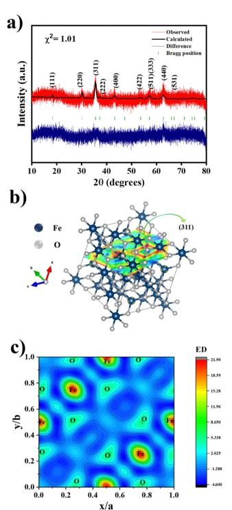
Fig. 1 (a) Rietveld refinement analysis of OA-coated  $Fe_3O_4$  NPs, (b) Crystal structure of OA-coated  $Fe_3O_4$  NPs with the (311) crystal plane highlighted, and (c) electron density map showcasing atomic distribution.
