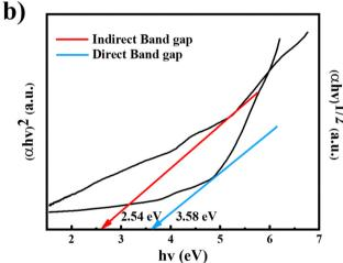
Fig. 2 (a) FTIR spectra of OA-coated Fe $_3$ O $_4$  NPs, (b) Tauc plot for direct and indirect band gap energy of OA-coated Fe $_3$ O $_4$  NPs.
