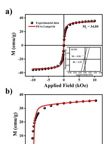
Fig. 4 (a) Room temperature M-H curve of the OA-coated Fe<sub>3</sub>O<sub>4</sub> NPs with a Langevin function fit, confirming their superparamagnetic behavior. The inset provides an enlarged view of the M-H curve near the origin, highlighting the negligible coercivity and remanence. (b) LAS fit of the M-Hcurve, further validating the magnetic characteristics and saturation magnetization of the NPs.
