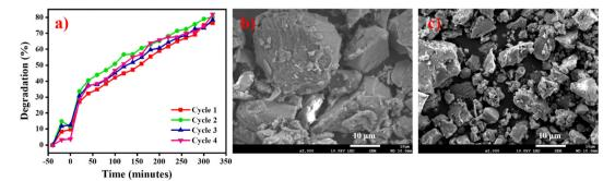
Fig. 9 (a) Stability test of the OA-coated Fe<sub>3</sub>O<sub>4</sub> NPs as a photocatalyst, demonstrating their reusability over multiple cycles. (b) FESEM images of OAcoated Fe<sub>3</sub>O<sub>4</sub> NPs showing the morphology before the degradation experiment and (c) after the recyclability test, highlighting structural changes.
