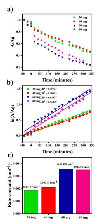
Fig. 8 (a)  $A/A_0$  vs. time graph, (b) rate kinetics and (c) bar graph representing the rate constants at different catalyst dosage.
