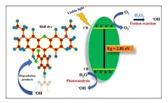
Fig. 10 Schematic representation of RhB dye degradation in presence of OA-coated  $Fe_3O_4$  NPs under visible light irradiation.
