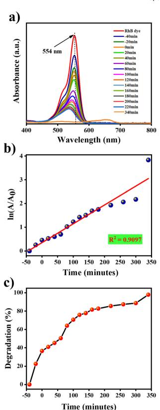
Fig. 7 (a) Absorbance spectra, (b) first order kinetic plot of  $ln(A/A_0)$ vs. time, (c) degradation efficiency of RhB dye using OA-coated Fe<sub>3</sub>O<sub>4</sub> NPs
