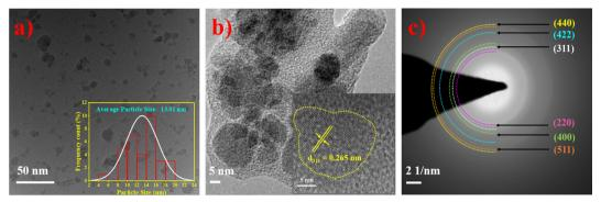
Fig. 3 (a) TEM micrograph of the OA-coated Fe<sub>3</sub>O<sub>4</sub> NPs with the inset showing the particle size distribution histogram, (b) HRTEM image of the NPs showing OA coating on NPs. Inset of the figure shows the lattice spacing corresponding to (311) plane. (c) SAED pattern illustrating multiple solid rings indicating polycrystalline nature of the NPs.
