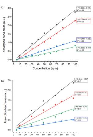
Fig. 6 Dependence of the absorbance band areas on concentration after 60 minutes of exposition using 5 μm film: (a) P3HB4HB and (b) PHO.
