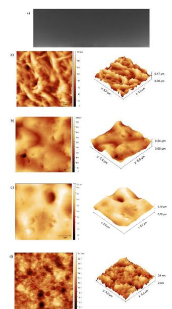
Fig. 3 AFM scan of a 5  $\mu$ m  $\times$  5  $\mu$ m area of (a) P3HB3HV film, (b) P3HB3HH film, (c) P3HB4HB film and (d) PHO film prepared by knife coating on a silicon wafer.
