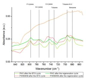
Fig. 8 The IR spectrum of the PHO and P3HB4HB film (5  $\mu$ m) before and after the regeneration cycle for 50 ppm BTX solution (flowrate of 3 mL min<sup>-1</sup>).
