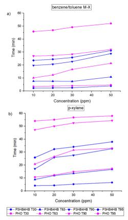
Fig. 7 Time dependence of the IR signal (at 30%, 63%, 90% and 95% of saturated signal) as a function of concentration for: (a) benzene/toluene M-X and (b) p-xylene using 5 μm thick PHA films.
