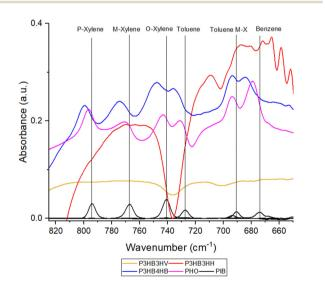
Fig. 4 The absorbance spectrum of 50 ppm BTX in water using PHA films (5  $\mu$ m) after 60 minutes of exposure to solution and a flow rate of 3 mL min<sup>-1</sup>, compared with 5 ppm BTX solution obtained in the same conditions with 5 µm (polyisobutylene film), showing the shift in the position of the absorbance bands (PHA films were fabricated by knife-coating, and PIB film by spin-coating).
