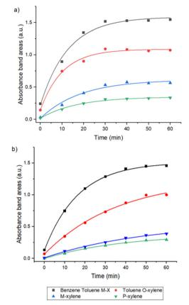
Fig. 5 Dependence of the IR absorbance band area on time using 5  $\mu$ m (a) P3HB4HB and (b) PHO polymer films to analyse 50 ppm BTX solution at a flow rate of 3 mL min<sup>-1</sup>.
