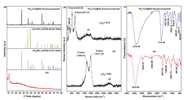
Fig. 4 XRD diffraction patterns (a), Raman spectra (b), and FTIR spectra (c) of GO and the mycogenic TiO<sub>2</sub>-CuO@GO bionanocomposite.
