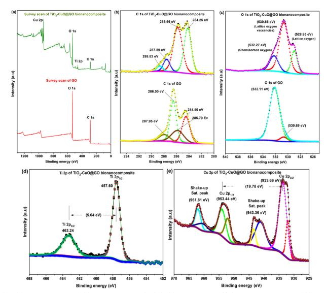
Fig. 5 XPS full scan survey spectra of GO and the mycogenic  $TiO_2$ –CuO@GO bionanocomposite (a), C 1s high-resolution spectra of GO and  $TiO_2$ –CuO@GO (b), O 1s high-resolution spectra of GO and  $TiO_2$ –CuO@GO (c), Ti 2p high-resolution spectrum of  $TiO_2$ –CuO@GO (d), and Cu 2p high-resolution spectrum of  $TiO_2$ – $TiO_2$ 00 (e).
