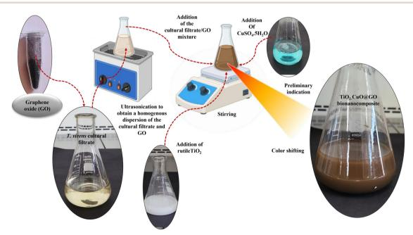
Fig. 2 A schematic diagram represents the mycogenic preparation process of the colloidal suspension containing TiO2-CuO@GO bionanocomposite using T. virens cultural filtrate
