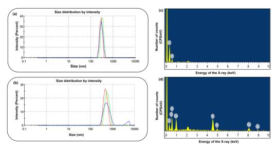
Fig. 6 Average particle size distribution determined by DLS (a) and (b) and FESEM-EDX analysis (c) and (d) for GO and TiO2-CuO@GO, respectively.
