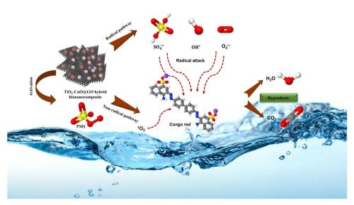
Fig. 13 Schematic diagram representing the catalytic degradation of CR via PMS-assisted catalytic activation by TiO2-CuO@GO bionanocomposite.
