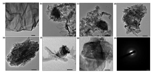
Fig. 7 Morphological characterization using HRTEM showing the ultra-morphological structure of GO (a) and TiO2-CuO@GO bionanocomposite (b)-(f) at different magnification scales (50 and 100 nm), lattice fringes (g), and SAED pattern of the bionanocomposite (h).
