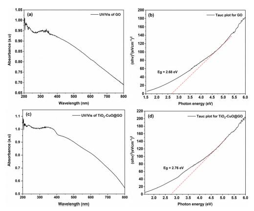
Fig. 3 UV-Vis spectra (a) and (c) and Tauc plot band gap energy ( $E_g$ ) (b) and (d) of GO nanosheets and TiO<sub>2</sub>-CuO@GO bionanocomposite, respectively.
