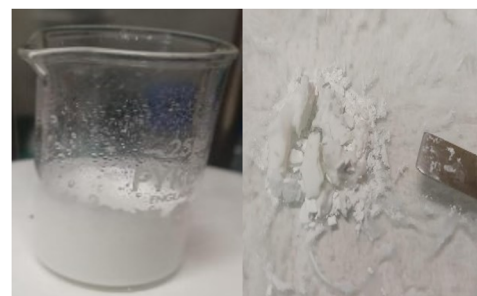
Fig. 1 ZCHNI1 synthesis: precipitate at the end of the reaction in the DES (left) and after water rinsing and drying (right).
