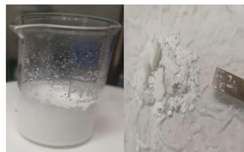
Fig. 1 ZCHNI1 synthesis: precipitate at the end of the reaction in the DES (left) and after water rinsing and drying (right).
