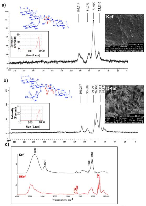
Fig. 1 Characterization of the native kefiran (Kef) and dialdehyde kefiran (DKef). The size distribution, SEM image, and <sup>13</sup>C NMR spectra of the (a) Kef and (b) DKef; (c) ATR-FTIR spectra of the Kef and DKef.
