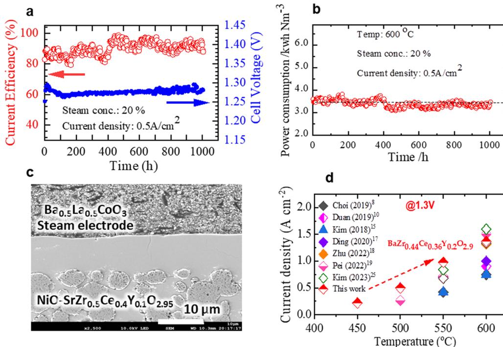
Fig. 6 (a) Long-term durability test of the BSZCY9144362-based cell at 600 °C. (b) Calculated amount of electricity to produce 1 N m<sup>3</sup> of H<sub>2</sub> as a function of time. (c) Microstructure of cell post measurement. (d) Performance comparison of our BZCY44362-based cell with similar electrolyte composition reported in the literature.
