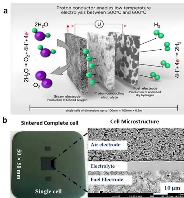
Fig. 1 (a) Schematic illustration of a steam proton conducting electrolysis cell (PCEC). (b) BZCY44362-based cell in the end-fired state with the microstructure after reduction.
