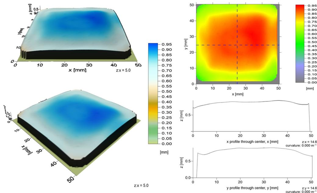
Fig. 4 Curvature and surface flatness of the as-fabricated 50 mm  $\times$  50 mm planar protonic electrolysis half-cells with the configuration  $\text{BaZr}_{0.44}\text{Ce}_{0.36}\text{Y}_{0.2}\text{O}_{3-\delta}$  |  $\text{NiO-SrZr}_{0.5}\text{Ce}_{0.4}\text{Y}_{0.1}\text{O}_{3-\delta}$  after sintering at 1350  $^{\circ}\text{C}/5$  h, evaluated by white-light topography measurement.
