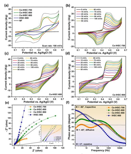
Fig. 9 (a) CV profiles of IHSC-900 and Ce-IHSC-x at a constant scan rate of 100 mV s<sup>-1</sup>; CV profiles of (b) Ce-IHSC-700, (c) Ce-IHSC-800, (d) Ce-IHSC-900 at scan rates from 5 to 100 mV s<sup>-1</sup>, (e) Nyquist plots for IHSC-900 and Ce-IHSC-x; inset depicts the high-frequency intercept of Nyquist plots and (f) bode plots for IHSC-900 and Ce-IHSC-x
