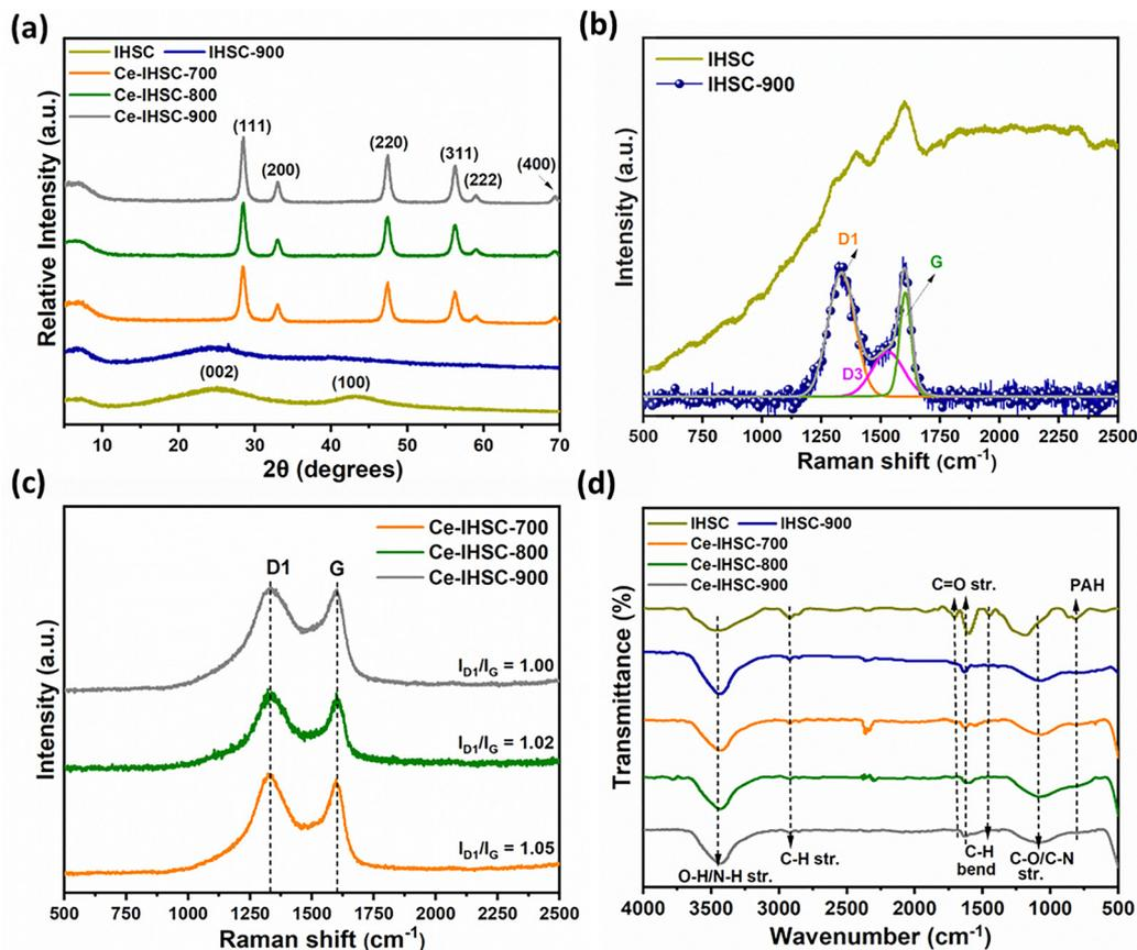
Fig. 2 (a) XRD patterns of IHSC, IHSC-900, and Ce-IHSC-*x*, (b) Raman spectra of IHSC, IHSC-900, (c) Raman spectra of Ce-IHSC-*x*, and FT-IR spectra of IHSC, IHSC-900, and Ce-IHSC-*x*.
