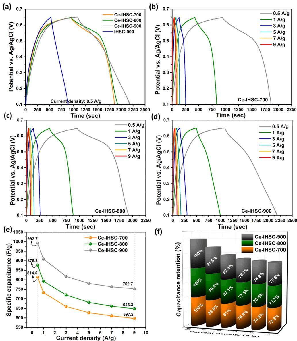
Fig. 10 (a) GCD plots of IHSC-900 and Ce-IHSC-*x* at a current density of 0.5 A g<sup>-1</sup>; GCD plots of (b) Ce-IHSC-700, (c) Ce-IHSC-800, and (d) Ce-IHSC-900 at current densities from 0.5 to 9 A g<sup>-1</sup>, (e) trend of specific capacitance vs. applied current density, and (f) capacitance retention vs. applied current density.
