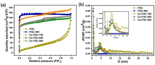
(a)  $N_2$  adsorption-desorption and (b) pore size distribution plots for IHSC, IHSC-900, and Ce-IHSC-x at 77 K.
