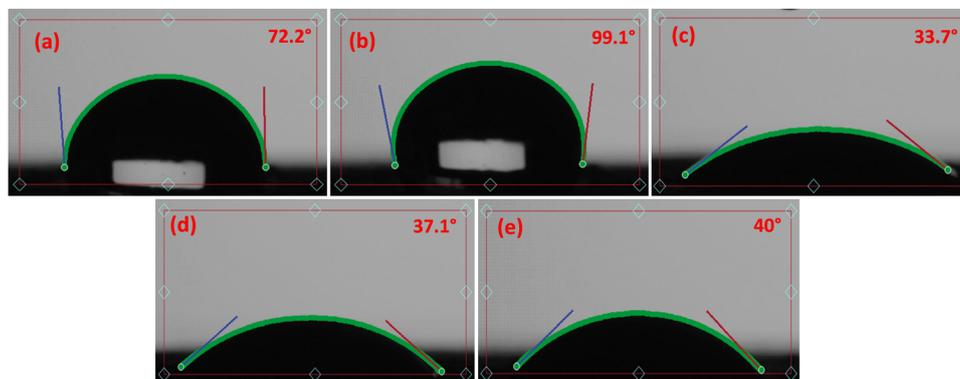
Fig. 8 Contact angle measurements for (a) IHSC, (b) IHSC-900, (c) Ce-IHSC-700, (d) Ce-IHSC-800, and (e) Ce-IHSC-900.
