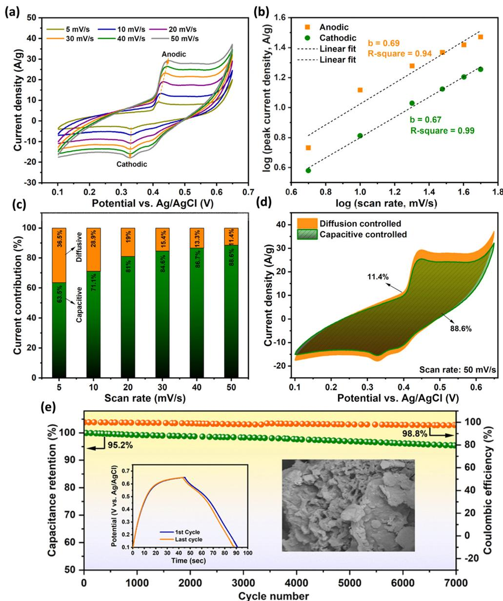
**Fig. 11** (a) CV profiles of Ce-IHSC-900 at scan rates from 5 to 50  $\text{mV s}^{-1}$ , (b) plot showing  $\log(\text{scan rate})$  vs.  $\log(\text{peak current density})$ , (c) current contribution from diffusion and capacitive processes at different applied scan rates, (d) CV profile showing deconvoluted diffusion and capacitive contribution at 50  $\text{mV s}^{-1}$ , and (e) cyclic stability plot of Ce-IHSC-900 measured at 9  $\text{A g}^{-1}$ .
