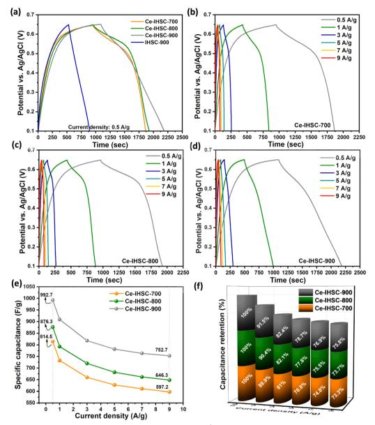
Fig. 10 (a) GCD plots of IHSC-900 and Ce-IHSC-x at a current density of 0.5 A  $g^{-1}$ ; GCD plots of (b) Ce-IHSC-700, (c) Ce-IHSC-800, and (d) Ce-IHSC-900 at current densities from 0.5 to 9 A  $g^{-1}$ , (e) trend of specific capacitance x. applied current density, and (f) capacitance retention x. applied current density.
