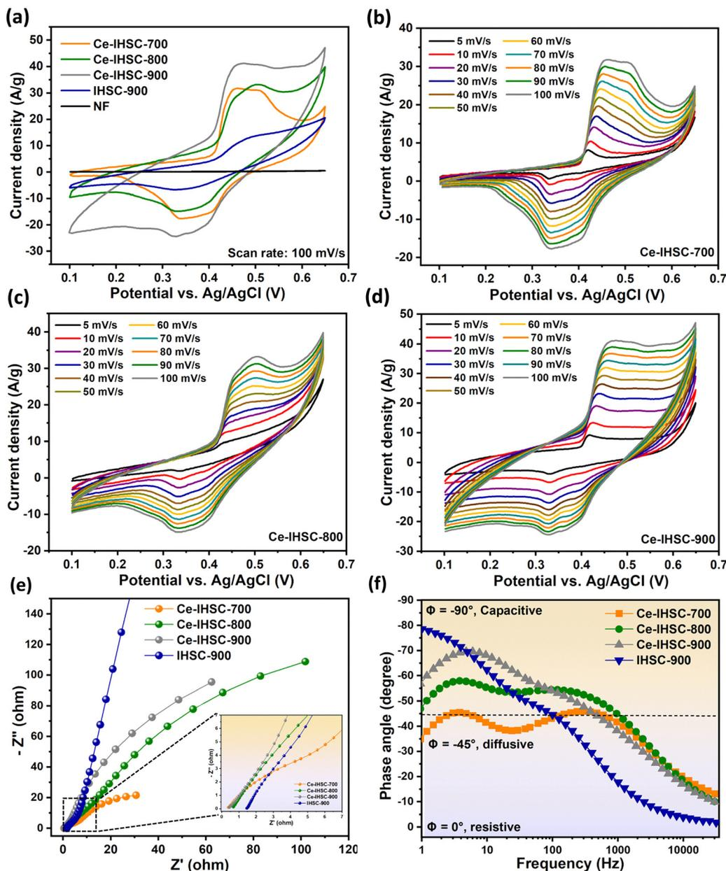
Fig. 9 (a) CV profiles of IHSC-900 and Ce-IHSC-*x* at a constant scan rate of 100 mV s<sup>-1</sup>; CV profiles of (b) Ce-IHSC-700, (c) Ce-IHSC-800, (d) Ce-IHSC-900 at scan rates from 5 to 100 mV s<sup>-1</sup>, (e) Nyquist plots for IHSC-900 and Ce-IHSC-*x*; inset depicts the high-frequency intercept of Nyquist plots and (f) bode plots for IHSC-900 and Ce-IHSC-*x*.
