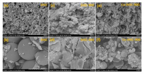
Fig. 3 FESEM images of (a) and (b) IHSC, (c) and (d) IHSC-900, and (e) and (f) Ce-IHSC-900.
