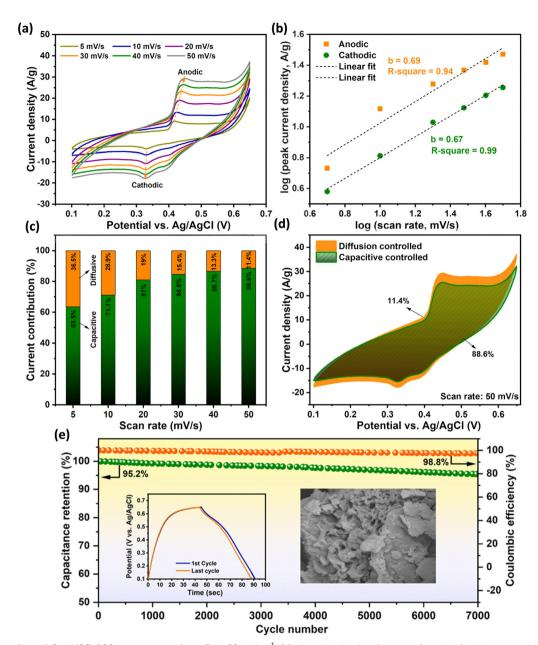
Fig. 11 (a) CV profiles of Ce-IHSC-900 at scan rates from 5 to 50 mV s<sup>-1</sup>, (b) plot showing log (scan rate) vs. log (peak current density), (c) current contribution from diffusion and capacitive processes at different applied scan rates, (d) CV profile showing deconvoluted diffusion and capacitive contribution at 50 mV s $^{-1}$ , and (e) cyclic stability plot of Ce-IHSC-900 measured at 9 A g $^{-1}$
