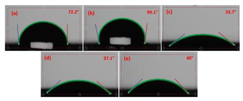
Fig. 8 Contact angle measurements for (a) IHSC, (b) IHSC-900, (c) Ce-IHSC-700, (d) Ce-IHSC-800, and (e) Ce-IHSC-900.
