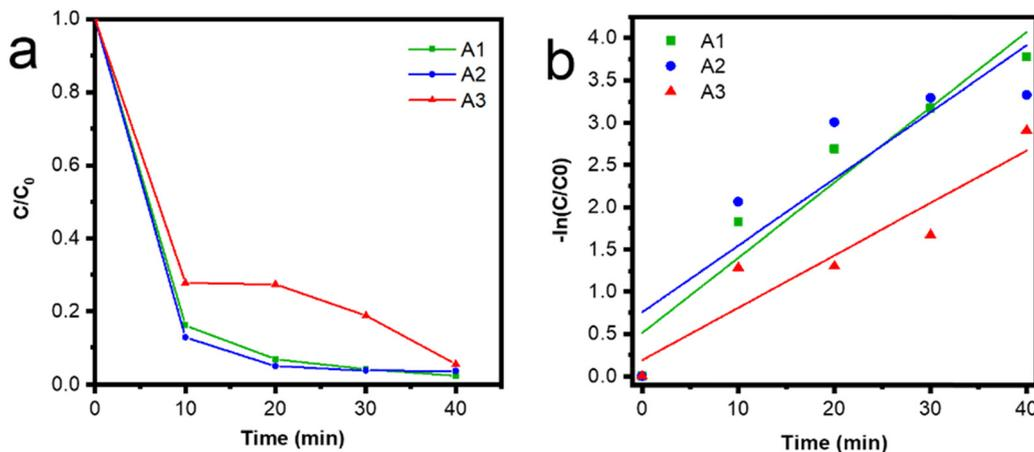
Fig. 9 (a) Photodegradation efficiency of samples and (b) first-order kinetics of MB dye in 40 min under irradiation of UV light.
