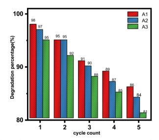
Fig. 11 Cyclic stability and reusability of the photocatalyst for A1, A2, and A3 samples in five cycles.
