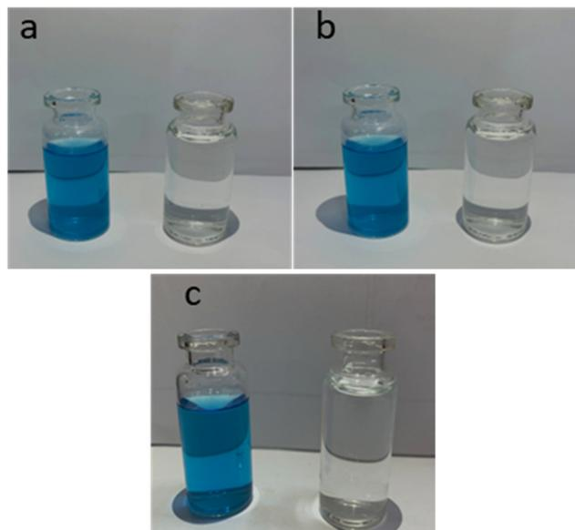
Fig. 10 Degradation of MB dye after 40 min UV light irradiation in presence of (a) A1, (b) A2 and (c) A3 photocatalysts.
