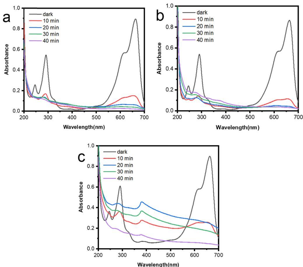
Fig. 8 UV-vis spectra of MB dye during photodegradation in presence of (a) A1 (b) A2 (c) A3 photocatalysts.
