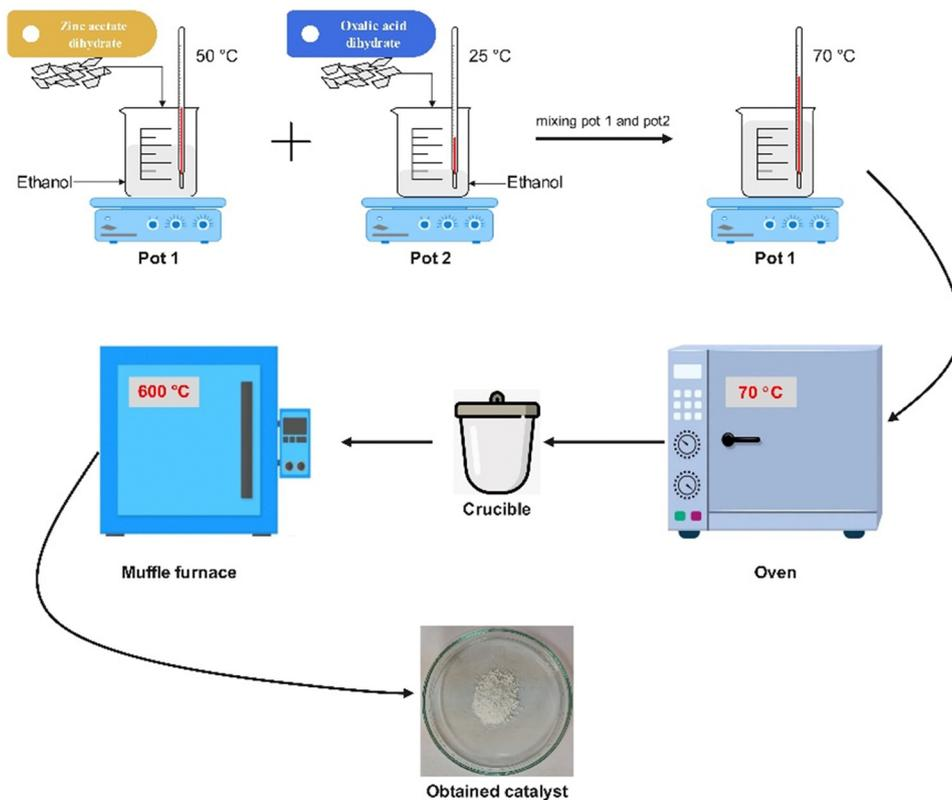
Fig. 1 Schematic of synthesizing process of ZnO photocatalyst.
