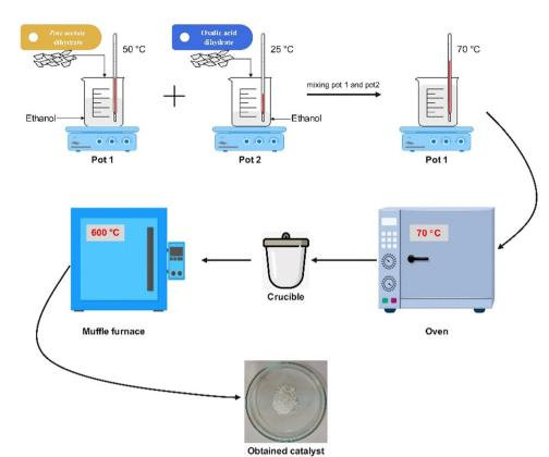
Fig. 1 Schematic of synthesizing process of ZnO photocatalyst.
