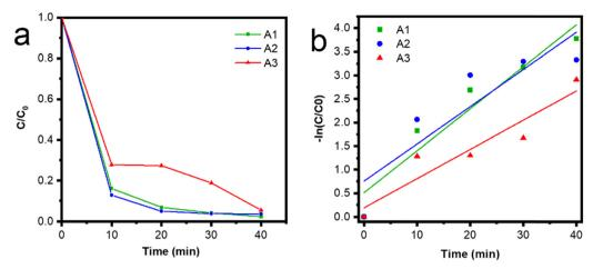
(a) Photodegradation efficiency of samples and (b) first-order kinetics of MB dye in 40 min under irradiation of UV light.
