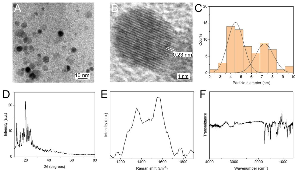
**Fig. 1** Characterization of the synthesized CDs. (A) TEM image of the CDs. (B) HR-TEM images of the CDs with lattice spacings. (C) Size distribution of the CDs. (D) XRD pattern of the CDs. (E) Raman spectrum of the CDs. (F) FTIR spectrum of the CDs dispersed in ethanol.
