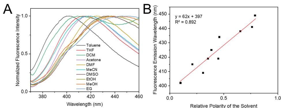
**Fig. 4** Response of the fluorescence emission of the CDs in different organic solvents. (A) Normalized blue emissions of the CDs in the different solvents under excitation of 340 nm. (B) The linear relation between the blue emission peak wavelength and the relative polarity of the solvent.
