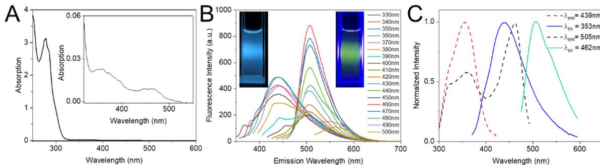
**Fig. 3** Optical properties of the CDs dispersed in ethanol. (A) Absorption spectra of the CDs in ethanol, inset shows the absorption peaks in the range of 320–550 nm. (B) The fluorescence spectra of the CDs at different excitation wavelengths showing dual emissions. Inset: Photos of CDs showing blue and green emissions under different LED lamps. (C) Normalized emission spectra (solid line) and corresponding excitation spectra (dotted line).
