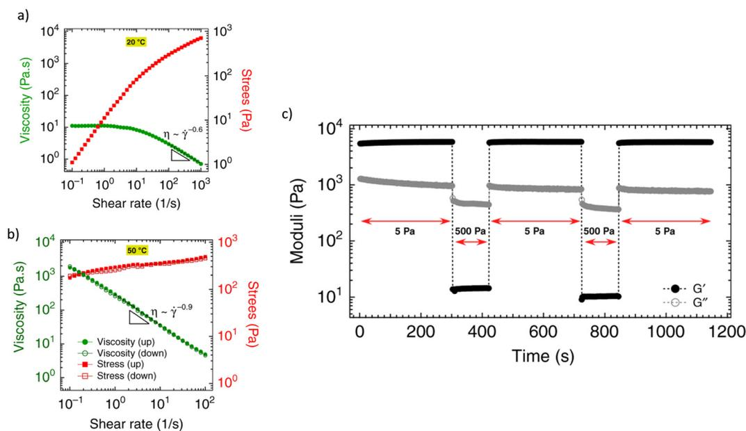
**Fig. 8** Yield stress with total recovery: (a) pseudoplasticity of a thermogelling nanoemulsion below 20 °C (sol state), (b) time-independent plastic behaviour ( $n \sim 0$ ) (gel state) above 50 °C, and, (c) total recovery of the moduli. Data reprinted with permission from ref. 114. Copyright © 2019 *Nature Comm.*
