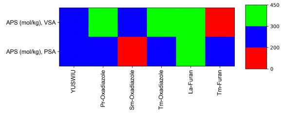
Fig. 7 APS of promising Ln-MOF candidates at VSA and PSA conditions. Geometries were optimized at QM-level and PACMOF charges were assigned Data provided for YUSWIU were taken from the calculations performed for the PACMOF-assigned crystal structure.
