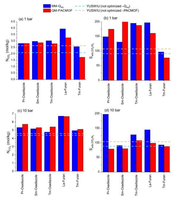
Fig. 5 Calculated CO<sub>2</sub> uptakes and  $S_{ads,CO_2/N_2}$  at 1 bar (a) and (b), and at 10 bar (c) and (d) for original YUSWIU and YUSWIU-derived hypothetical MOFs.
