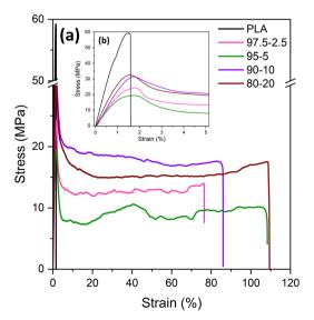
Fig. 12 (a) Tensile stress—strain curves of PLA and PLA-*b*-PEAz copolyesters and (b) zoom area at low strain values.
