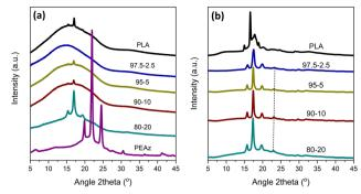
Fig. 7 XRD patterns of PLA, PEAz and their copolymers (a) using asreceived compression molded samples and (b) after annealing of the compression molded samples at  $T_{\rm cc}$  (onset) – 10 °C for 1 h.
