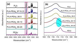
Fig. 2 ATR-FTIR spectra of (a) PLA, PEAz, and their copolymers, and (b) zoom at carbonyl's region.
