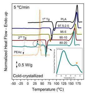
Fig. 5 DSC traces during heating of quenched samples at 5 °C min<sup>-1</sup>.
