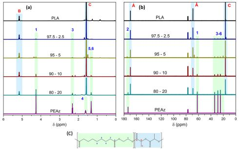
Fig. 3 (a) <sup>1</sup>H NMR, (b) <sup>13</sup>C NMR spectra of the synthesized homopolyesters and copolyesters, and (c) the corresponding signal assignments.
