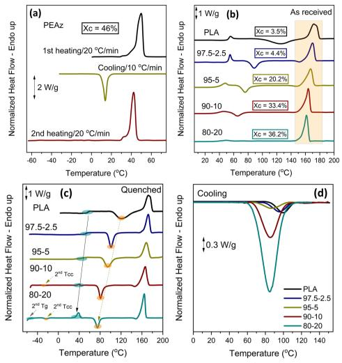
Fig. 4 (a) DSC traces of PEAz, and (b) PLA and PLA-b-PEAz copolyesters during heating at 20 °C min<sup>-1</sup> of as-received compression molded samples, (c) during heating at 20 °C min<sup>-1</sup> of guenched samples, and (d), during cooling at 10 °C min<sup>-1</sup>.
