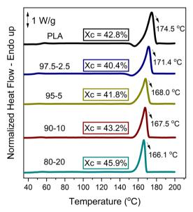
Fig. 6 DSC traces of the materials after annealing at  $T_{\rm cc}$  (onset) – 10 °C for 1 h for the compression molded samples. The DSC traces were recorded during the heating rate of 20 °C min<sup>-1</sup>.
