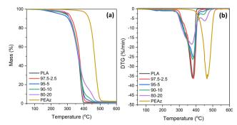
Fig. 11 (a) TGA curves of PLA, PEAz and their copolymers at 20  $^{\circ}$ C min $^{-1}$  in inert atmosphere, and (b) derivative TG curves of PLA, PEAz and their copolymers.
