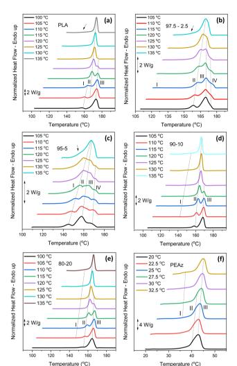
Fig. 9 Subsequent heating at 20 °C min<sup>-1</sup> after isothermal melt crystallization at the corresponding temperatures of (a) PLA, PLA-b-PEAz copolyesters, (b), 97.5-2.5, (c) 95-5, (d) 90-10, (e) 80-20, and (f) PEAz.
