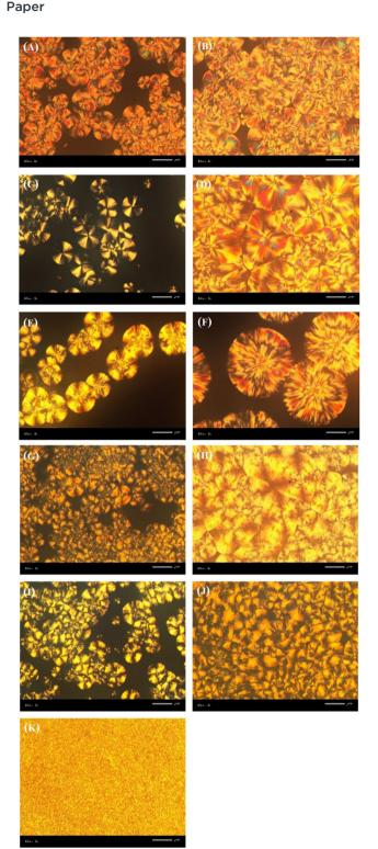
Fig. 10 PLM observations under isothermal melt crystallization of (a) and (b) PLA, (c) and (d) PLA-b-PEAz\_97.5-2.5 copolyester, (e) and (f) PLA-b-PEAz\_95-5 copolyester, (g) and (h) PLA-b-PEAz\_90-10 copolyester, (i) and (j) PLA-b-PEAz\_80-20 copolyester at 115 °C and (k) PEAz at 30 °C. The scale bar was set at 500  $\mu m$ .
