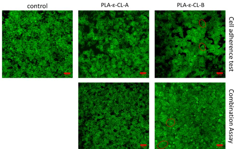
**Fig. 5** Representative images of microscopic evaluation of TR146 cells on PLA- $\epsilon$ -CL specimens (control) and PLA- $\epsilon$ -CL-A/B specimens with immobilized PHMB without and after previous bacterial contamination, using actin filament staining. Scale bar 50  $\mu$ m.
