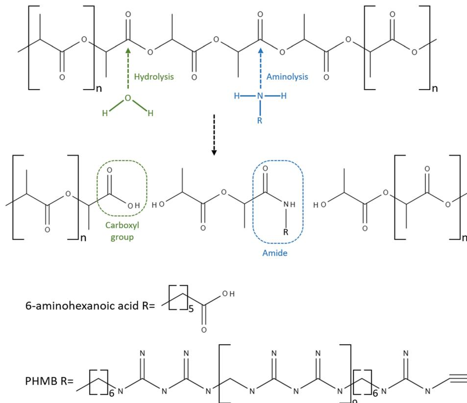
Fig. 3 Reaction of PHMB with the PLA- $\epsilon$ -CL surface when using procedure A or B. Using procedure A, carboxylic groups after hydrolysis enable PHMB immobilization, whereas using procedure B, PHMB is tethered via an amide group to the PLA- $\epsilon$ -CL surface after aminolysis.
