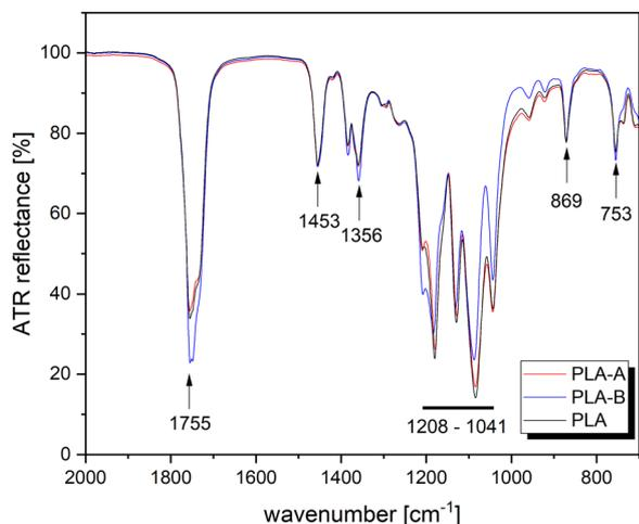
Fig. 4 Characteristic ATR-FTIR spectra in the fingerprint region: reference sample PLA- $\epsilon$ -CL (PLA) and PLA- $\epsilon$ -CL coated with PHMB using procedures A and B (PLA-A and PLA-B, respectively).
