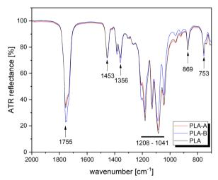
**Fig. 4** Characteristic ATR-FTIR spectra in the fingerprint region: reference sample PLA-ε-CL (PLA) and PLA-ε-CL coated with PHMB using procedures A and B (PLA-A and PLA-B, respectively).
