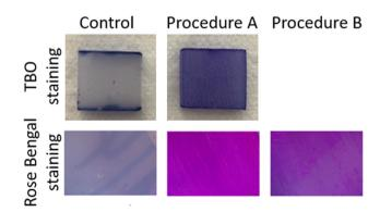
Fig. 2 Representative image of staining anionic groups after the hydrolysis of test specimens in NaOH/EtOH (top row) and of staining specimens after procedure A and B with Rose Bengal for the quantification of immobilized PHMB (bottom row).
