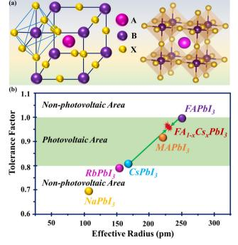
Fig. 5 (a) Basic formation of ABX<sub>3</sub> with corner-sharing BX<sub>6</sub> octahedra. (b) The role of the Goldschmidt tolerance factor in performance.
