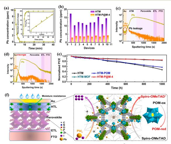
Fig. 13 (a) Absorption of lead ions on P@M-4. The two inserted figures show the quantity of absorbed Pb<sup>2+</sup> and the pseudo-first-order kinetic model. (b) Pb concentration in contaminated water, detected by ICP-OES. TOF-SIMS depth profiles of PSCs with (c) pristine HTL and (d) HTL-P@M-4. (e) Stability test of the unencapsulated devices in 40% RH and 25 °C. (f) A schematic diagram of the impact of P@M on the performance of the devices. Reproduced with permission from ref. 195
