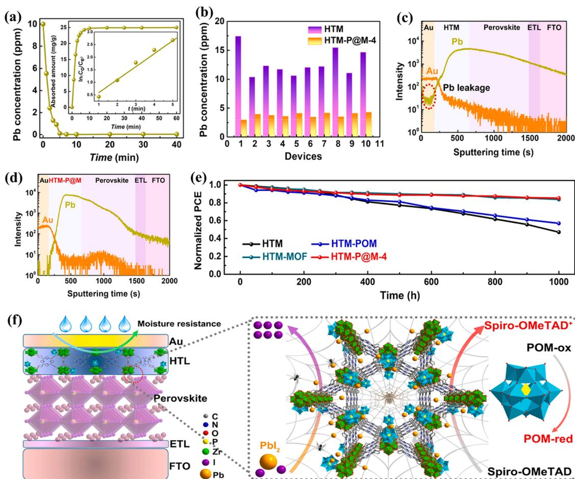
**Fig. 13** (a) Absorption of lead ions on P@M-4. The two inserted figures show the quantity of absorbed  $\text{Pb}^{2+}$  and the pseudo-first-order kinetic model. (b) Pb concentration in contaminated water, detected by ICP-OES. TOF-SIMS depth profiles of PSCs with (c) pristine HTL and (d) HTM-P@M-4. (e) Stability test of the unencapsulated devices in 40% RH and 25 °C. (f) A schematic diagram of the impact of P@M on the performance of the devices. Reproduced with permission from ref. 195.
