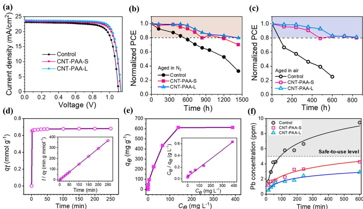
**Fig. 10** (a) Photovoltaic performance curves of the best PSCs. Stability test in (b) glovebox and (c) ambient air of the PSCs with and without CNT-PAA. (d) Adsorption of lead by CNT-PAA (inset: Lagergren second-order fitting model) and (e) isotherm adsorption of lead by CNT-PAA (inset: Langmuir adsorption fitting model) and (f) lead concentration after the immersion of the devices in water. Reproduced with permission from ref. 203.
