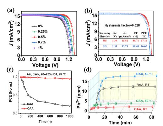
Fig. 12 (a) I-V characteristics of PSCs with different concentrations of BP-9 additives. (b) I-V hysteresis. (c) Stability test at 25 °C in ambient air with 20-25% RH with BP-9(OAA) and pristine device (RAA). (d) Pb<sup>2+</sup> leakage test into deionized water at room temperature and 50 °C of the additive-induced device and pristine device. Reproduced with permission from ref. 206
