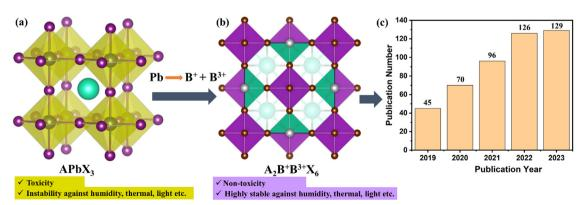
Fig. 8 (a) and (b) Comparison between lead-based and lead-free HDP materials: the transition from toxic, unstable, lead-based PVSKs to non-toxic, stable, lead-free double halide alternatives. (c) The increasing research interest in lead-free HDPs is highlighted by the growing number of publications from 2019 to 2023.
