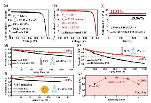
Fig. 18 (a) and (b) J-V characteristics of fresh and recycled PSC. (c) SPO values measured at MPP for both fresh and recycled PSC. Stability of the unencapsulated fresh and recycled PSC (d) under air atmosphere for 1200 h (RH = 60-80%), (e) under nitrogen atmosphere at 85 °C for 1200 h and (f) under one-sun illumination in air and MPP tracking. (g) Cycling stability of the regenerated PSC. Reproduced with permission from ref. 201.
