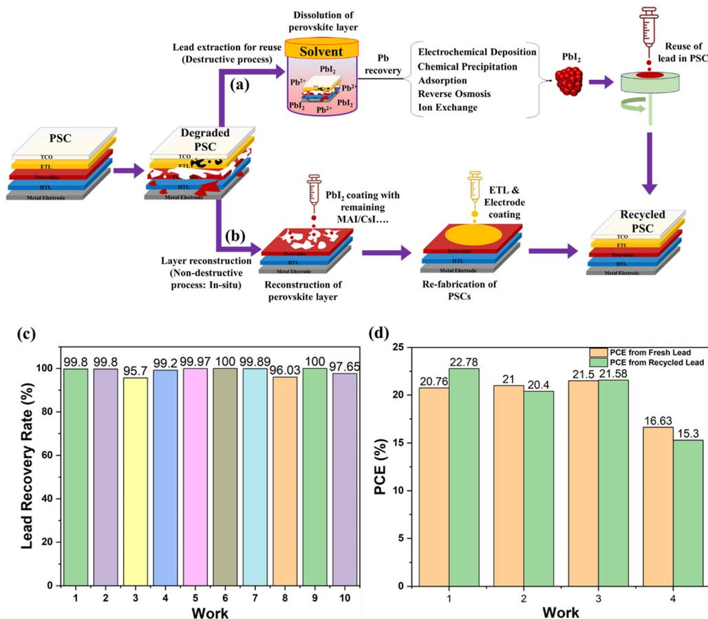
Fig. 17 (a) Extraction of lead and reuse in a PSC. (b) Reconstruction of PVSK layer and other layers. (c) Percentage of lead recovery using various tactics.<sup>225–234</sup> (d) Comparison of recycled lead-based PSCs with fresh lead-based PSCs.<sup>235–238</sup>
