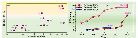
Fig. 2 Attempt to produce eco-friendly PSCs. (a) Comparing the toxicity of various metals; redrawn with permission from ref. 42. (b) The progression in efficiency of lead-free PSCs.
