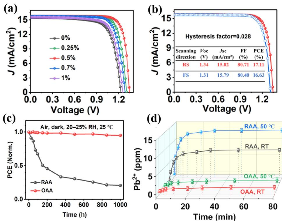
Fig. 12 (a)  $I$ - $V$  characteristics of PSCs with different concentrations of BP-9 additives. (b)  $I$ - $V$  hysteresis. (c) Stability test at 25 °C in ambient air with 20–25% RH with BP-9(OAA) and pristine device (RAA). (d)  $\text{Pb}^{2+}$  leakage test into deionized water at room temperature and 50 °C of the additive-induced device and pristine device. Reproduced with permission from ref. 206.
