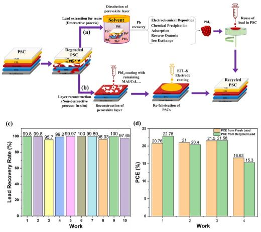
Fig. 17 (a) Extraction of lead and reuse in a PSC. (b) Reconstruction of PVSK layer and other layers. (c) Percentage of lead recovery using various tactics.<sup>225–234</sup> (d) Comparison of recycled lead-based PSCs with fresh lead-based PSCs.<sup>235–238</sup>
