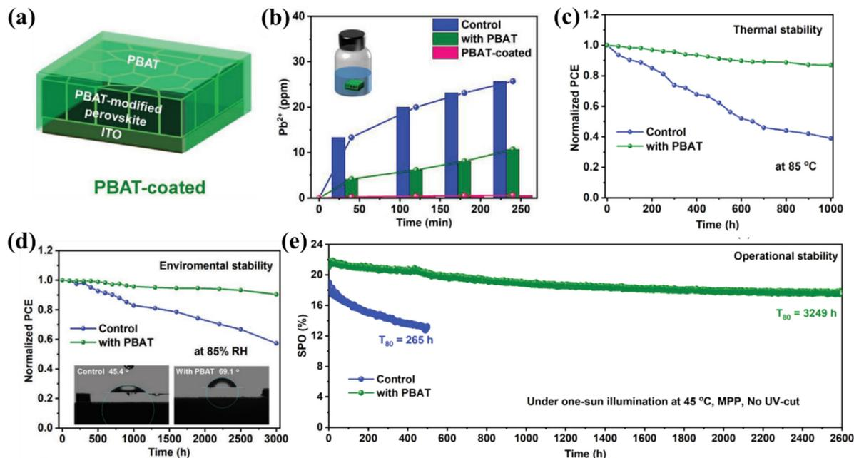
**Fig. 9** (a) Schematic illustration of PVSK film coated with a PBAT. (b) Concentration of leaked Pb after 240 minutes of immersion of pristine, PBAT-incorporated, and PBAT-coated PVSK films in water. (c) Thermal stability test in nitrogen at 85 °C of the PSCs without encapsulation. (d) Moisture stability test of the PSCs under 85% RH. (e) Operational stability of encapsulated PSCs with and without PBAT under one sun at 45 °C with MPP tracking in air. Reproduced with permission from ref. 191.
