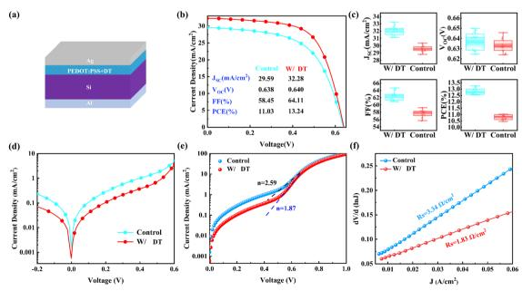
Fig. 4 (a) Schematic of the devices with DT. (b) J-V curves under 100 mW cm<sup>-2</sup> illumination (AM 1.5), (c) statistical plots of the photovoltaic performance and (d) dark J-V curves of the devices with or without DT. (e) Linear fitting and (f)  $dV/d(\ln J)-J$  curves calculated from the dark J-V curves of the devices with and without DT.
