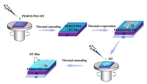
Fig. 1 Schematic of the fabrication process for colored devices.
