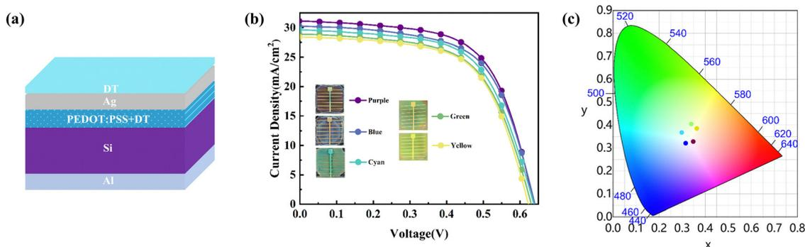
Fig. 5 (a) Schematic of the colored devices. (b)  $J$ - $V$  curves of the colorful devices under  $100 \text{ mW cm}^{-2}$  illumination (AM 1.5). (c) Coordinates of the colored devices in the CIE 1931 chromaticity diagram.
