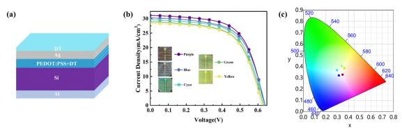
Fig. 5 (a) Schematic of the colored devices. (b) J-V curves of the colorful devices under 100 mW cm<sup>-2</sup> illumination (AM 1.5). (c) Coordinates of the colored devices in the CIE 1931 chromaticity diagram.
