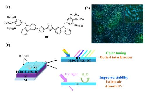
Fig. 2 (a) Chemical structure of DT. (b) Image of DT obtained by polarized optical microscopy. (c) Schematic of the two functions of the DT coating for colorful and stable devices.
