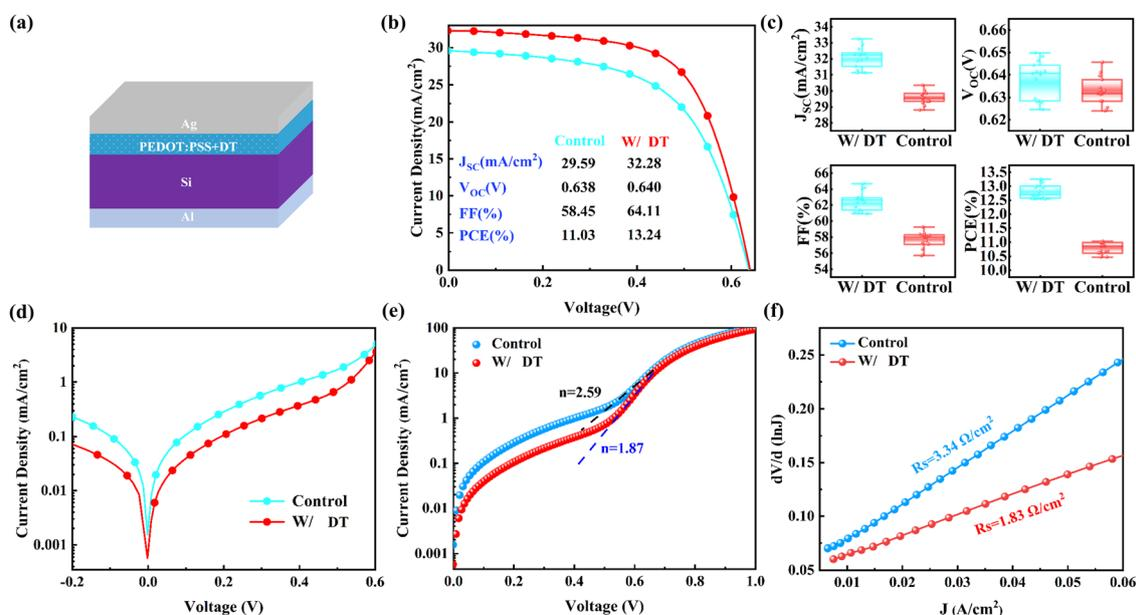
Fig. 4 (a) Schematic of the devices with DT. (b)  $J$ - $V$  curves under  $100 \text{ mW cm}^{-2}$  illumination (AM 1.5), (c) statistical plots of the photovoltaic performance and (d) dark  $J$ - $V$  curves of the devices with or without DT. (e) Linear fitting and (f)  $dV/d(\ln J)$ - $J$  curves calculated from the dark  $J$ - $V$  curves of the devices with and without DT.
