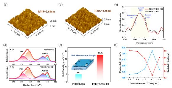
Fig. 3 Root mean square roughness images of (a) PEDOT:PSS films and (b) PEDOT:PSS + DT films. (c) Normalized Raman spectra, (d) XPS spectra in the S 2p region and (e) Hall mobility obtained from Hall measurements of PEDOT:PSS and PEDOT:PSS + DT films. (f) Conductivity and resistivity of PEDOT:PSS films with the addition of different concentrations of DT solution.
