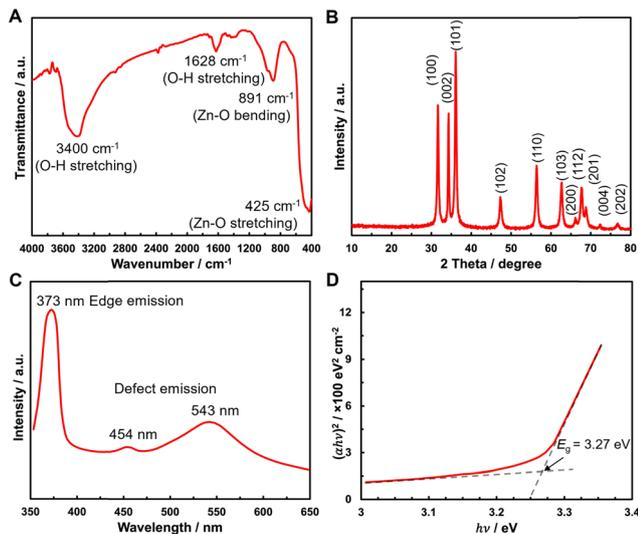
**Fig. 1** Structural and optical characterization of ZnO. (A) FTIR spectrum showing the functional groups present. (B) XRD pattern with labeled peaks corresponding to specific crystalline planes. (C) PL spectrum indicating the optical emission properties. (D) Tauc plot showing the optical bandgap energy derived from UV-Vis absorption data. The dotted lines in the Tauc plot indicate the base (horizontal) and fitted (vertical) lines. a.u. on the Y-axes indicates arbitrary units.
