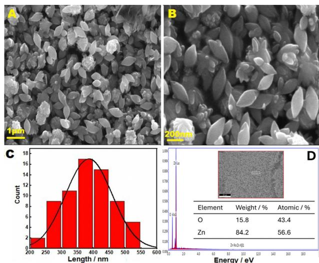
**Fig. 2** Morphological and compositional analysis of ZnO. (A) and (B) SEM images at two different magnifications. (C) Particle size distribution histogram derived from the SEM image (B), with a Gaussian fit shown as a black curve. (D) EDS spectrum, with the inset showing the full area analyzed (upper) and the elemental composition (lower).
