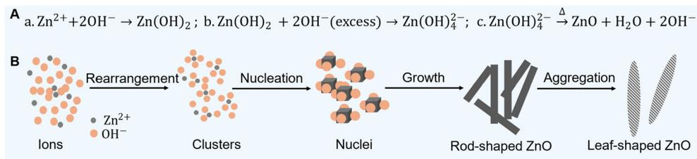
**Scheme 2** Reactions and mechanisms in ZnO formation. (A) Possible reactions involved in the synthesis of ZnO. (B) Proposed mechanism for the formation of ZnO leaf structures.
