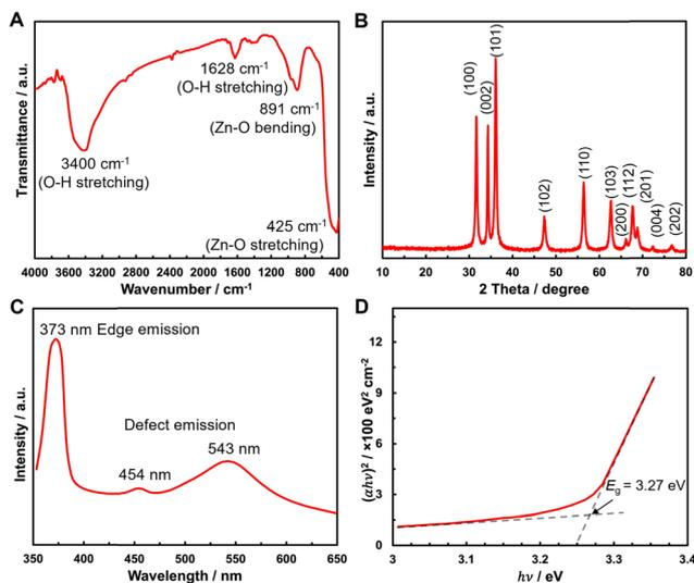
**Fig. 1** Structural and optical characterization of ZnO. (A) FTIR spectrum showing the functional groups present. (B) XRD pattern with labeled peaks corresponding to specific crystalline planes. (C) PL spectrum indicating the optical emission properties. (D) Tauc plot showing the optical bandgap energy derived from UV-Vis absorption data. The dotted lines in the Tauc plot indicate the base (horizontal) and fitted (vertical) lines. a.u. on the Y-axes indicates arbitrary units.
