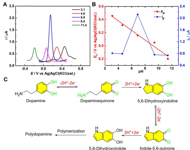
Fig. 4 pH-dependent DA oxidation at the ZnO/GC electrode in 0.1 M PBS. (A) DPVs in the presence of 50  $\mu$ M DA at different pH values. (B) Plot of peak potential ( $E_p$ ) versus pH and peak current ( $i_p$ ) versus pH derived from (A). (C) Plausible mechanism for the electrochemical oxidation of DA at the ZnO/GC electrode. The experimental parameters for DPV: potential increment = 4 mV, pulse amplitude = 50 mV, pulse width = 60 ms, and pulse period = 0.5 s.
