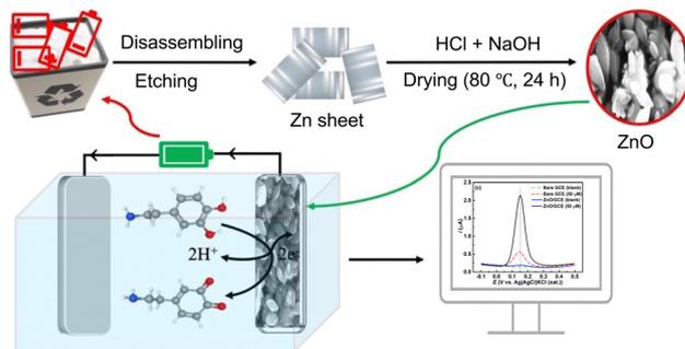
**Scheme 1** Synthesis of ZnO nanostructures and their application in DA detection. (Upper panel) Schematic representation of the synthesis of ZnO nanostructures from waste batteries. (Lower panel) Electrochemical detection of DA using the ZnO-based electrode.
