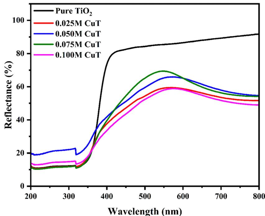
Fig. 6 UV-Vis DRS spectra of pure TiO<sub>2</sub> and different Cu-doped TiO<sub>2</sub> samples.
