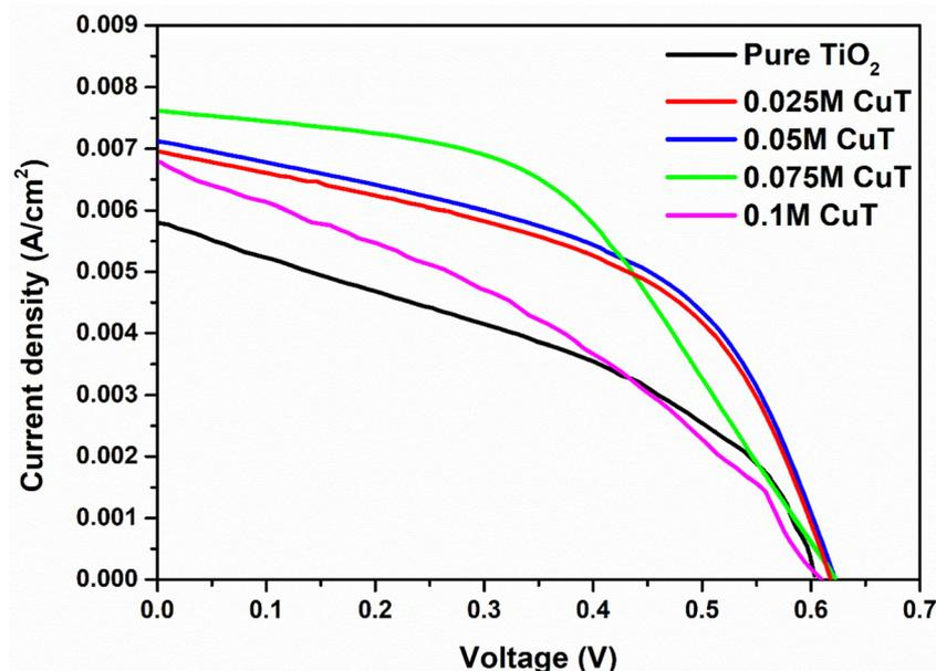
Fig. 9  $J$ - $V$  analysis of pure and various Cu-doped  $\text{TiO}_2$  DSSCs.
