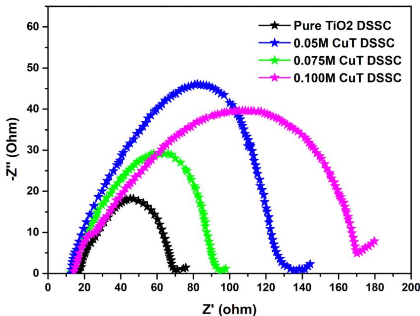
Fig. 11 EIS spectra of pure and various Cu-doped  $\text{TiO}_2$ -based DSSCs.
