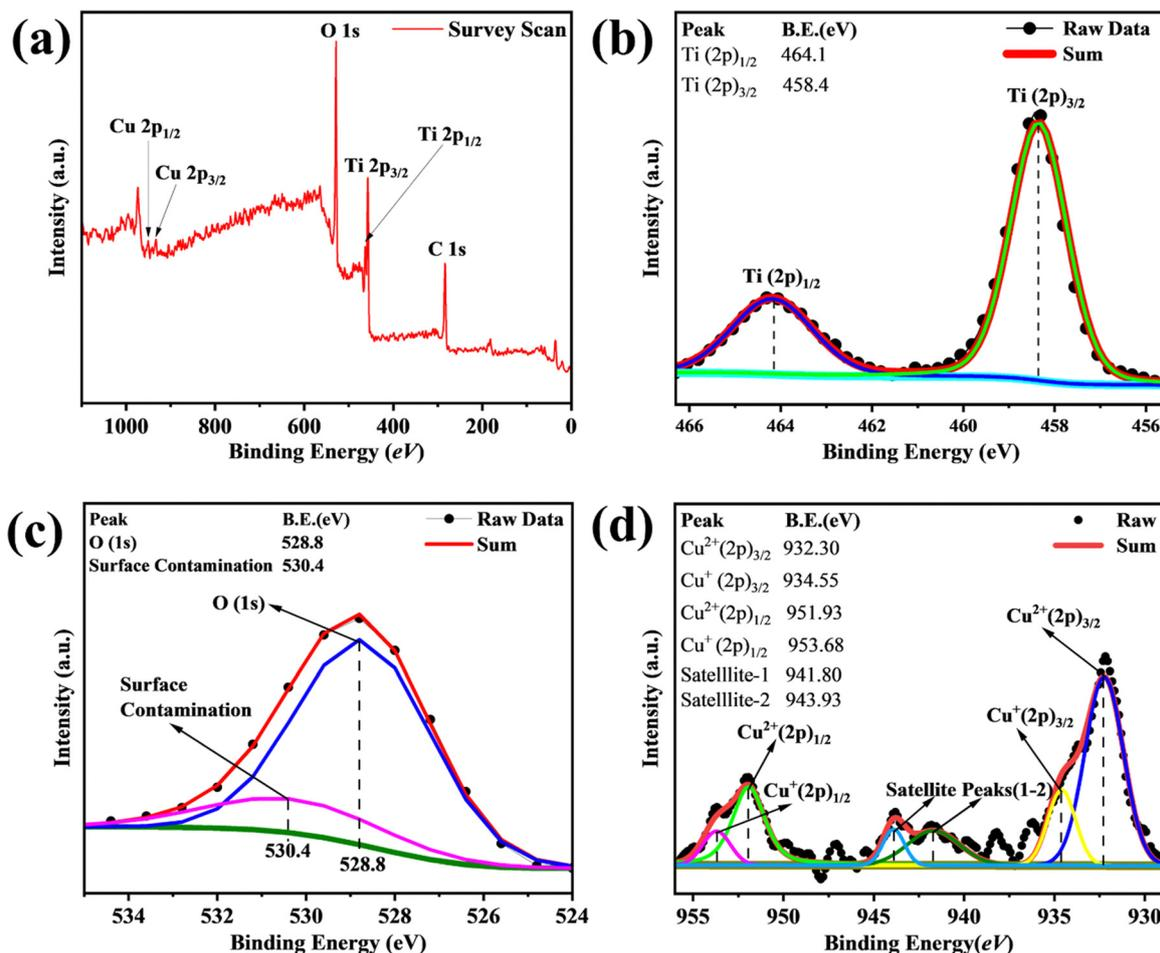
Fig. 8 (a) Survey spectrum of 0.075 M Cu-doped TiO<sub>2</sub> sample; (b) core level spectra of Ti; (c) core level spectra of O; (d) core level spectra of Cu in 0.075 M Cu-doped TiO<sub>2</sub> sample.
