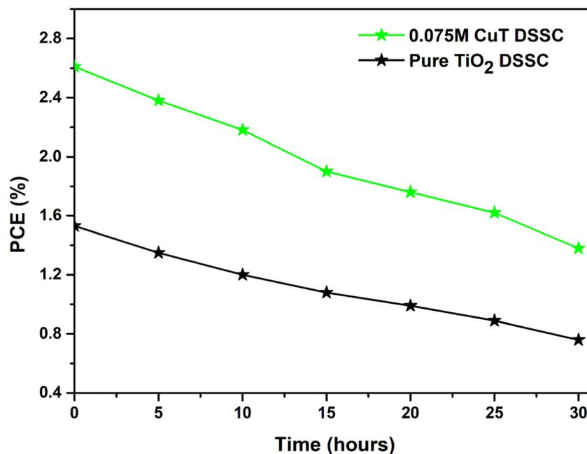
Fig. 12 Stability test graph of the pure TiO<sub>2</sub> DSSC and 0.075 M CuT DSSC.
