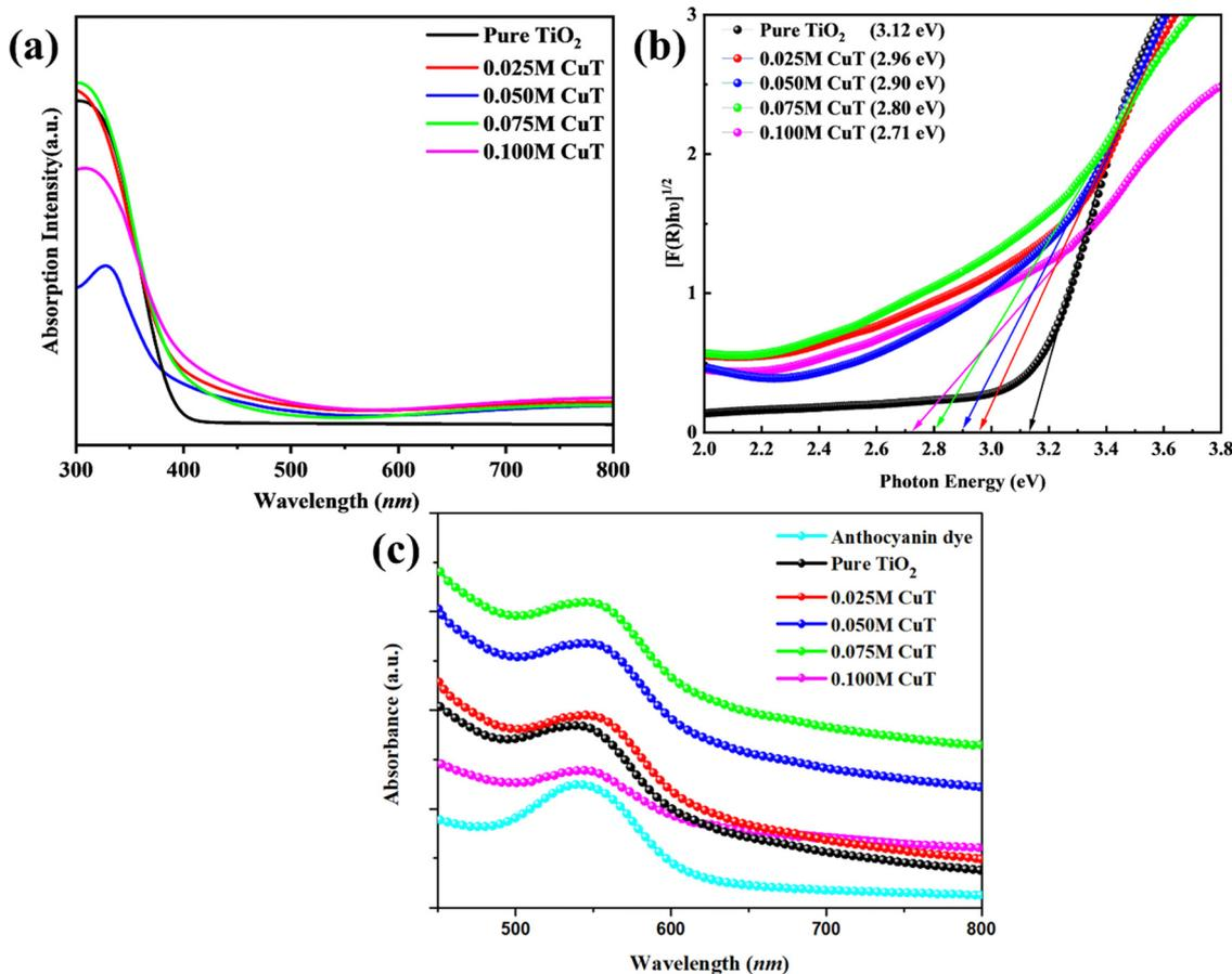
Fig. 7 (a) and (b) UV-Vis absorbance spectra and Tauc plots for undoped TiO<sub>2</sub> and different Cu-doped TiO<sub>2</sub> samples; and (c) absorbance spectra of anthocyanin sensitized various TiO<sub>2</sub> films.
