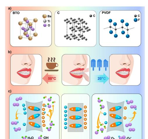
Fig. 1 Schematic illustration of the composition structure of the BCPCF and the working principle. (a) Schematic representations of the molecular structures of BTO, C and PVDF from left to right. (b) The BCPCF stimulated piezoelectric and thermal catalytic effects through mastication pressure and temperature changes. (c) BTO produced  ${}^{\bullet}\text{OH}$  and  ${}^{\bullet}\text{O}_2^-$  via piezoelectric and thermal catalytic effects.
