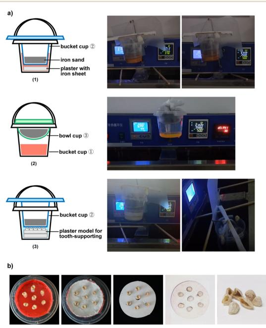
Scheme 1 ATT. 1 Equipment for whitening experiments. (a) (1) For the mechanical pressure cycle test and the mechanical pressure and cooling-heating cycle test in the RhB degradation test. (2) For the cooling-heating cycle test in the RhB degradation test. (3) For the mechanical pressure and coolingheating cycle test in the dental whitening experiment. (b) The preparation of the plaster model for tooth-support and the image of the BCPCF.
