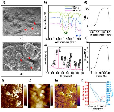
Fig. 2 The characterization of the BCPCF. (a) SEM image of the BCPCF. (1) and (2) indicate the C particles and the BTO particles, respectively. (b) FT-IR image of the PF, the BCPCF and the BPCF. (c) X-ray image of the BCPCF. (d) and (e) indicate the tensile strength and the elasticity modulus of the BCPCF respectively. (f)-(i) indicate the amplitude, the height-line, the phase, and the local piezoelectric hysteresis loop image of the BCPCF. Data are means  $\pm$ SD(n = 3)
