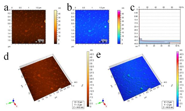
(a) and (b) 2D AFM images, (c) average height and (d) and (e) 3D AFM images of Pd/r-TiO<sub>2</sub> catalysts.
