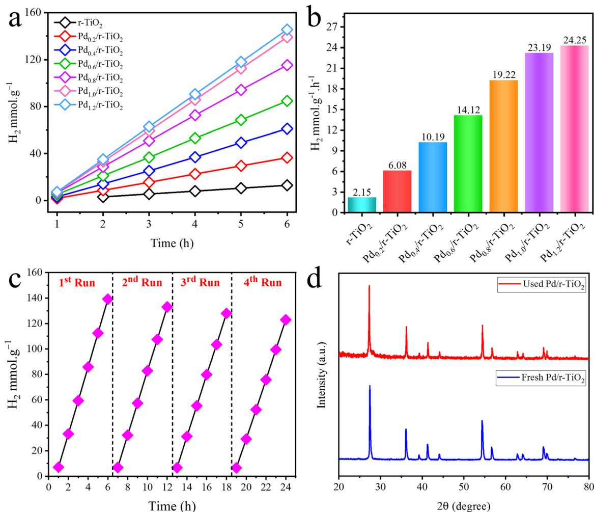
Fig. 7 (a) and (b) H<sub>2</sub> generation activities of catalysts, (c) recyclability test and (d) XRD analysis of used catalysts.
