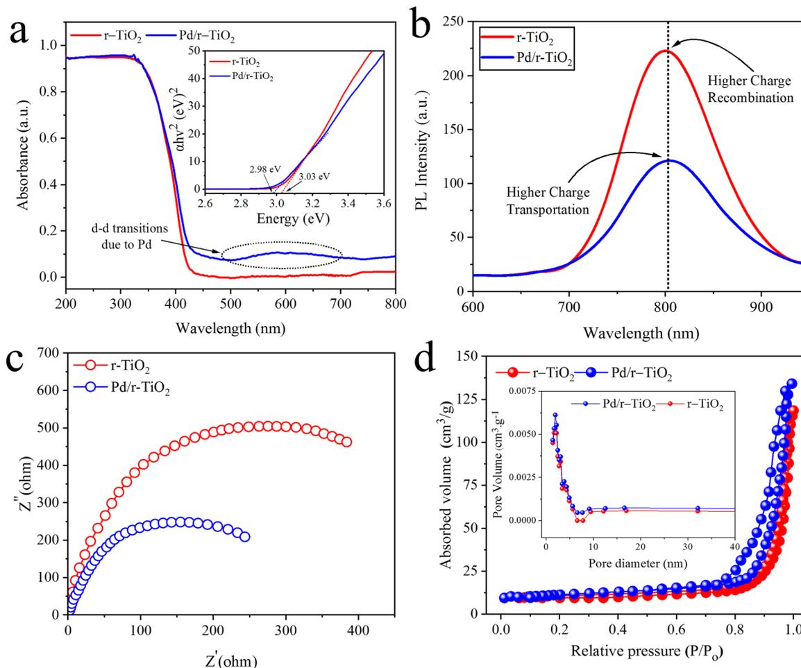
Fig. 5 (a) UV-Vis/DRS results, inset: band gap energy diagrams, (b) PL results, (c) EIS analysis, and (d) BET analysis, inset: pore volume/size distribution of r-TiO<sub>2</sub> and Pd/r-TiO<sub>2</sub>.
