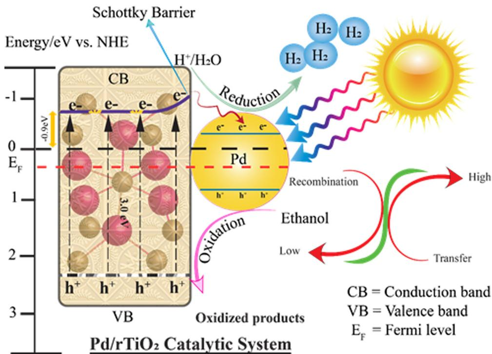
Fig. 9 Mechanism of the water splitting reaction for H<sub>2</sub> generation.
