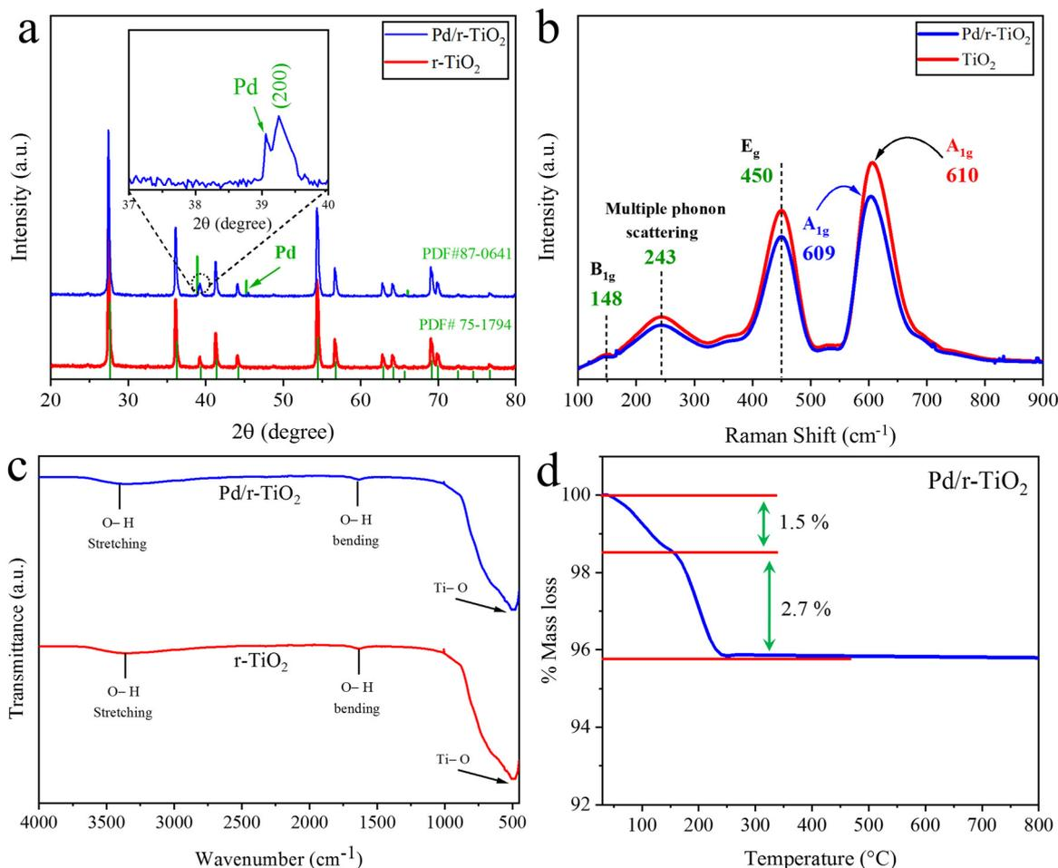
Fig. 2 (a) XRD patterns (inset: zoomed view of Pd diffraction), (b) Raman spectrum, (c) FTIR results *r*-TiO<sub>2</sub> and Pd/*r*-TiO<sub>2</sub> and (d) TGA analysis of Pd/*r*-TiO<sub>2</sub>.
