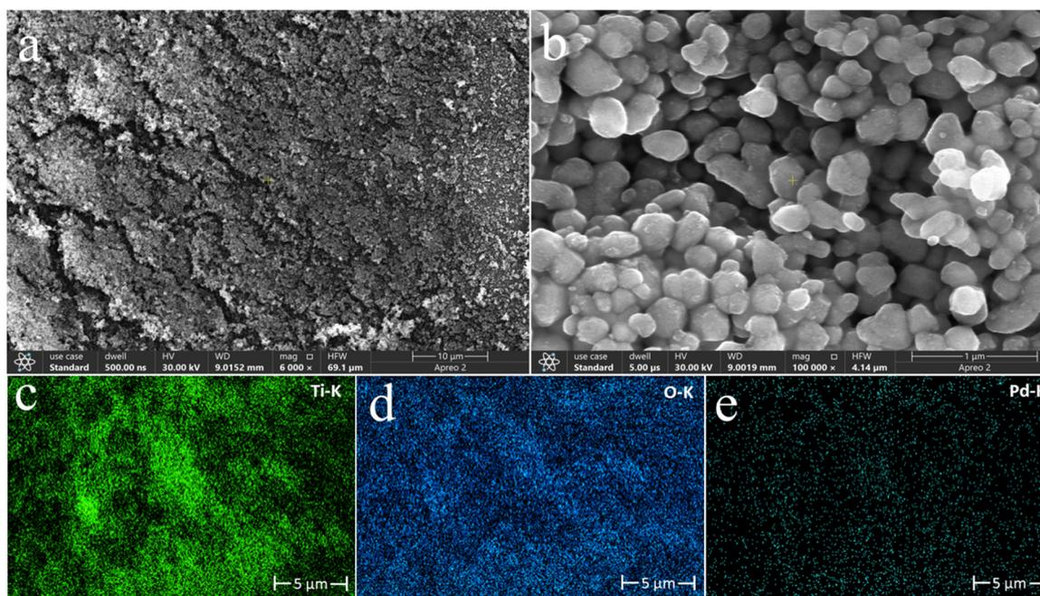
Fig. 8 SEM results of the used Pd/r-TiO<sub>2</sub> catalysts, (a)  $10 \mu\text{m}$ , (b)  $1 \mu\text{m}$ , elementals maps (c) Ti-K (d) O-K and (e) Pd-K.
