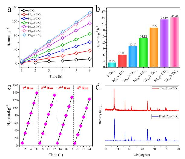
(a) and (b) H2 generation activities of catalysts, (c) recyclability test and (d) XRD analysis of used catalysts.
