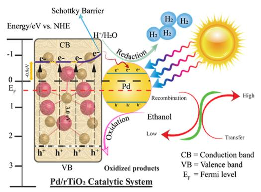
Fig. 9 Mechanism of the water splitting reaction for H<sub>2</sub> generation.
