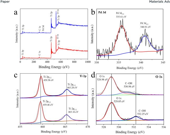
Fig. 6 (a) Survey scans XPS of Pd/r-TiO<sub>2</sub> catalysts. XPS of (b) Pd, (c) Ti and (d) oxygen (O).
