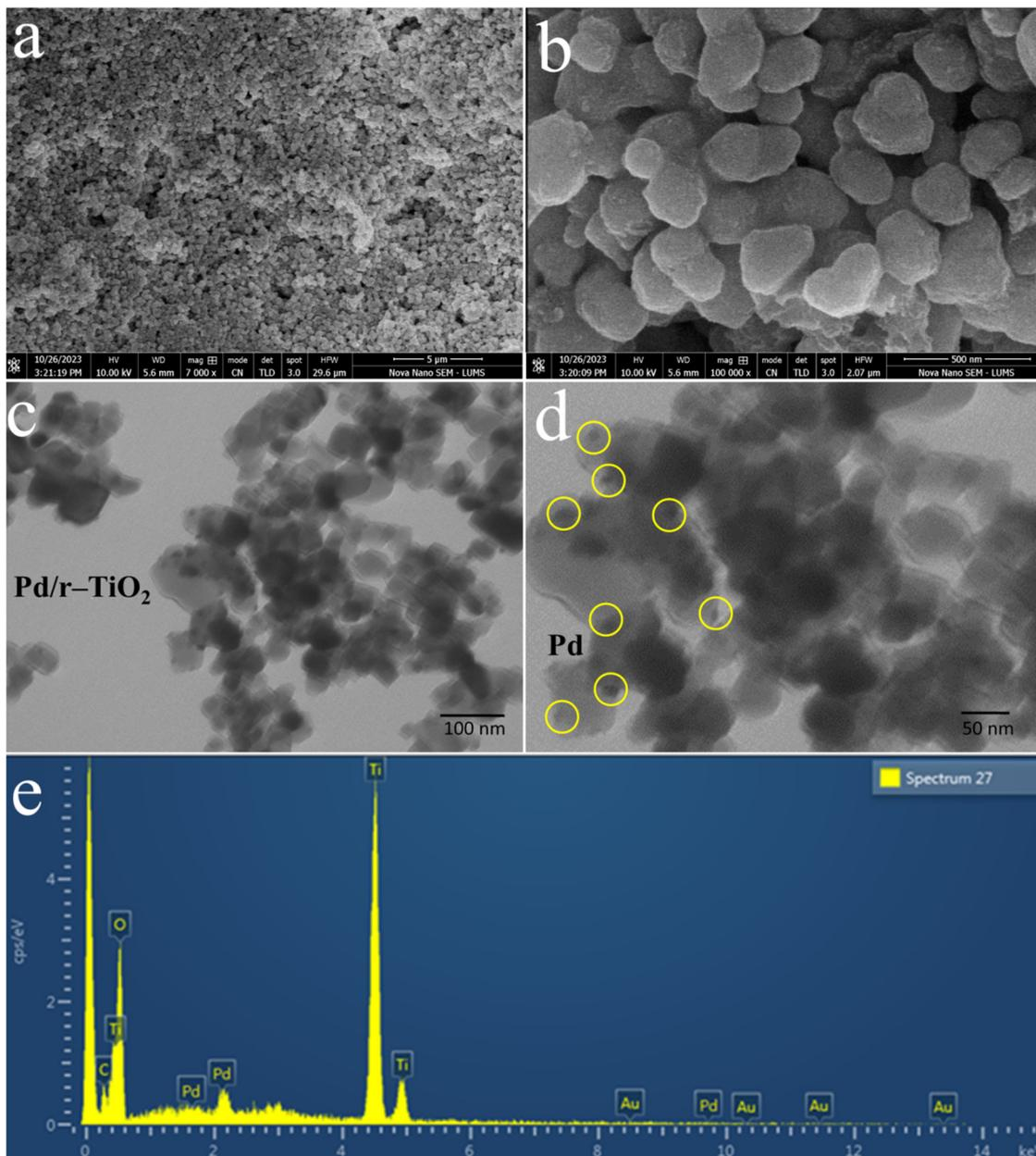
Fig. 3 SEM results (a) 5  $\mu\text{m}$  and (b) 500 nm. (c) TEM results at 100 nm and (d) 50 nm. (e) EDX of Pd/r-TiO<sub>2</sub> catalysts.
