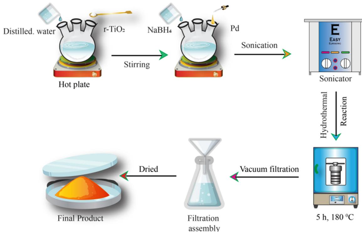
Fig. 1 Synthesis scheme for the preparation of Pd/r-TiO<sub>2</sub> catalysts.
