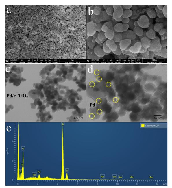
Fig. 3 SEM results (a) 5  $\mu$ m and (b) 500 nm. (c) TEM results at 100 nm and (d) 50 nm. (e) EDX of Pd/r-TiO<sub>2</sub> catalysts.
