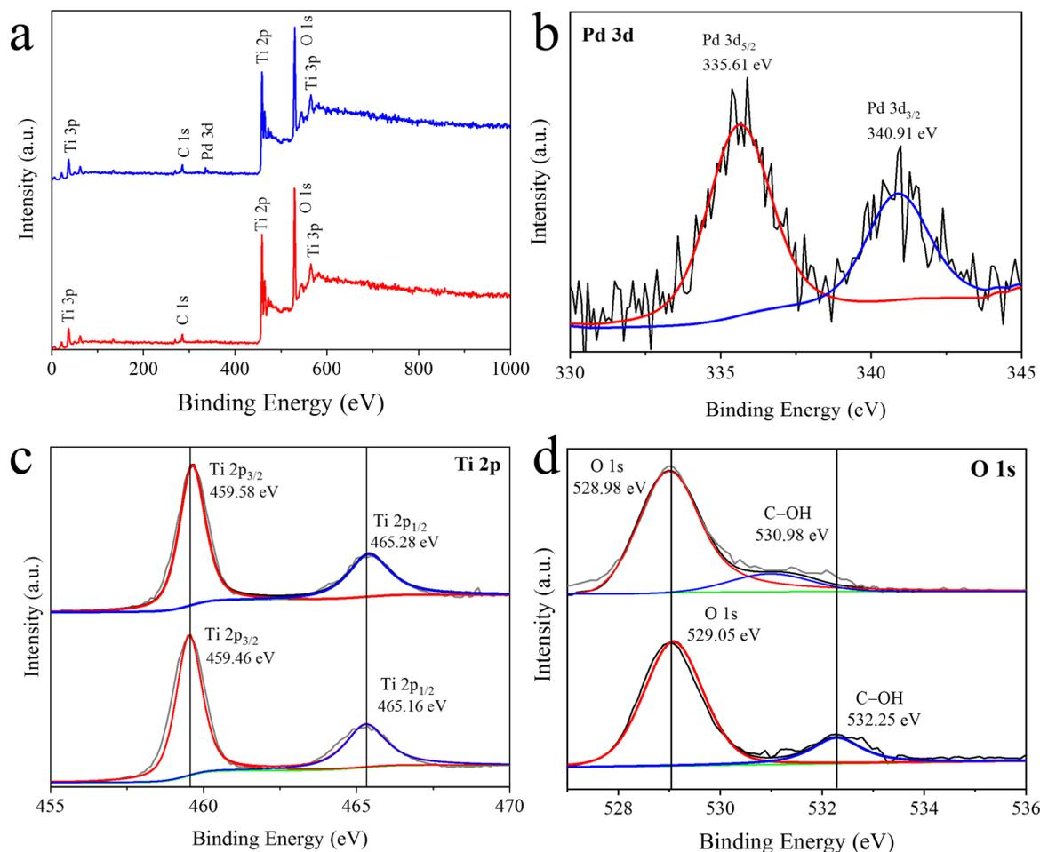
Fig. 6 (a) Survey scans XPS of Pd/r-TiO<sub>2</sub> catalysts. XPS of (b) Pd, (c) Ti and (d) oxygen (O).
