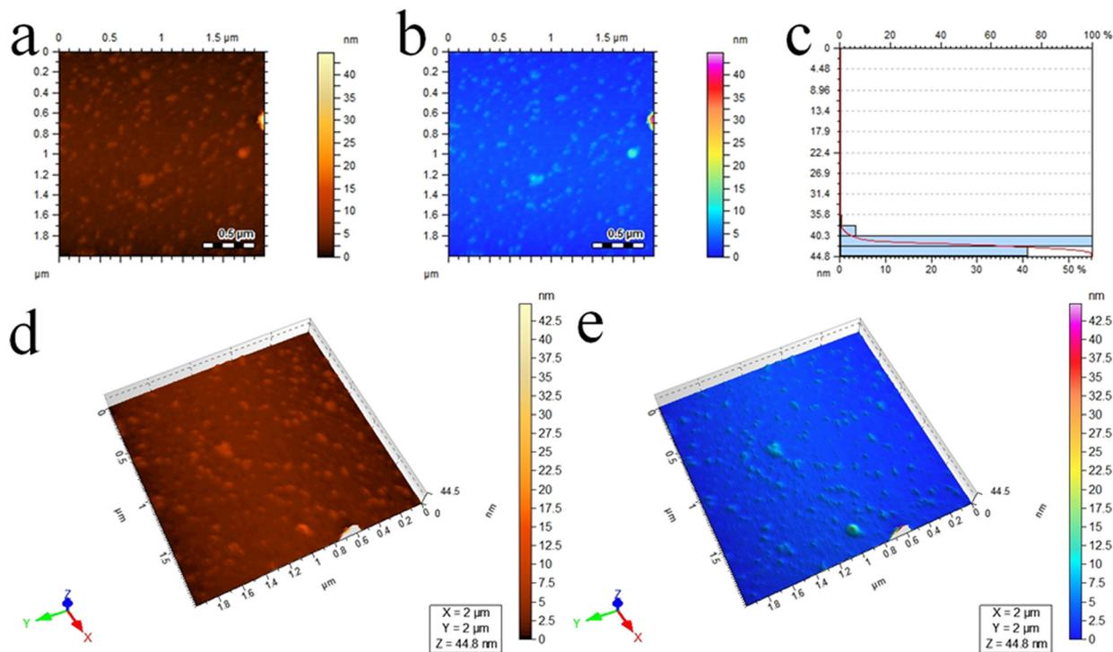
Fig. 4 (a) and (b) 2D AFM images, (c) average height and (d) and (e) 3D AFM images of Pd/r-TiO<sub>2</sub> catalysts.
