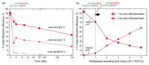
Fig. 5 (a) Retention ratio of -1st order diffraction efficiency for thin circular polarization hologram at various storage conditions. (b) Variation of ±1st order diffraction efficiency with different recording times of the second hologram for polarization hologram multiplexing.
