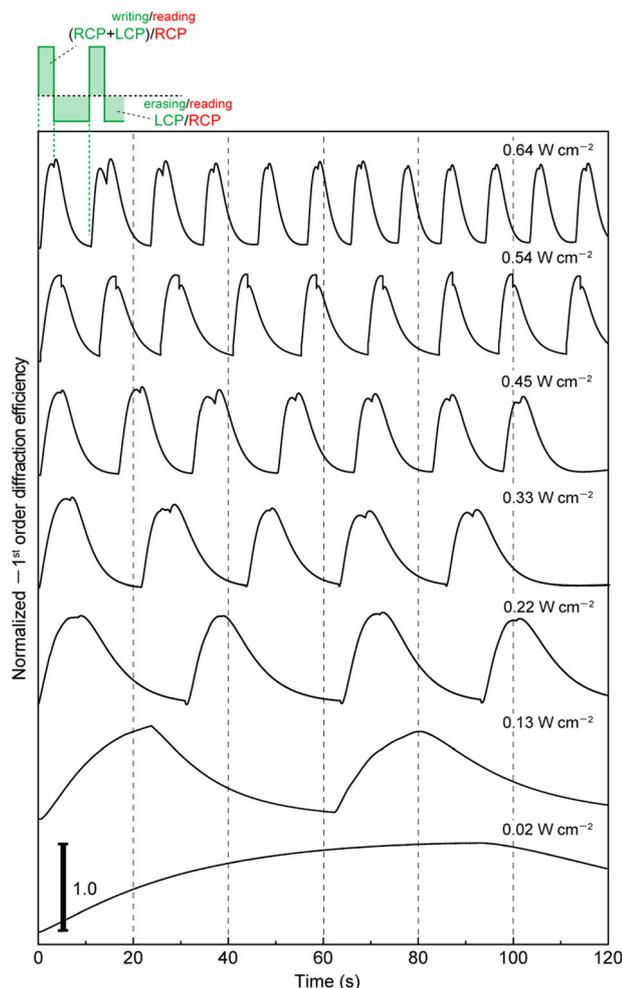
Fig. 6 Multiple cycles of writing and erasing of the thin circular polarization holograms relative to the writing beam intensity at (a)  $0.02 \text{ W cm}^{-2}$ , (b)  $0.13 \text{ W cm}^{-2}$ , (c)  $0.22 \text{ W cm}^{-2}$ , (d)  $0.33 \text{ W cm}^{-2}$ , (e)  $0.45 \text{ W cm}^{-2}$ , (f)  $0.54 \text{ W cm}^{-2}$  and (g)  $0.64 \text{ W cm}^{-2}$ .
