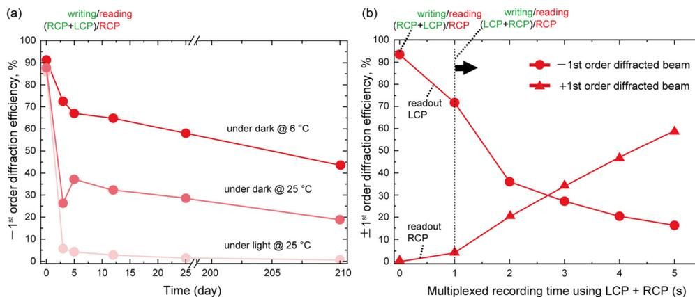
Fig. 5 (a) Retention ratio of  $-1$ st order diffraction efficiency for thin circular polarization hologram at various storage conditions. (b) Variation of  $\pm 1$ st order diffraction efficiency with different recording times of the second hologram for polarization hologram multiplexing.
