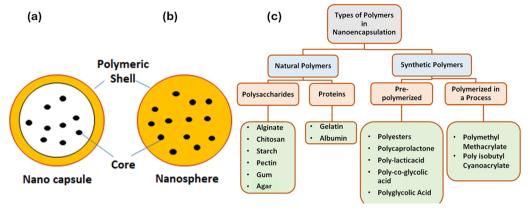
Fig. 3 Classifications of polymer nanoparticles in nanoencapsulation: (a) nanocapsules with an active material confined in a polymer shell, (b) nanospheres with an active material dispersed in a polymer matrix and (c) classification of polymers used in nanoencapsulation as natural and synthetic for encapsulating essential oils. 45,46
