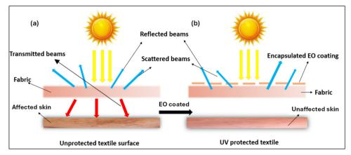
Fig. 8 (a) Pristine textile enabling the penetration of UV radiation, which reaches the skin, and (b) anti-UV finished textile impregnated with essential oil (EO)-loaded polymeric formulation, causing the transmittance of UV radiation and inhibiting it from reaching the skin
