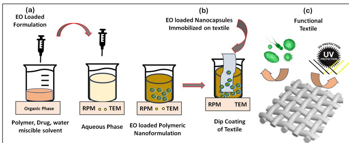
Fig. 7 (a) Synthesis of essential oil (EO)-loaded polymeric formulation *via* nanoprecipitation technique using organic and aqueous phases, (b) fabrication of EO-loaded nanocapsules on textile through dip coating and (c) functional textile showing anti-bacterial and anti-UV properties.
