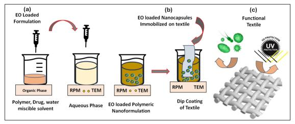
Fig. 7 (a) Synthesis of essential oil (EO)-loaded polymeric formulation via nanoprecipitation technique using organic and aqueous phases, (b) fabrication of EO-loaded nanocapsules on textile through dip coating and (c) functional textile showing anti-bacterial and anti-UV properties.
