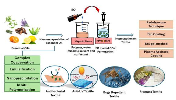
Fig. 1 Nanoencapsulation strategies for loading essential oils (EOs) in polymeric nanoparticles, showcasing the formation of oil-in-water (O/W) formulations, followed by their impregnation into multifunctional textile finishing
