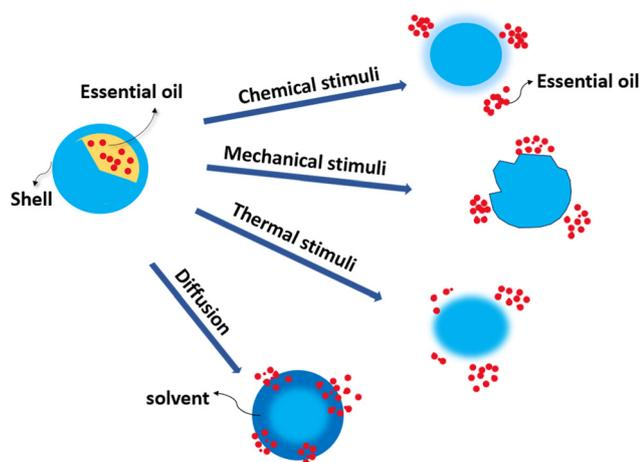
Fig. 4 Release Mechanisms of essential oils from polymeric nanocapsules.<sup>54</sup>
