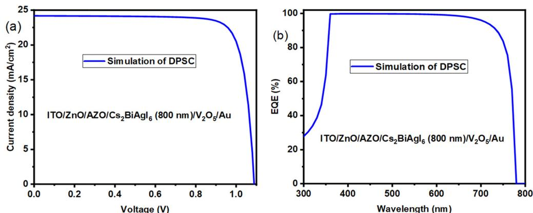
Fig. 4 (a)  $J$ – $V$  curve and (b) EQE curve for ITO/ZnO/AZO/Cs<sub>2</sub>BiAgI<sub>6</sub> (800 nm)/V<sub>2</sub>O<sub>5</sub>/Au device.
