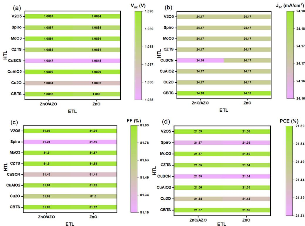
Fig. 3 Photovoltaic output parameters of (a)  $V_{oc}$  (V), (b)  $J_{sc}$  (mA cm<sup>-2</sup>), (c) FF (%), and (d) PCE (%). Contour mapping plots of the device of ITO/ETLs/Cs<sub>2</sub>BiAgI<sub>6</sub> (800 nm)/HTLs/Au for two ETLs and eight HTLs with different materials.
