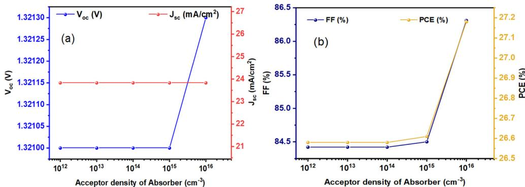
Fig. 8 (a)  $V_{oc}$  and  $J_{sc}$ , and (b) FF and PCE curves for  $\text{Cs}_2\text{BiAgI}_6$ -DPSC against acceptor density of absorber.
