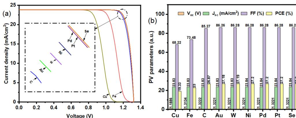
Fig. 15 (a)  $J$ - $V$  curve. Inset of the figure shows C (Carbon), Au (Gold), W (Tungsten), Ni (Nickel), Pd (Palladium), Pt (Platinum), and Se (Selenium) work functions. (b) PV parameters as a bar chart against different work functions of  $\text{Cs}_2\text{BiAgI}_6$ -DPSCs ranging from 4.65 eV to 5.9 eV.
