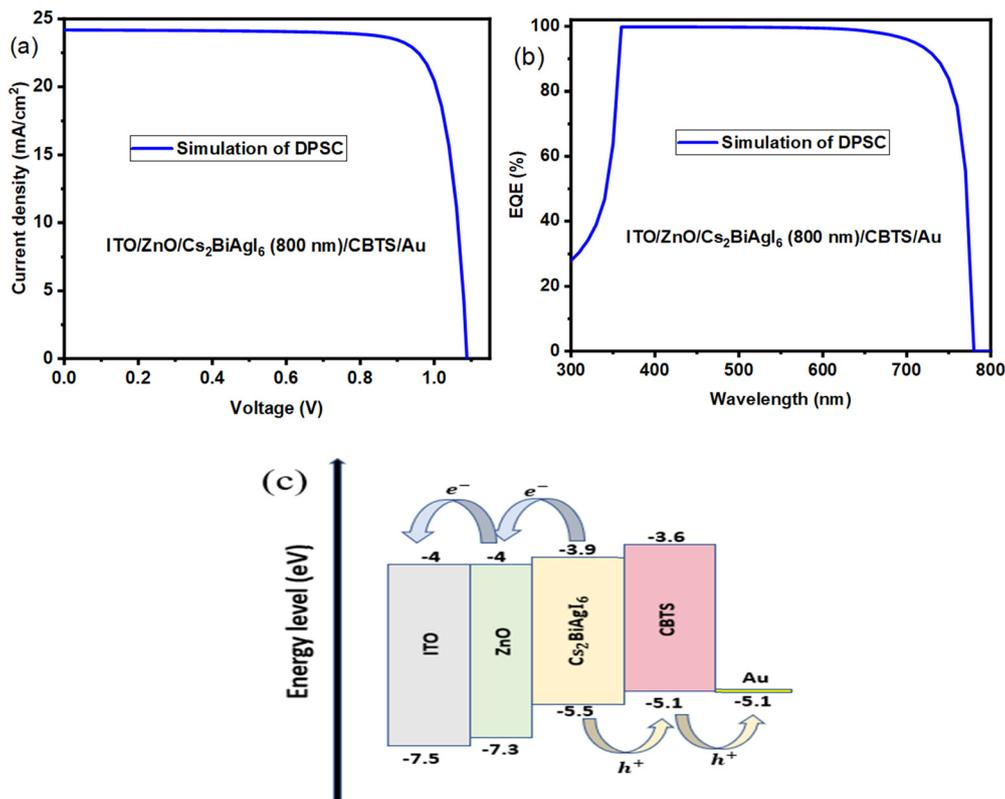
Fig. 2 Simulation results for the (a) current density–voltage ( $J$ – $V$ ) curve, (b) external quantum efficiency (EQE) curve, and (c) energy band alignment of the ITO/ZnO/Cs<sub>2</sub>BiAgI<sub>6</sub> (800 nm)/CBTS/Au device.<sup>47</sup>
