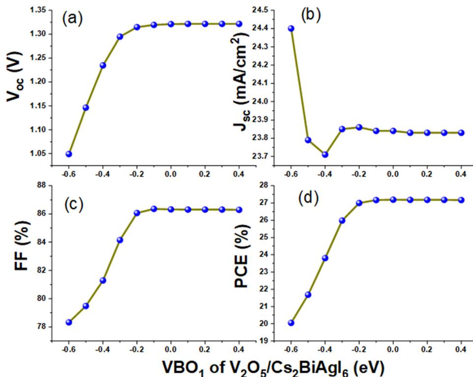
Fig. 10 (a)–(d) PV output parameters with the variation of VBO<sub>1</sub> of V<sub>2</sub>O<sub>5</sub>/Cs<sub>2</sub>BiAgI<sub>6</sub> between –0.6 eV and +0.4 eV.
