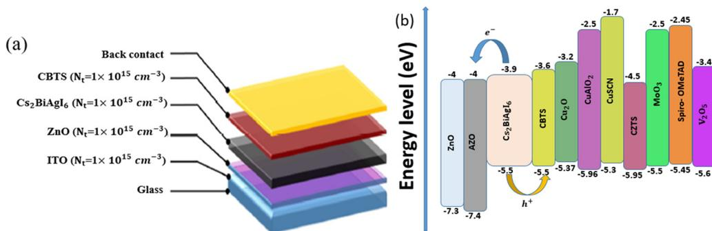
Fig. 1 (a) Device structure of the  $\text{Cs}_2\text{AgBiI}_6$ -DPSC. The defect densities of each layer ( $N_t$ ) are shown in the parentheses. (b) Energy band alignment of ETLs, HTLs, and the DPPVK layer.
