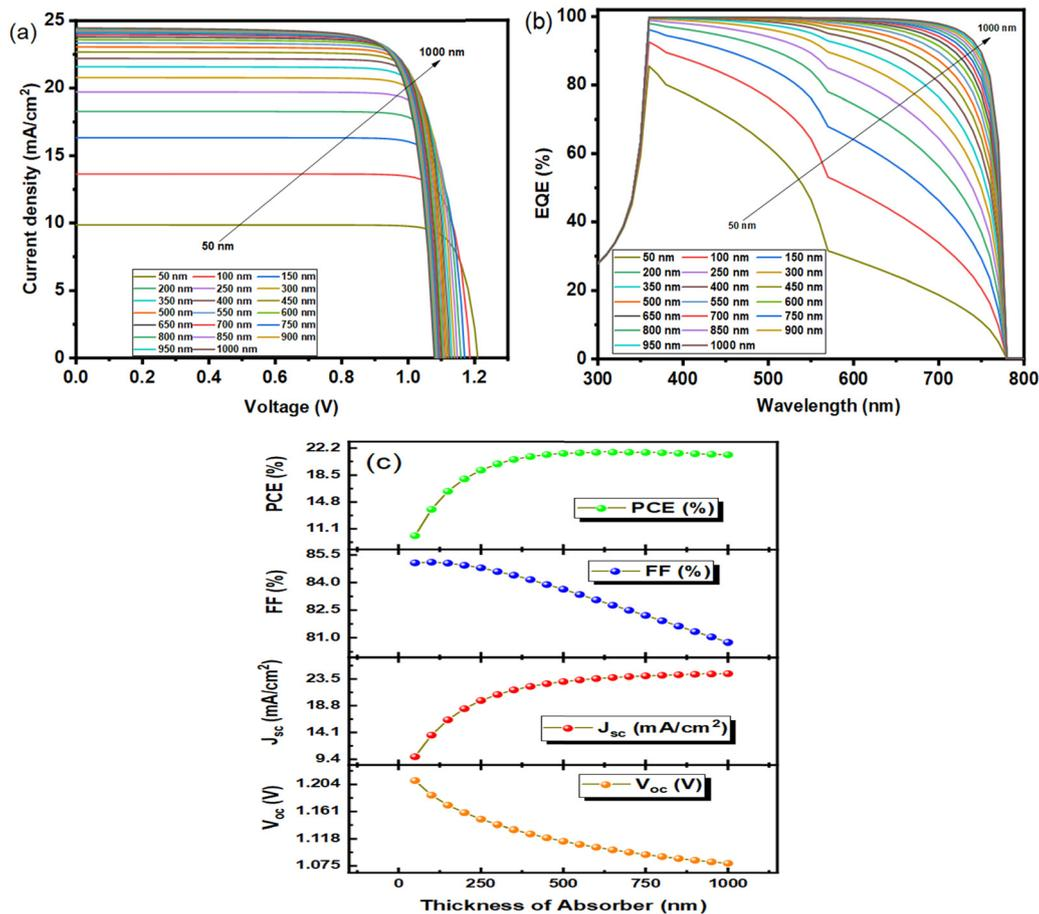
Fig. 6 (a)  $J$ - $V$  curve, (b) EQE curve, and (c) performance parameters for different double perovskite absorber layer thicknesses ranging from 50 to 1000 nm in 20 steps.
