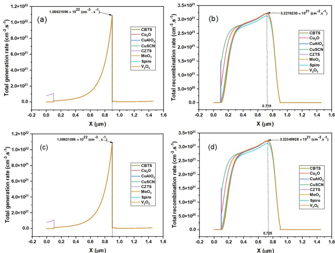
Fig. 5 Total generation and recombination rate of (a) and (b) ZnO/AZO and (c) and (d) ZnO ETLs.
