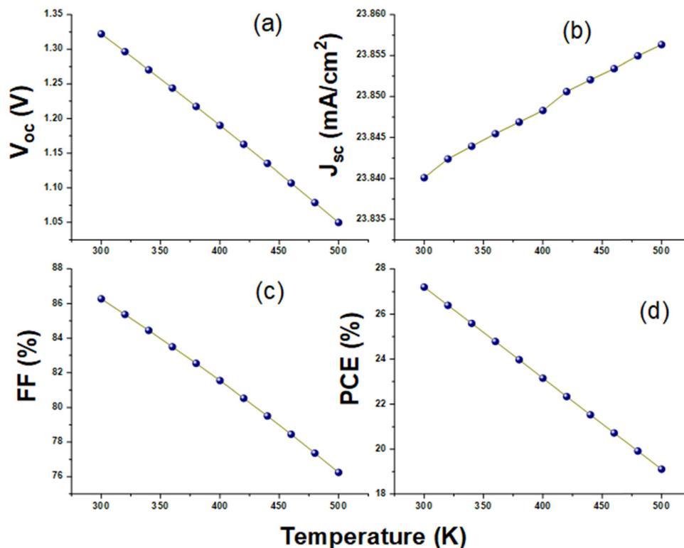
Fig. 16 PV output parameters: (a)  $V_{oc}$ , (b)  $J_{sc}$ , (c) FF, and (d) PCE for  $Cs_2BiAgI_6$ -DPSC against temperature.
