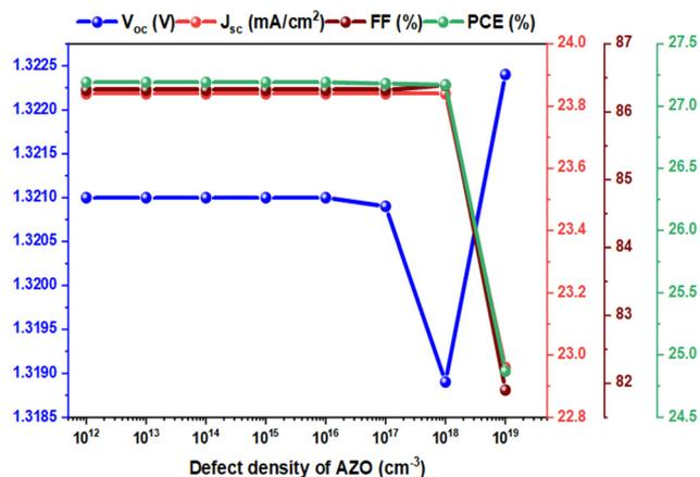
Fig. 11 PV output parameters for Cs<sub>2</sub>BiAgI<sub>6</sub>-DPSC against the defect density of AZO UTL.
