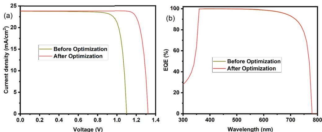
Fig. 17 Comparing the results of before and after optimization for ITO/ZnO/AZO/ $Cs_2BiAgI_6$  (650 nm)/ $V_2O_5$ /Se device: (a)  $J$ - $V$  curve and (b) EQE curve.
