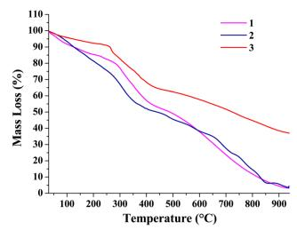
Fig. 3 TGA curves of [Zn(ahpa)(Cl)(H<sub>2</sub>O)] (1), [Zn(ahpa)(NO<sub>3</sub>)(H<sub>2</sub>O)] (2) and  $[Zn(ahpa)(H_2O)_2](ClO_4)$  (3) under an inert atmosphere of nitrogen gas at a heating rate of  $\sim 12$  °C min<sup>-1</sup>.
