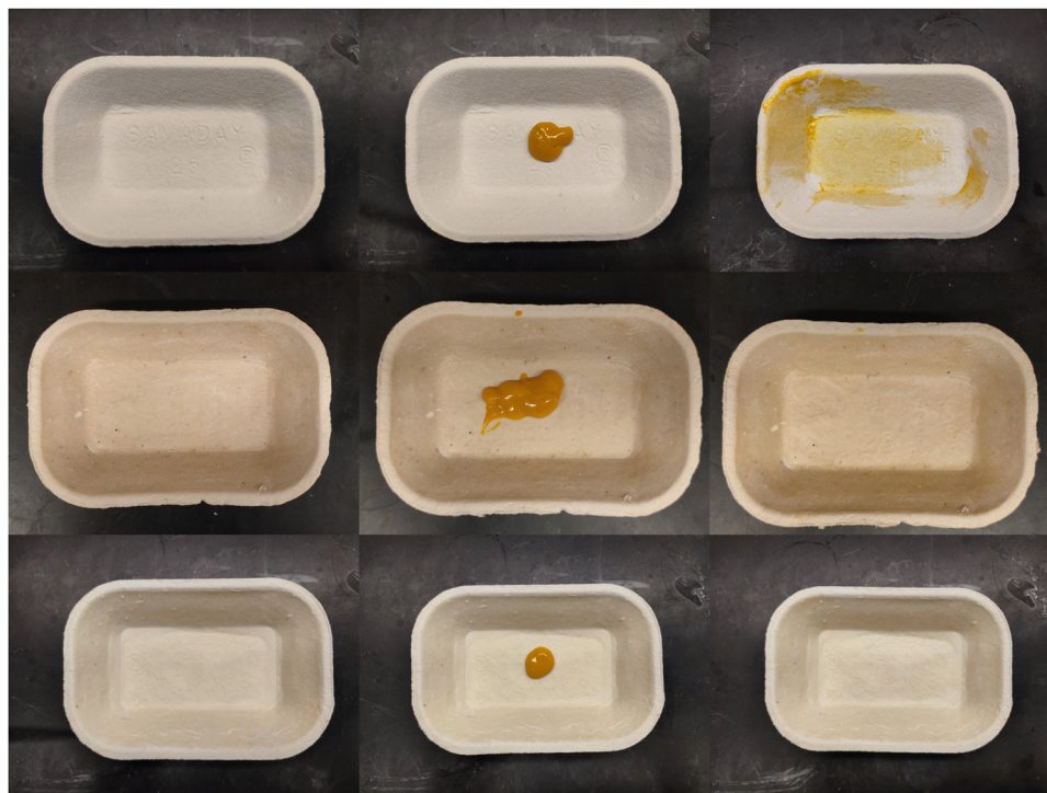
Fig. 4 Yellow mustard stain test. From top to bottom were uncoated MP trays, CNF/CMC coated MP trays, and formulated CNF coated trays. From left to right there were trays before testing, during testing, and after testing.
