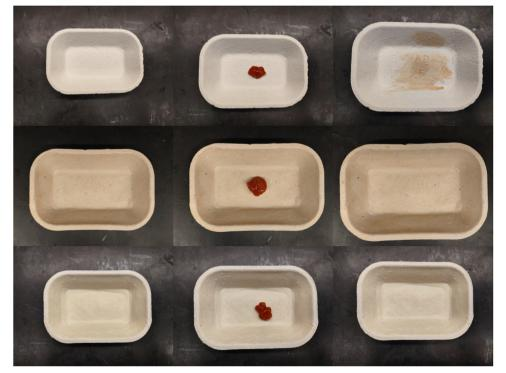
Fig. 3 Ketchup stain test. From top to bottom were uncoated MP trays, CNF/CMC coated MP trays, and formulated CNF coated trays. From left to right there were trays before testing, during testing, and after testing
