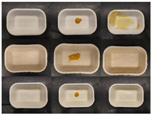
Fig. 4 Yellow mustard stain test. From top to bottom were uncoated MP trays, CNF/CMC coated MP trays, and formulated CNF coated trays. From left to right there were trays before testing, during testing, and after testing.
