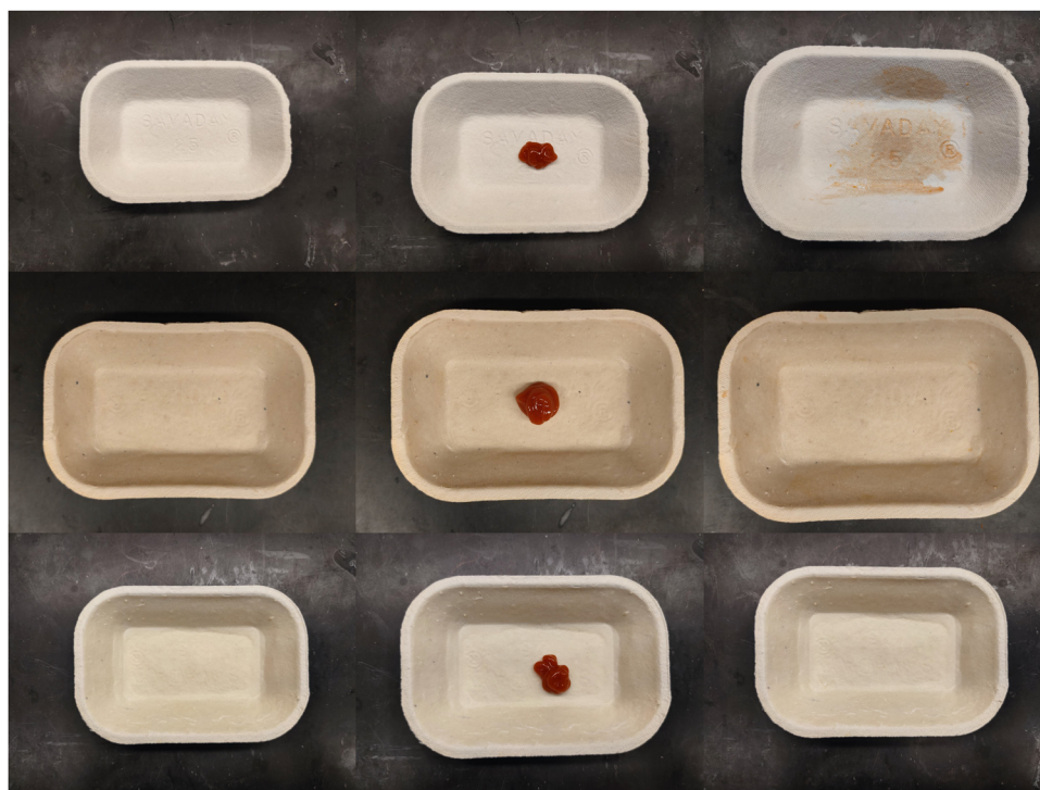
Fig. 3 Ketchup stain test. From top to bottom were uncoated MP trays, CNF/CMC coated MP trays, and formulated CNF coated trays. From left to right there were trays before testing, during testing, and after testing.
