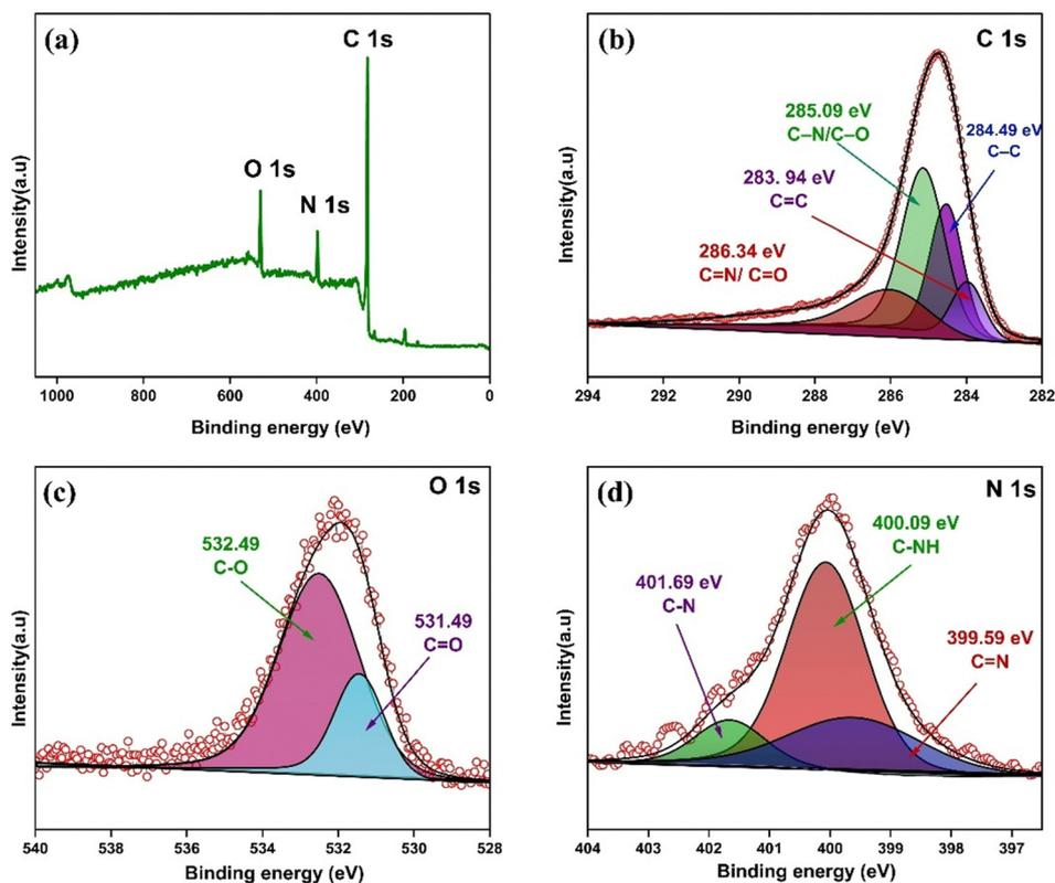
Fig. 2 Deconvoluted XPS spectra of UzMWCNT/PPy: (a) survey spectra, (b) C 1s, (c) O 1s, and (d) N 1s.
