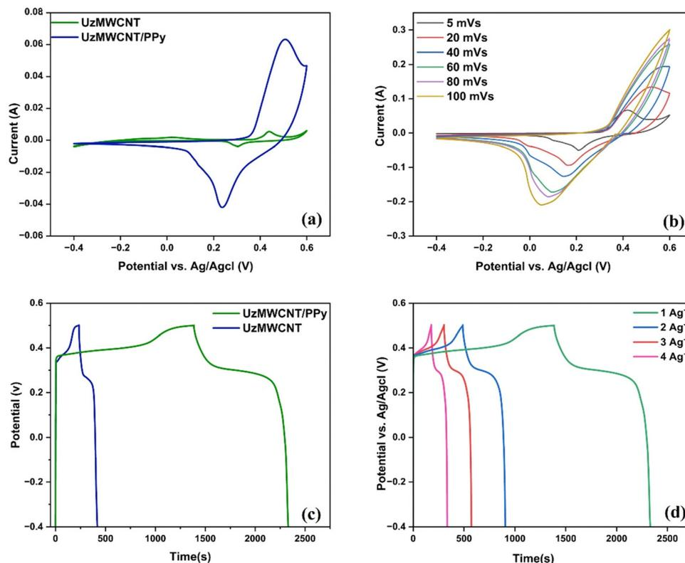
Fig. 6 (a) Cyclic voltammograms of UzMWCNT and UzMWCNT/PPy nanocomposites at a fixed scan rate of  $50 \text{ mV s}^{-1}$ ; (b) CV curves of the UzMWCNT/PPy nanocomposite electrode at varying scan rates; (c) GCD profiles of UzMWCNT and UzMWCNT/PPy nanocomposites; and (d) GCD curves of UzMWCNT/PPy nanocomposite electrodes at different current densities.
