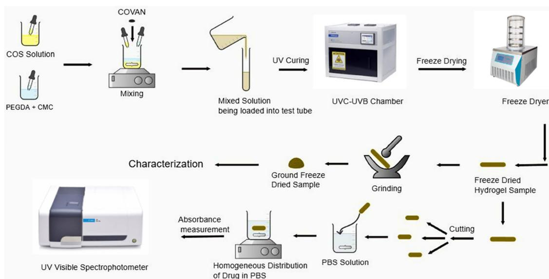
Fig. 1 The graphical methodology starting from hydrogel synthesis to characterization and application.
