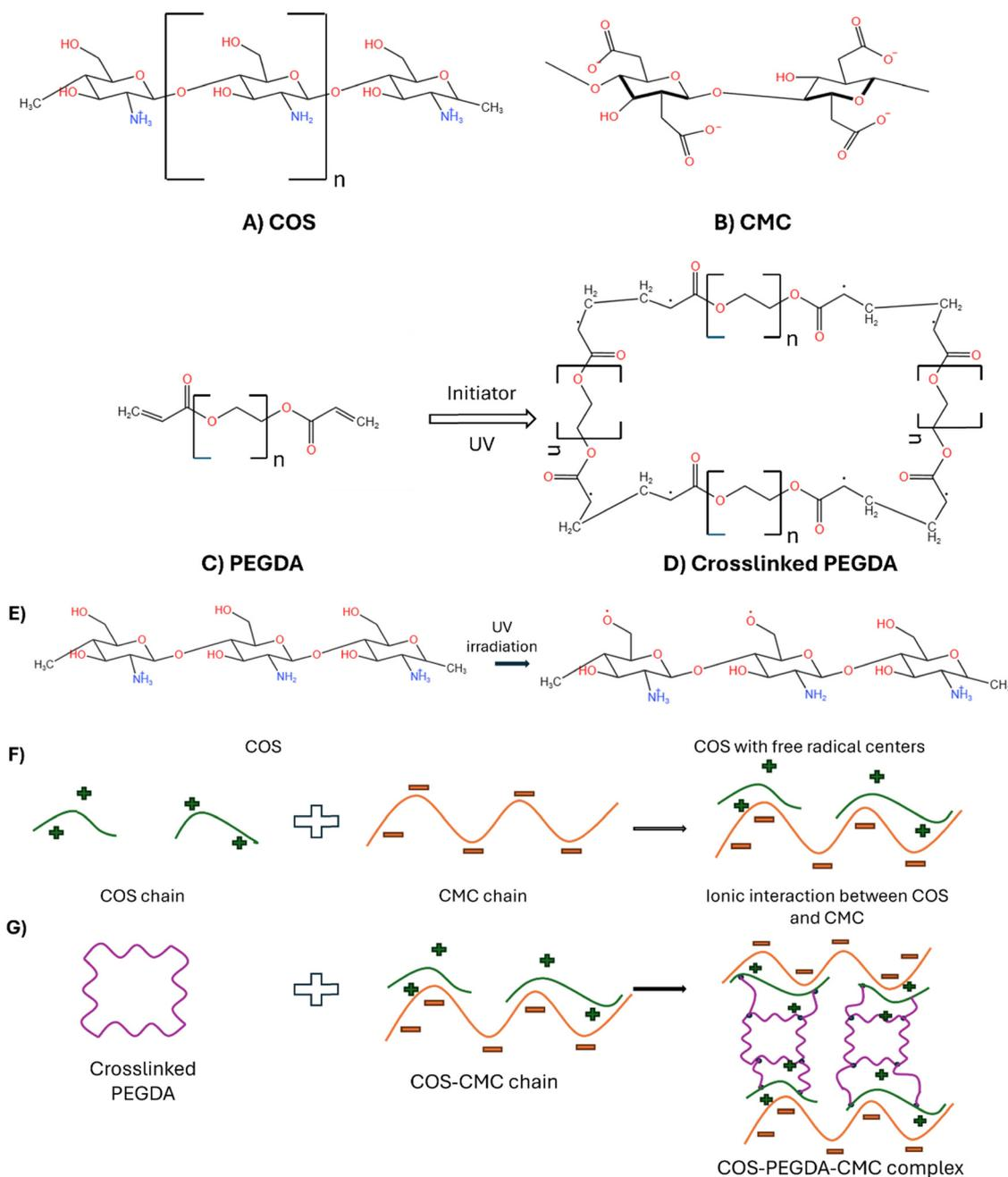
**Fig. 4** Chemical structure of (A) COS; (B) CMC; (C) PEGDA; (D) crosslinked PEGDA due to UV photocrosslinking; (E) free radical formation on the COS chain due to UV irradiation; (F) ionic interaction between COS and the CMC chain; and (G) interaction between crosslinked PEGDA and the COS–CMC complex to form a COS–PEGDA–CMC complex.
