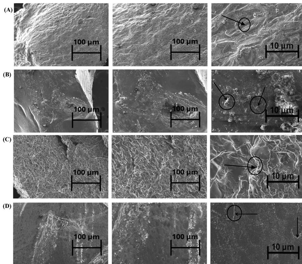
Fig. 3 Scanning electron microscope images of the surface morphology at 500 $\times$ , 1k $\times$  and 5k $\times$  of (A)  $N(\text{WD})$ ; (B)  $N(\text{D})$ ; (C)  $4^\circ(\text{WD})$  and (D)  $4^\circ(\text{D})$ . The black arrows and circles in  $4^\circ(\text{WD})$  and  $N(\text{WD})$  indicate the voids in the hydrogel surface. In contrast, the black arrows and circles in  $4^\circ(\text{D})$  and  $N(\text{D})$  indicate the loaded drug.
