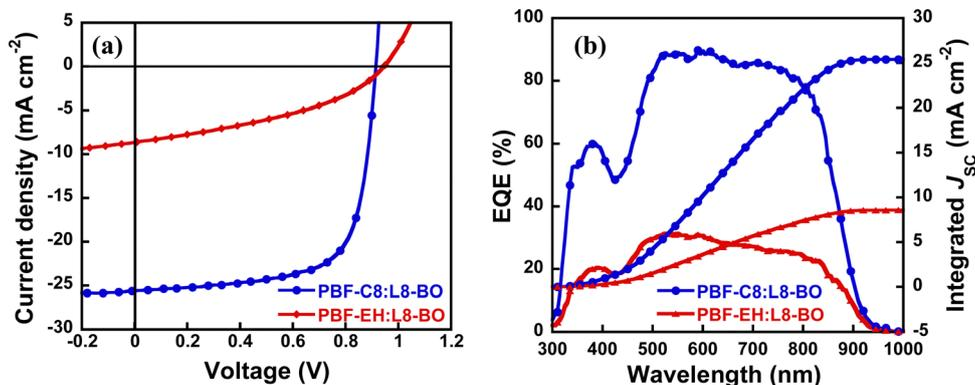
Fig. 5 (a)  $J$ - $V$  characteristics and (b) EQE curves of the optimal devices.
