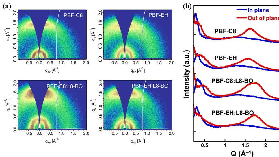
Fig. 9 2D GIWAXS patterns (a) and line-cut profiles in the IP and OOP directions (b) for PBF-C8 and PBF-EH neat and blended films.
