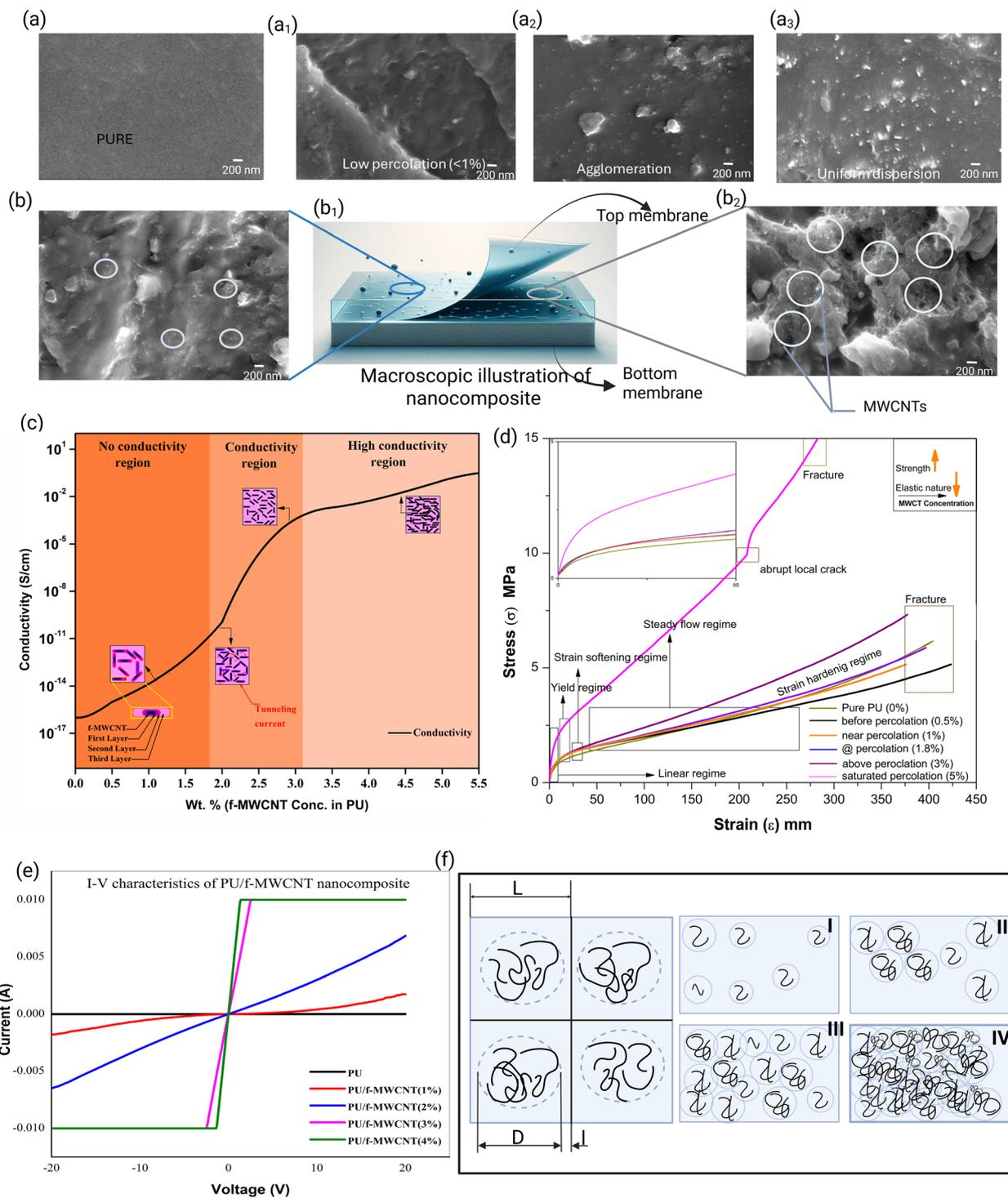
Fig. 4 (a)–(a<sub>3</sub>) SEM micrographs of the surface of nanocomposites at different filler loading conditions. (b)–(b<sub>2</sub>) SEM micrographs of the surface after removal of the top membrane. (c) Electrical percolation curve of PU/f-MWCNTs nanocomposites. (d) Tensile study of nanocomposites. (e) *I*–*V* curves of PU/f-MWCNTs nanocomposites. (f) Illustration of the interface between the filler and the polymer for electrical conduction.
