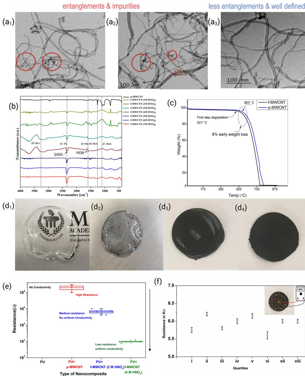
Fig. 3 TEM images of p-MWCNTs (a<sub>1</sub> and a<sub>2</sub>) and f-MWCNTs (a<sub>3</sub>). (b) FTIR spectra of acid functionalization. (c) TGA curves of MWCNTs. (d<sub>1</sub>)–(d<sub>4</sub>) PU and its nanocomposites. (e) Resistance change for different filler loadings of nanocomposites. (f) Uniform electrical properties of the nanocomposite.
