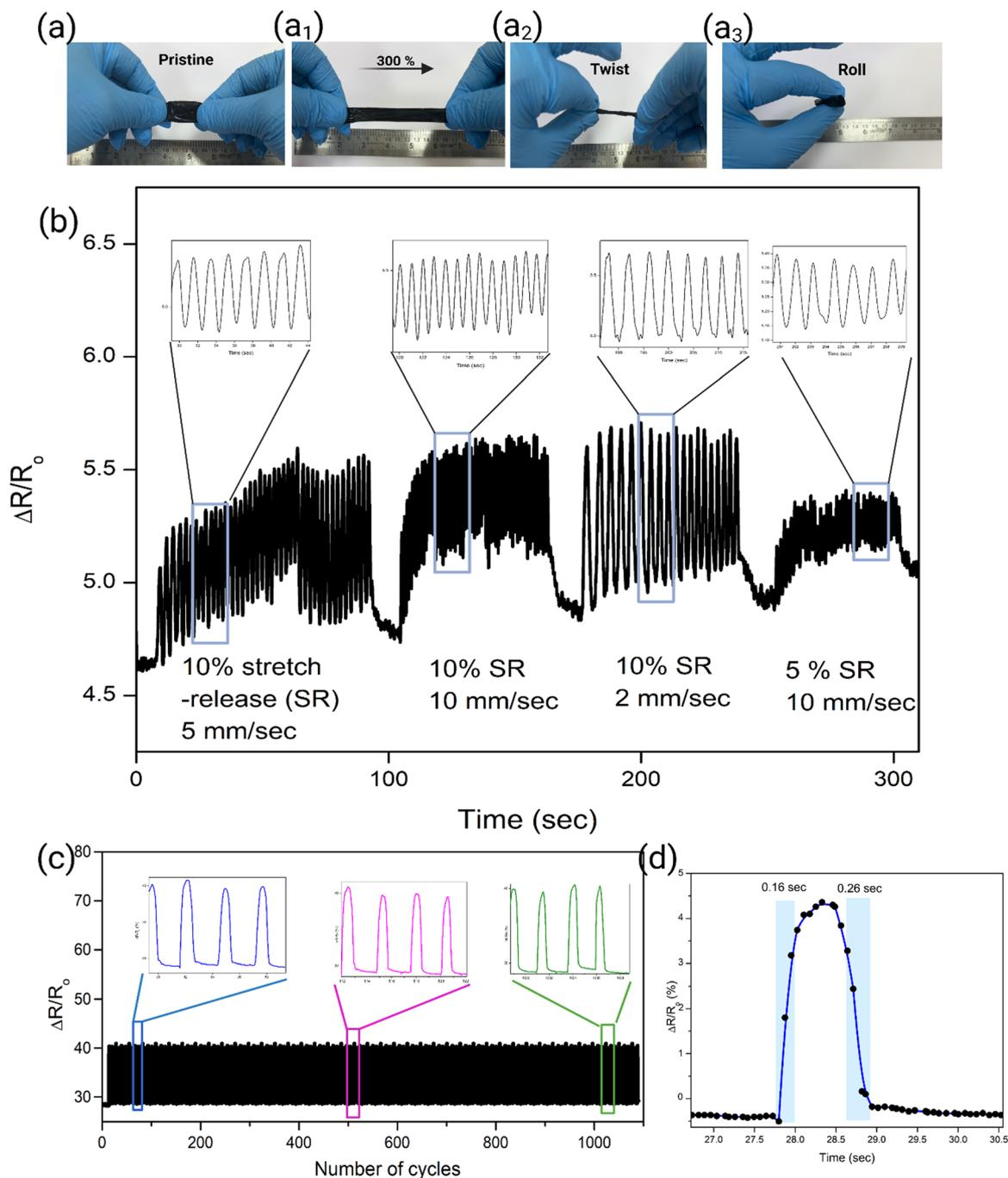
Fig. 6 (a)–(a<sub>3</sub>) Sensors flexible properties. (b) Real-time data of sensor stretch–release performance. (c) Sensitivity of the sensor over prolonged time. (d) Response time of the sensor.
