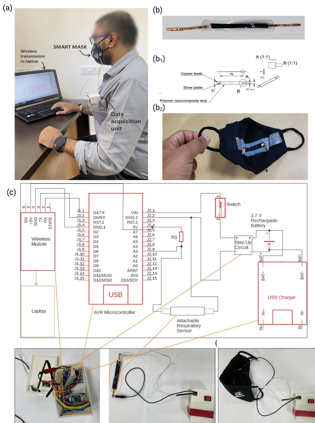
Fig. 5 (a) Sensor enabled mask wearing for the test. (b and b<sub>1</sub>) Sensor and its CAD model and (b<sub>2</sub>) sensor-integrated mask. (c) Circuit diagram for acquiring signals for fabrication of the DAU.
