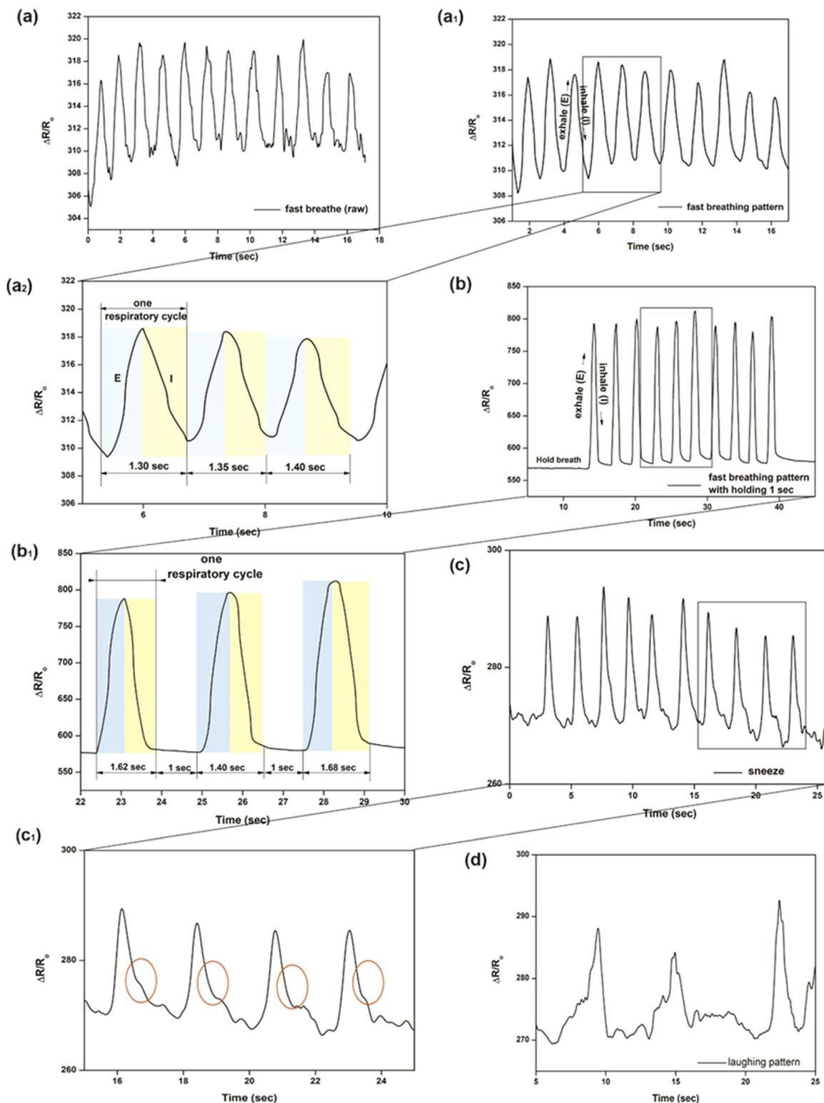
Fig. 8 (a) Raw signal of fast breathing, (a<sub>1</sub>) processed signal of fast breathing with (a<sub>2</sub>) the enlarged view. (b) Fast breathing with a hold of 1 s and its (b<sub>1</sub>) enlarged view. (c) Sneezing pattern with its (c<sub>1</sub>) enlarged view. (d) Laughing pattern.
