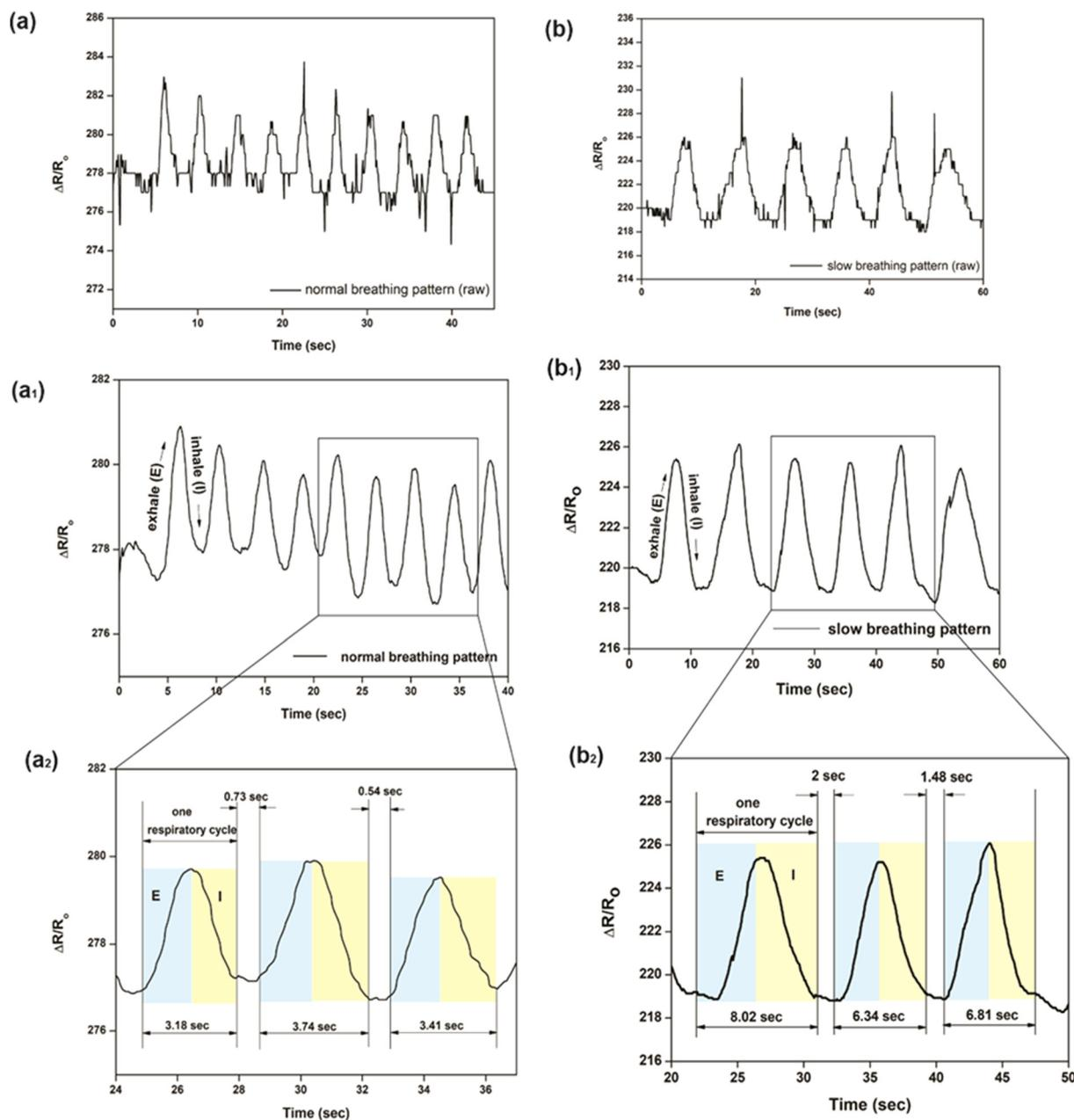
Fig. 7 (a) Raw signal of the normal breathing pattern with its (a<sub>1</sub>) processed signal and (a<sub>2</sub>) enlarged view with breathing parameters. (b) Raw signal of slow breathing with its (b<sub>1</sub>) processed signals, and enlarged (b<sub>2</sub>) view of the same pattern with breathing parameters.
