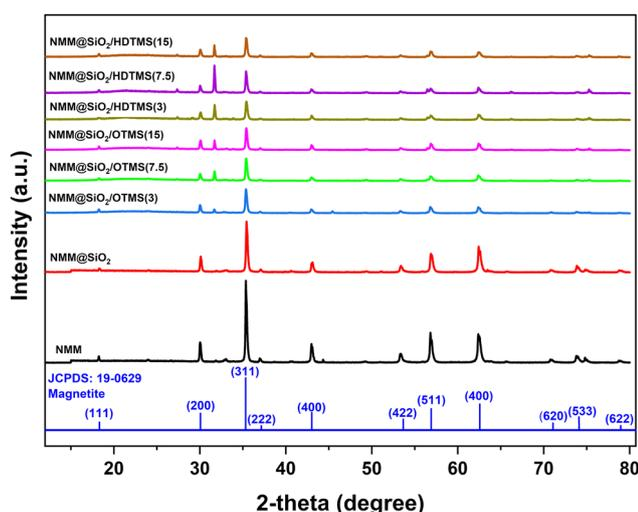
Fig. 3 XRD patterns of NMM@SiO<sub>2</sub>/alkylsilane materials.
