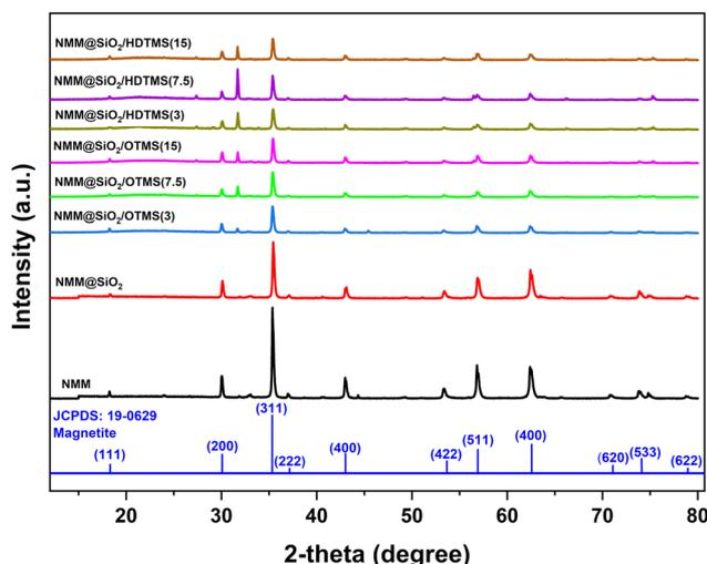
Fig. 3 XRD patterns of NMM@SiO<sub>2</sub>/alkylsilane materials.
