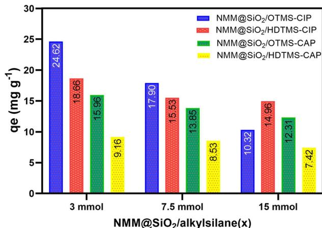
Fig. 5 Comparison of modified NMM@SiO<sub>2</sub>/OTMS and NMM@SiO<sub>2</sub>/HDTMS [ $C_0 = 100 \text{ mg L}^{-1}$ ,  $m = 20 \text{ mg}$ ,  $V = 20 \text{ mL}$ , time = 60 min (CIP), 90 min (CAP), pH = 6 (CIP and CAP), rotary speed = 250 rpm,  $T = 25 \text{ }^\circ\text{C}$ ].
