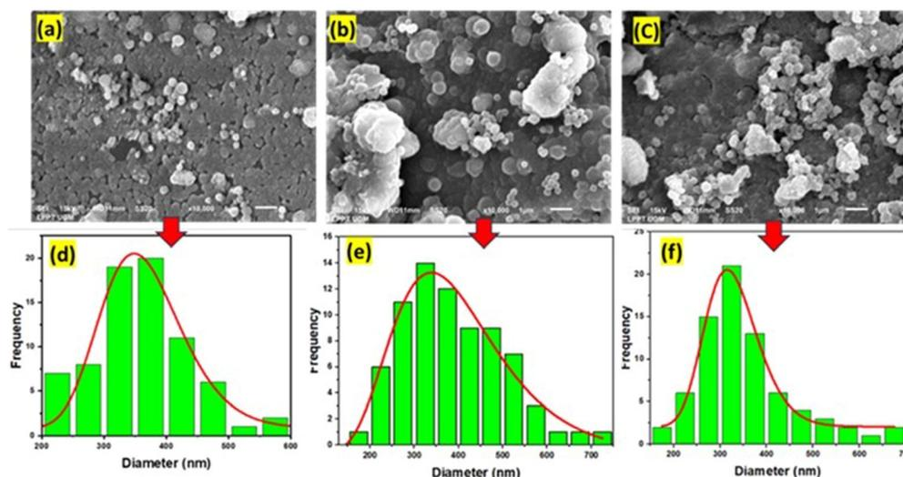
Fig. 6 SEM images of (a) NMM@SiO<sub>2</sub>/OTMS(3), (b) NMM@SiO<sub>2</sub>/OTMS(7.5), and (c) NMM@SiO<sub>2</sub>/OTMS(15), and particle size of (d) NMM@SiO<sub>2</sub>/OTMS(3), (e) NMM@SiO<sub>2</sub>/OTMS(7.5), and (f) NMM@SiO<sub>2</sub>/OTMS(15).
