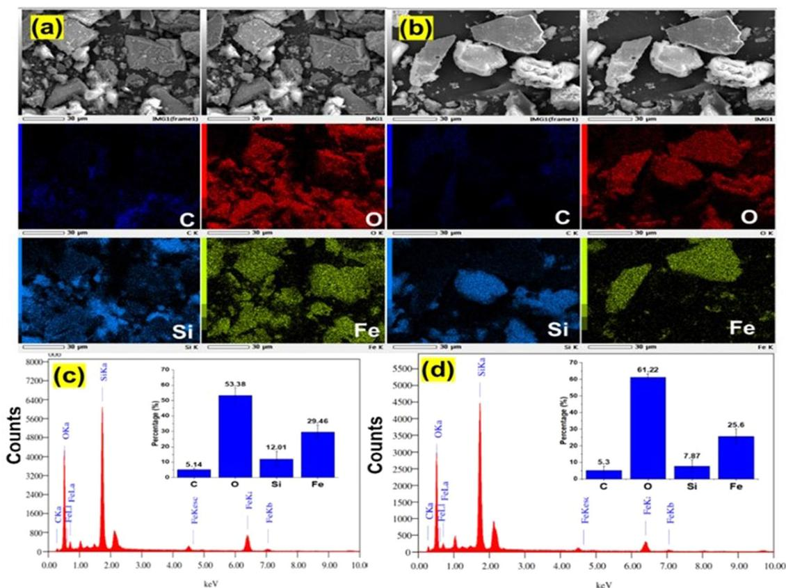
Fig. 7 SEM mapping of (a) NMM@SiO<sub>2</sub>/OTMS(3), (b) NMM@SiO<sub>2</sub>/HDTMS(3), and EDX spectra of (c) NMM@SiO<sub>2</sub>/OTMS(3), (d) NMM@SiO<sub>2</sub>/HDTMS(3).
