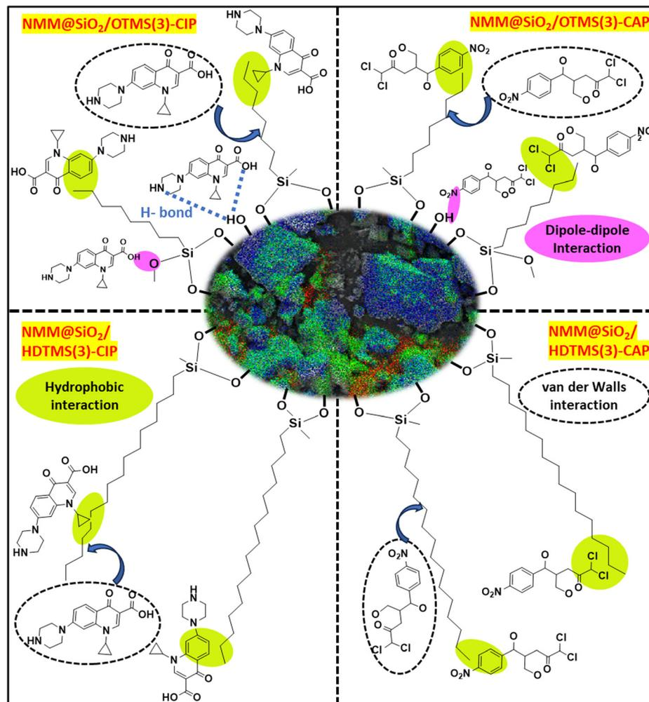
Fig. 14 Mechanism model of interaction between NMM@SiO<sub>2</sub>/OTMS and NMM@SiO<sub>2</sub>/HDTMS for CIP and CAP.
