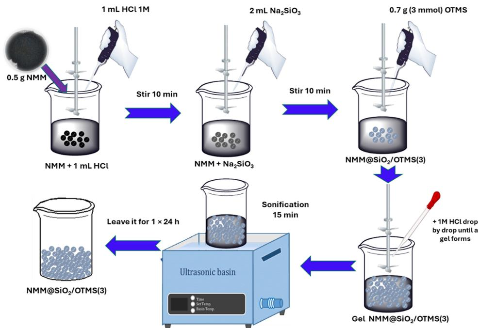
Fig. 1 NMM@SiO<sub>2</sub>/OTMS(3) synthesis pathway.
