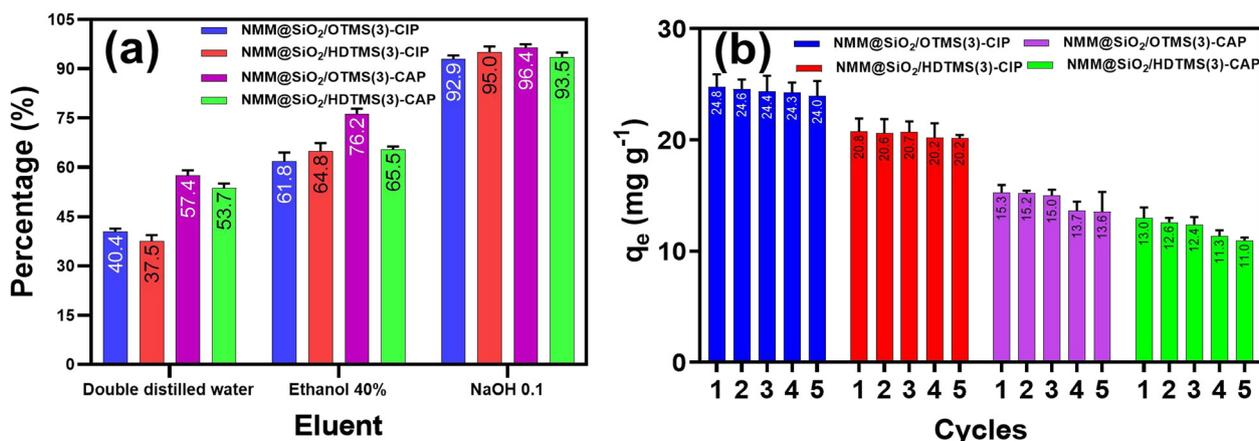
Fig. 13 (a) Desorbed antibiotic percentage from adsorbent with different eluents and (b) reusability of CIP and CAP adsorption in five cycles. [Conditions: adsorbent = NMM@SiO<sub>2</sub>/OTMS(3) and NMM@SiO<sub>2</sub>/HDTMS(3), time = 90 min (CAP), 60 min (CIP),  $C_0 = 100$  mg L<sup>-1</sup>, pH = 6,  $m = 20$  mg,  $V = 20$  mL, rotary speed = 250 rpm,  $T = 25$  °C].
