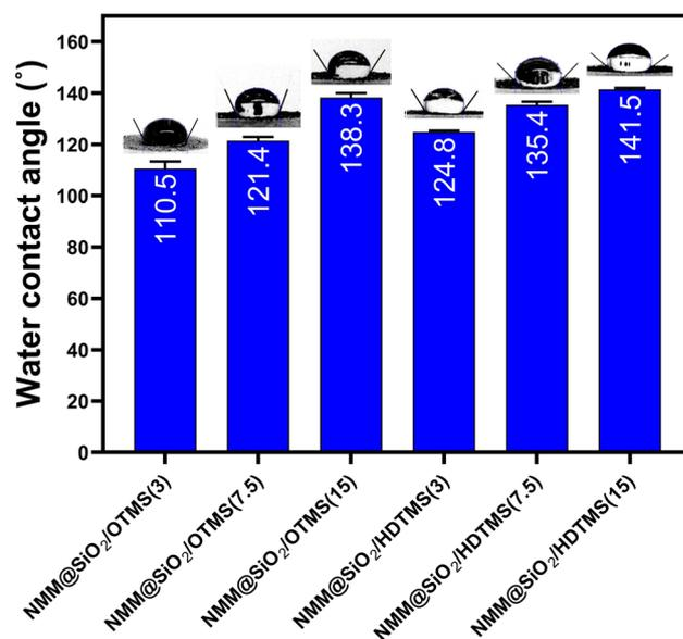
Fig. 4 Water contact angle of materials adsorbent.
