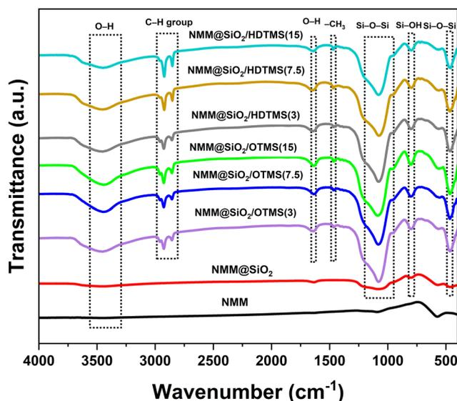
Fig. 2 FTIR spectra of NMM@SiO<sub>2</sub>/alkylsilane materials.
